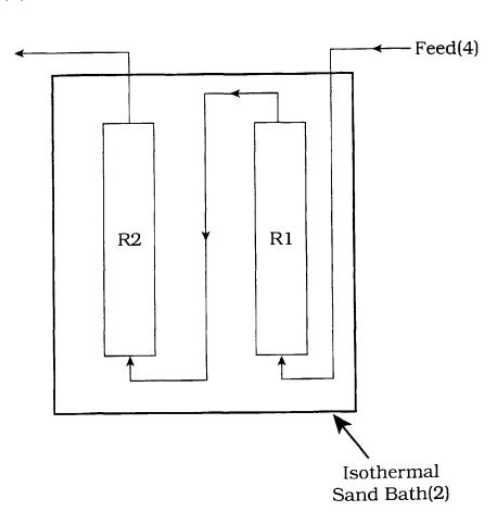
(57) Abstract: A process for the production of a winter diesel fuel from wax containing hydrocarbons produced by the Fischer-Tropsch hydrocarbon synthesis process. A 300° F+Fischer-Tropsch fraction is upgraded first by hydroisomerization followed by catalytic dewaxing resulting in a diesel fuel suitable for use as a winter diesel fuel having excellent cold flow properties and reduced emissions.
