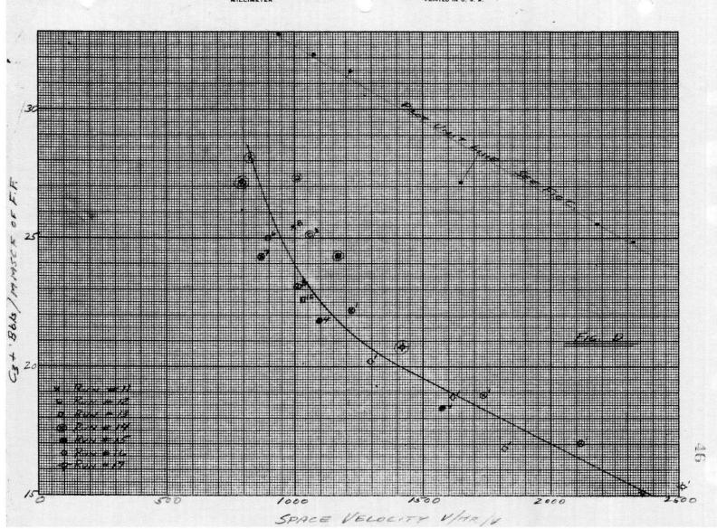
The pilot unit line on the other hand since it was based on the first few days operation of several different runs (see Table V p. 21 PR 37P) shows the effect predominantly of space velocity alone.
