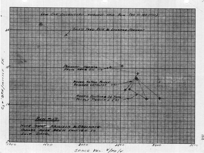
sharp drop which occurred during the later part of Runs 13 & 8. The drop in Run 13 may have been caused by a sharp change in mass spectrometer operations (could not be pinned down as such however) but that in Run #8 it is too consistent, in spite of maintaining constant operating conditions to be anything but catalyst deactivation.
