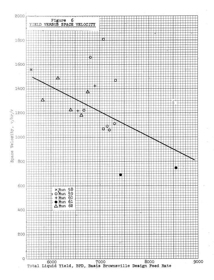
feed ratio. The unique factor of this run was the use of reduced catalyst which had been previously used in ammonia synthesis. This catalyst was essentially fully reduced when received at Montebello Research Laboratory.
