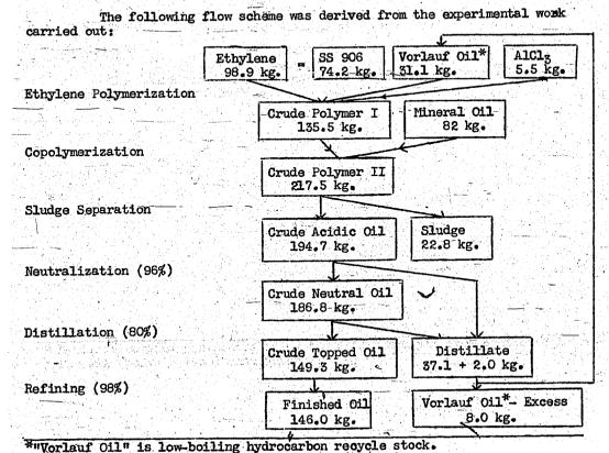
The final product was obtained from 74.2 kg. of SS Oil = 50.8% and 71.8 kg. of mineral oil = 49.2%, i.e., the two components were in this case taken in a ratio of almost 1:1. It is to be considered that, when ethylene is employed for copolymerization, instead of R-Oil\*\* being formed (to an extent of 7% on the basis of the finished SS-Oil), an asphaltic material is formed which must be disposed of by burning, for example, and does not yield any more lubricant.
