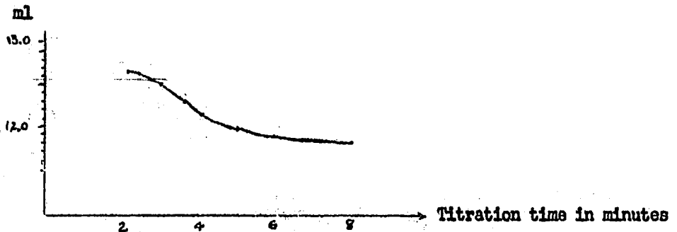
Curve 1: Dependence of Potassium Ferricyanide Consumption on Titration Time.
