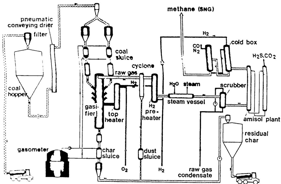
gasification pressure : up to 120 bar      coal throughput : up to 9,6 t/h dried brown coal
