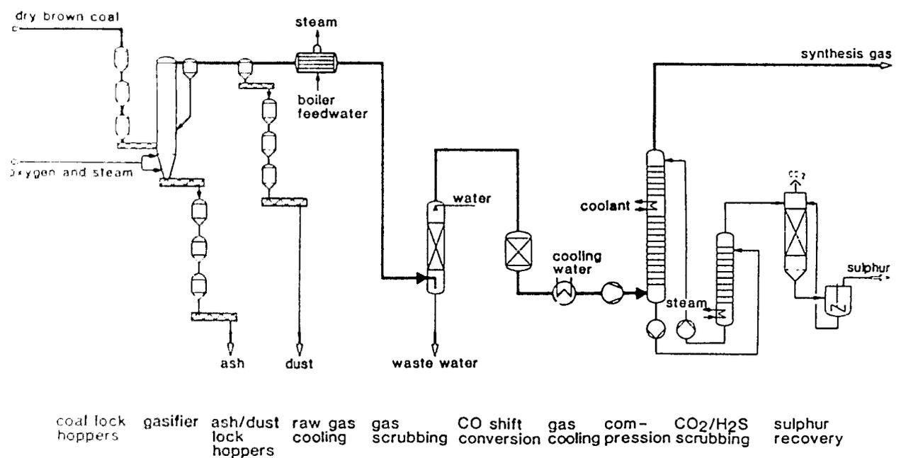
Fig. 5: Flow sheet of the HTW demonstration plant
