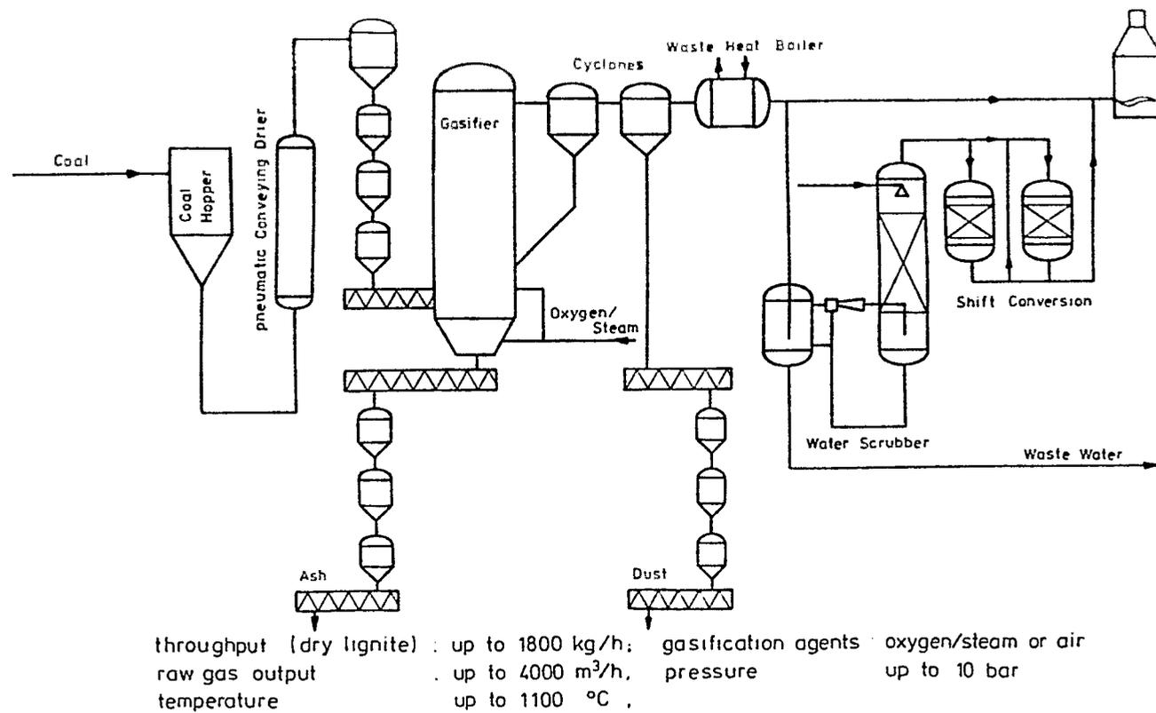
Fig. 1: Flow sheet HTW pilot plant
