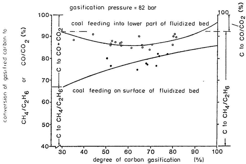
Fig. 7: Influence of coal feeding point on conversion of carbon into gases suitable for SNG
