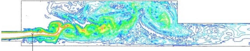
Figure 14. Scalar Field (Red: unburned gas, Blue: burned gas) With Swirl Correction
