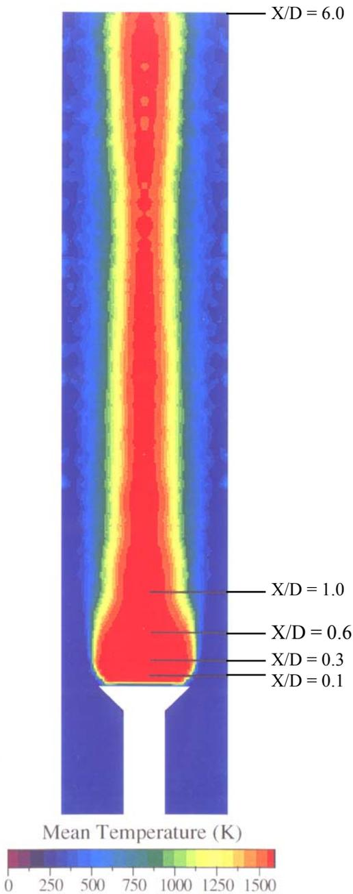
Figure 20. Predicted Mean Temperature in Lean Premixed Bluff-Body Combustor Using 5-step Chemistry and Monte Carlo PDF Method (Cannon, 1997)
