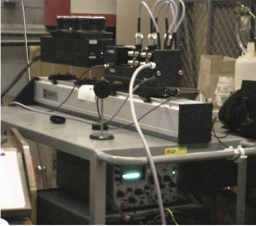
Figure 3.7: Laser Doppler Anemometer Setup.
