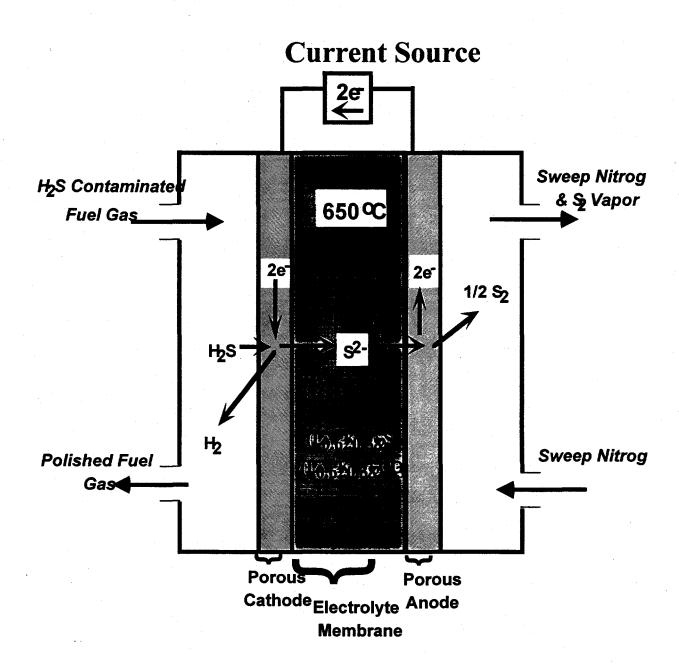
Figure 1. Single-Cell View of the Electrochemical Membrane Separator
