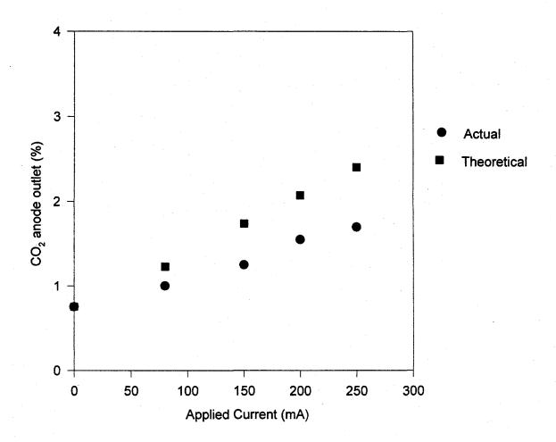
Figure 3. Run #34. Carbonate Transport - CO<sub>2</sub> Production vs. Applied Current
