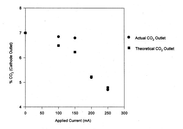
Figure 2. Run #34. Carbonate Transport - CO<sub>2</sub> Removal versus Applied Potential
