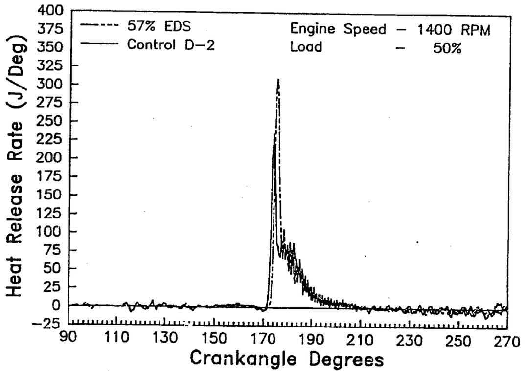
**FIGURE 6.43. HEAT RELEASE RATE FOR 57 PERCENT EDS AND CONTROL DF-2 FUELS AT 1400 RPM, 50 PERCENT LOAD, SIMULATED AIR-TO-AIR AFTERCOOLER AND HIGH PRESSURE FUEL INJECTION SYSTEM**
