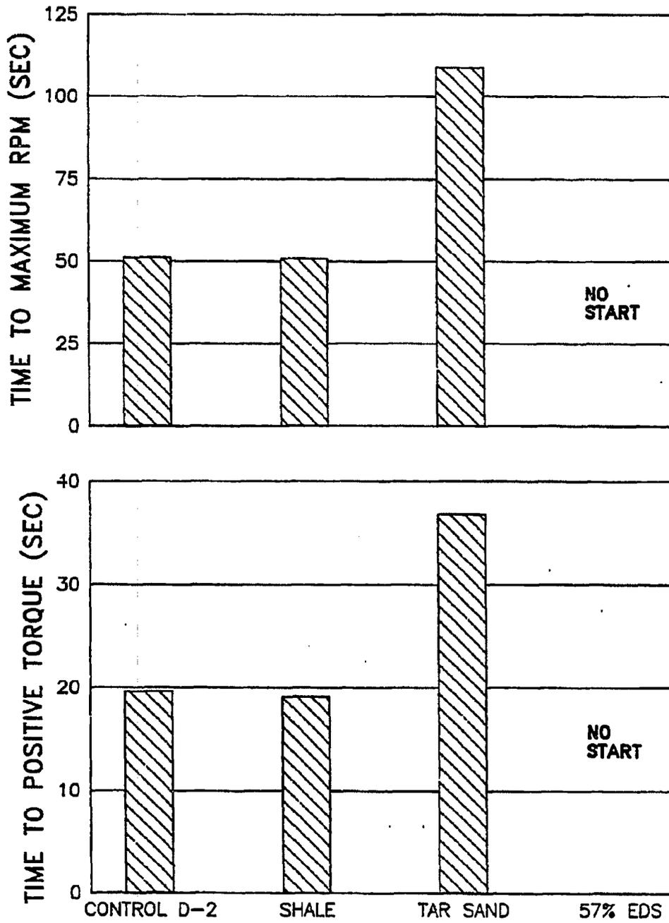
FIGURE 6.19. COLD START DATA AT -20° C
