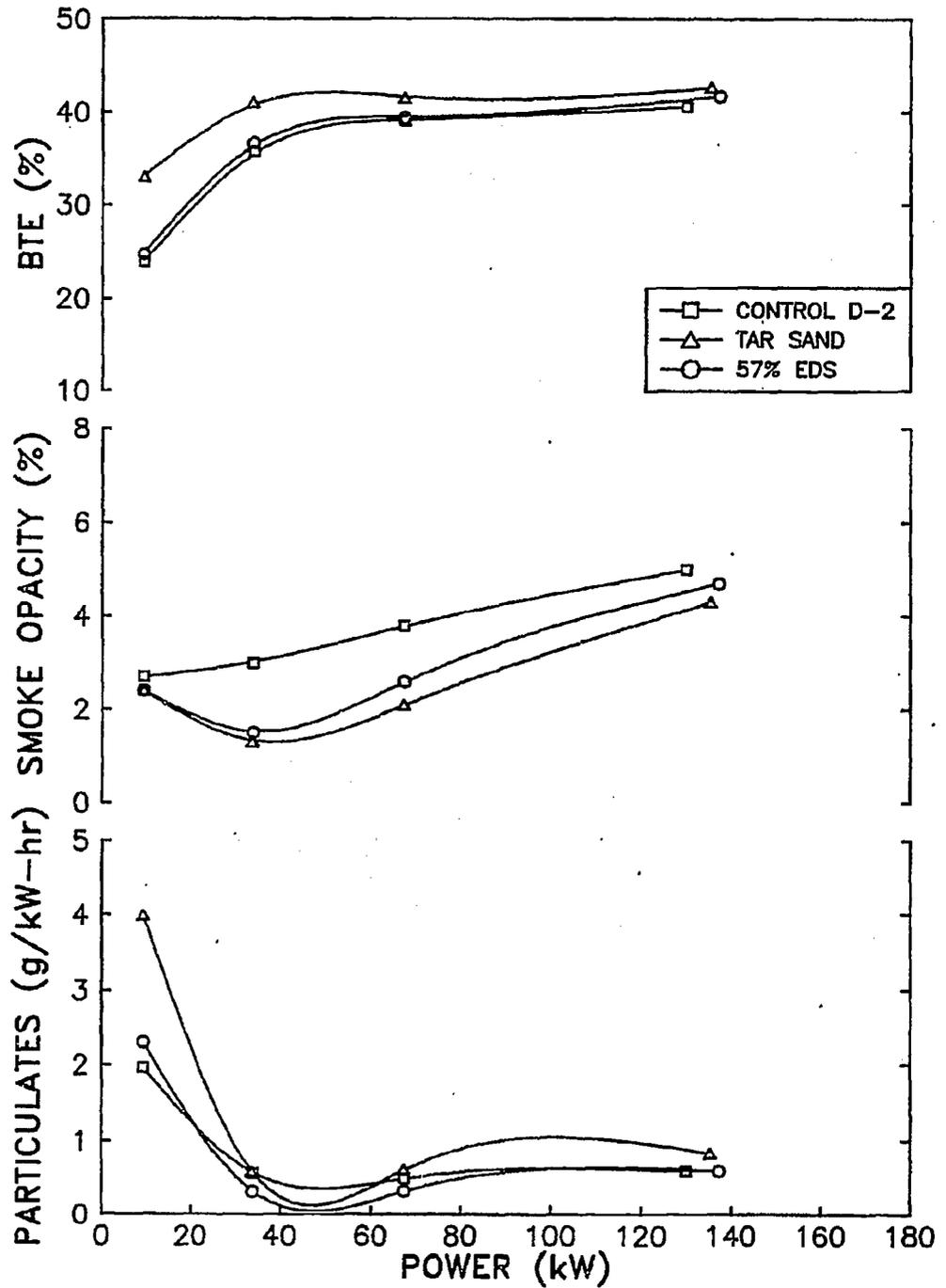
FIGURE 6.38. PERFORMANCE RESULTS AT 1400 RPM,
