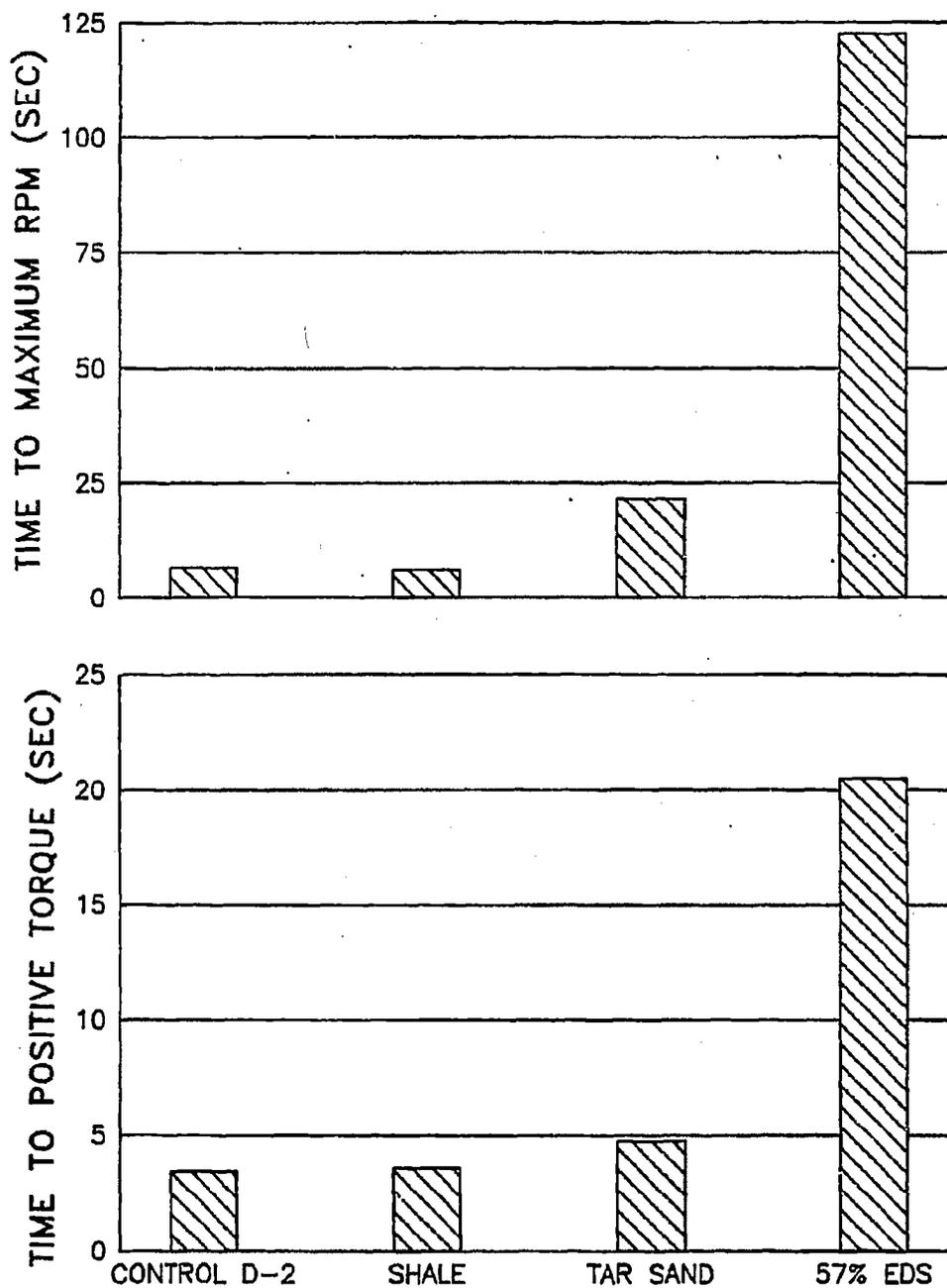
FIGURE 6.18. COLD START DATA AT 0°C
