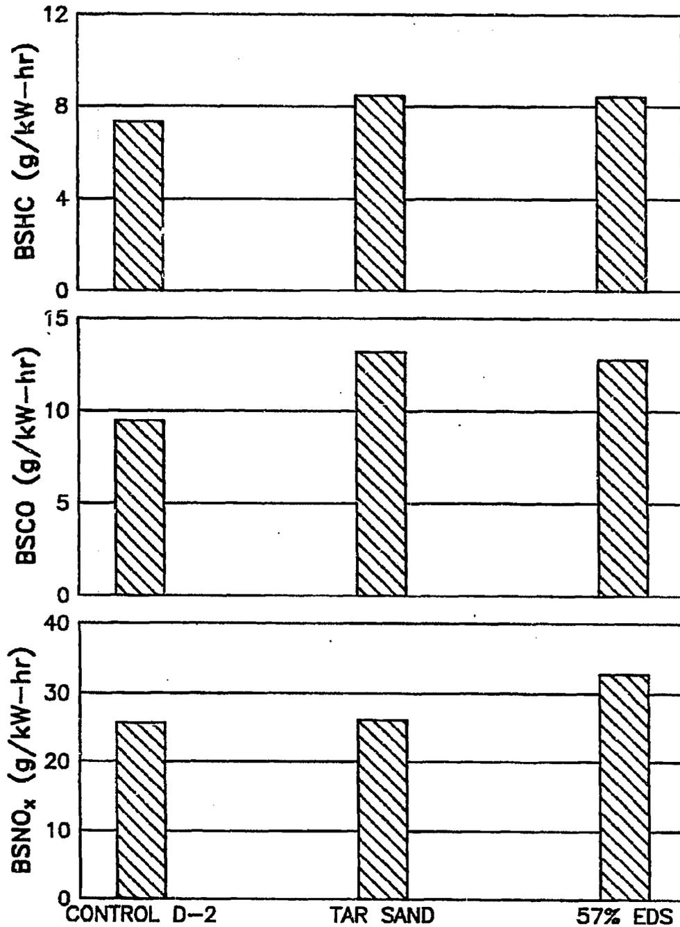
FIGURE 6.33. BRAKE SPECIFIC EMISSIONS AT IDLE, PHASE II SIMULATED AIR-TO-AIR AFTERCOOLER
