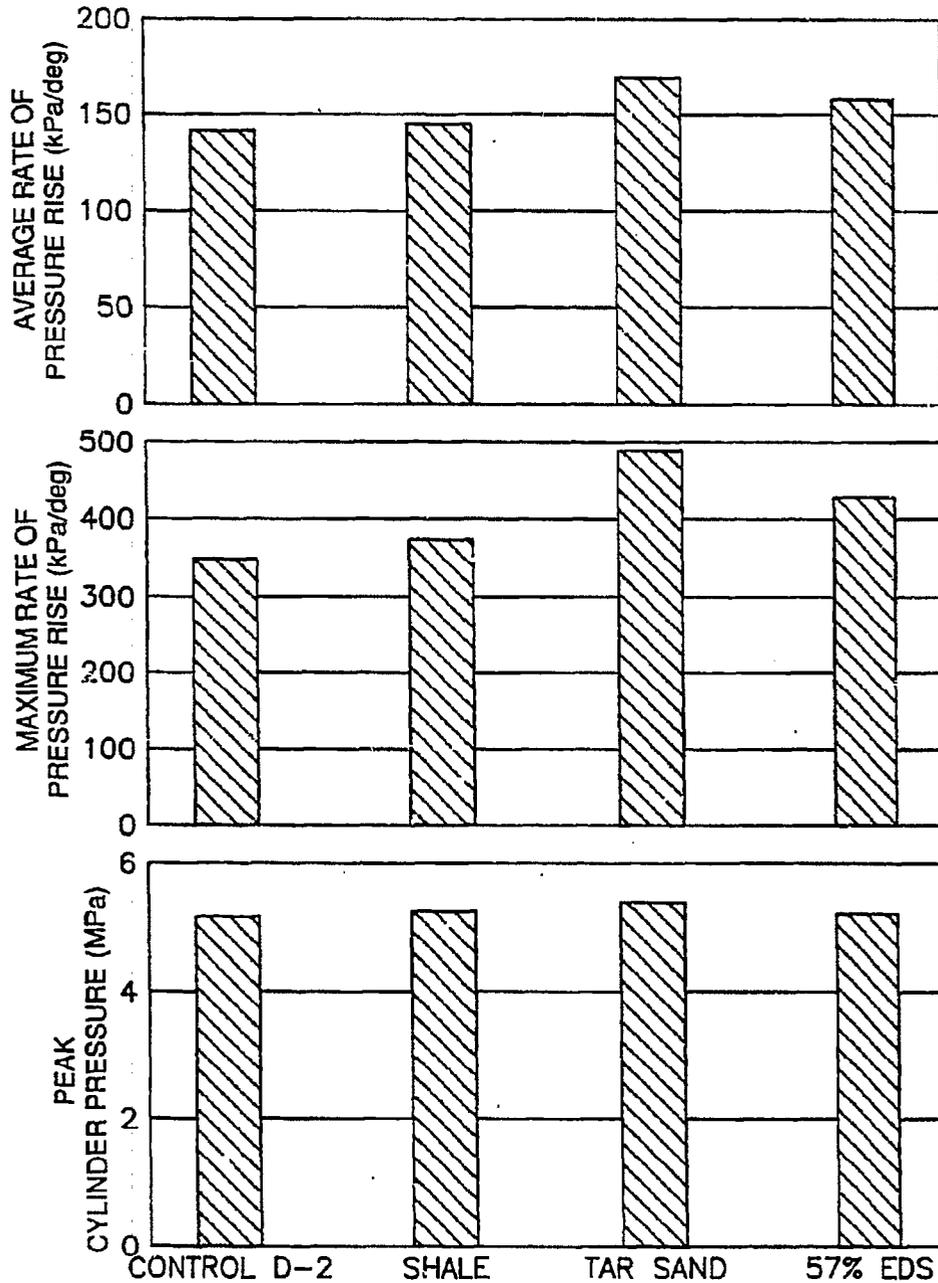
FIGURE 6.13. PEAK CYLINDER PRESSURES AND RATES OF PRESSURE RISE FOR EACH FUEL AT IDLE
