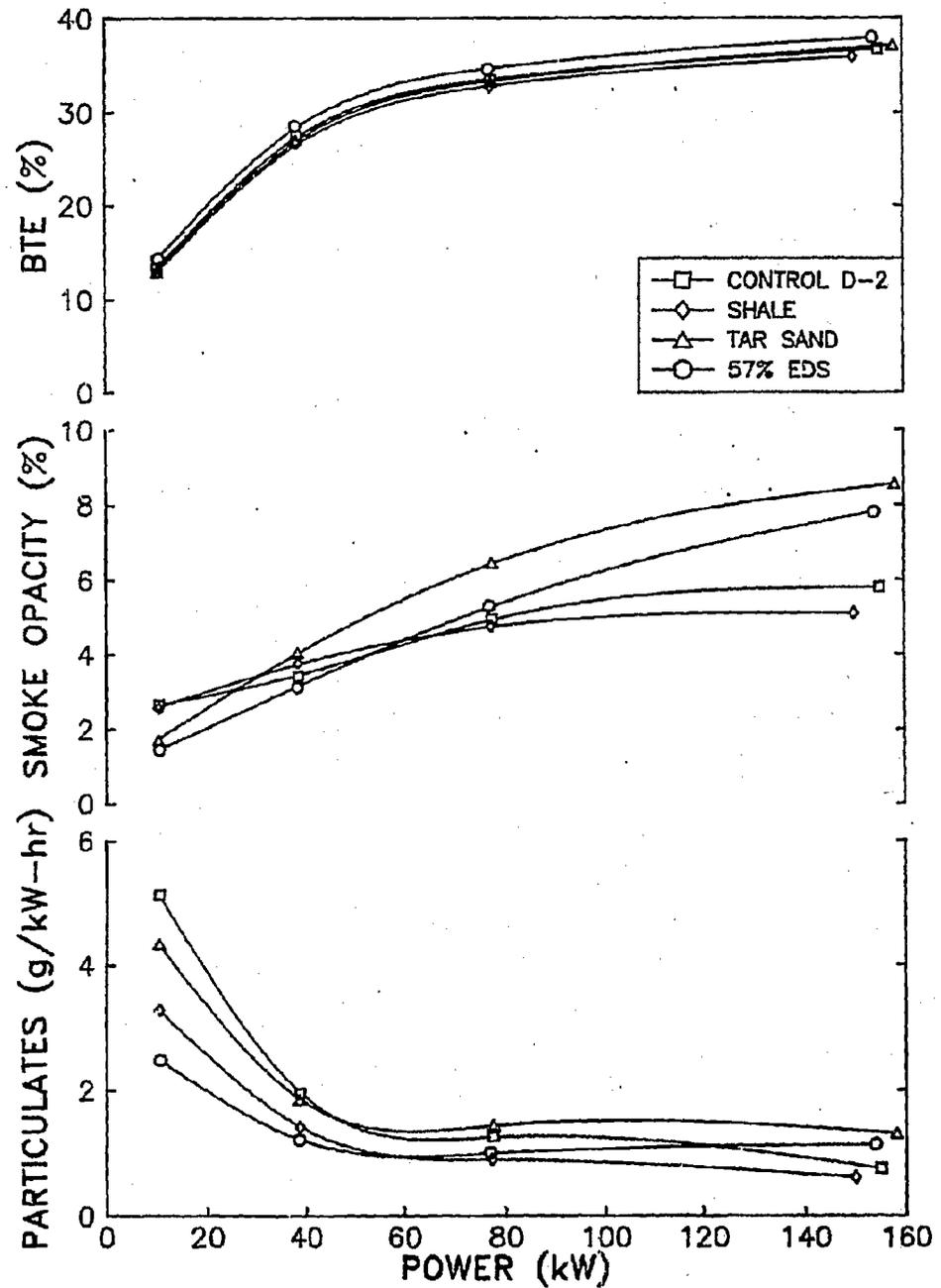
FIGURE 6.1. PERFORMANCE RESULTS AT 2200 RPM
