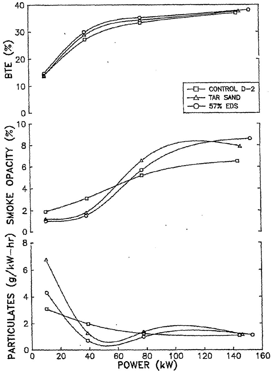
FIGURE 6.28. PERFORMANCE RESULTS AT 2200 RPM, PHASE II SIMULATED AIR-TO-AIR AFTERCOOLER
