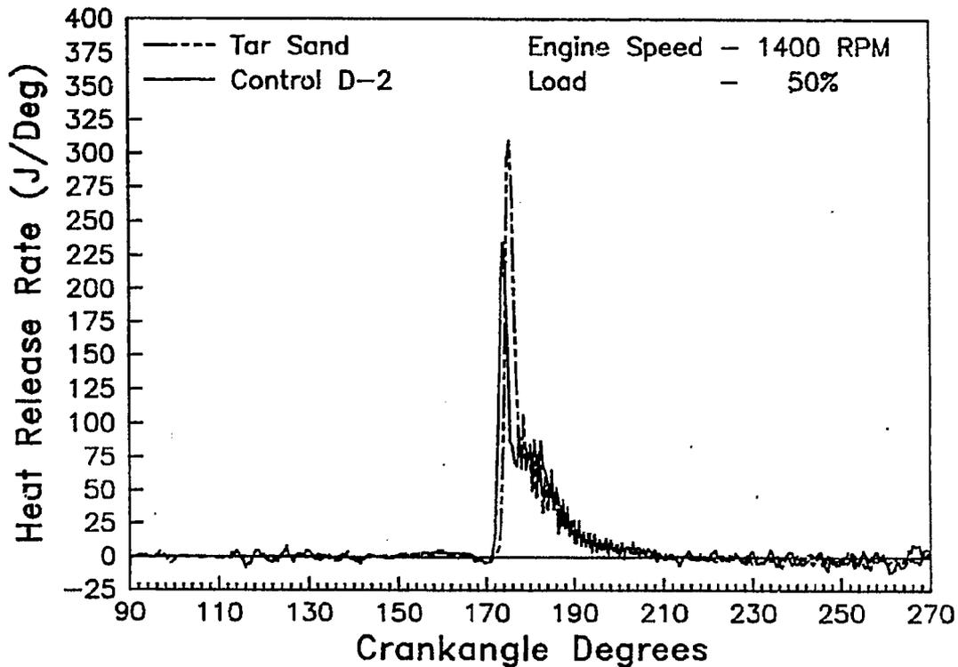
**FIGURE 6.42. HEAT RELEASE RATE FOR
