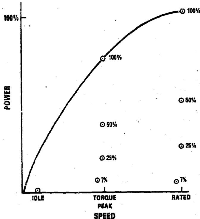
**FIGURE 5.6. DATA POINTS USED FOR PERFORMANCE, COMBUSTION, AND EMISSIONS ANALYSES**
