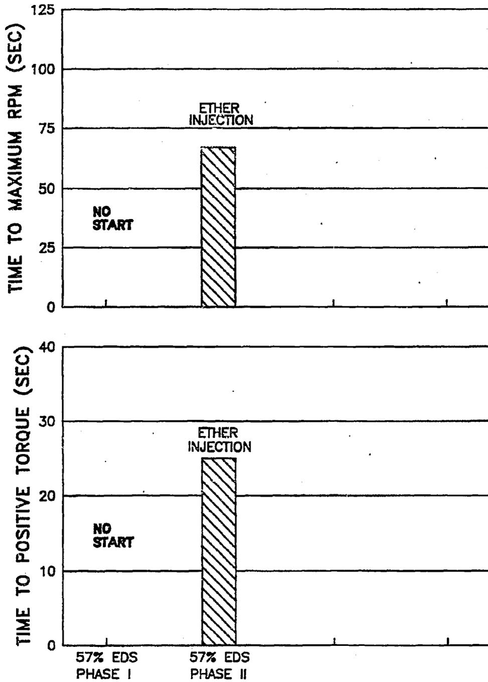
**FIGURE 6.45. COLD START DATA AT -20°C,
