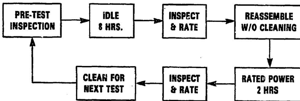
**FIGURE 5.7. SCHEMATIC OF THE IDLE DEPOSIT TEST SEQUENCE**
