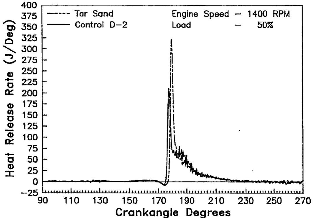
**FIGURE 6.34. HEAT RELEASE RATE FOR TAR SAND AND CONTROL D-2 FUELS AT 1400 RPM, 50 PERCENT LOAD, SIMULATED AIR-TO-AIR AFTERCOOLER**
