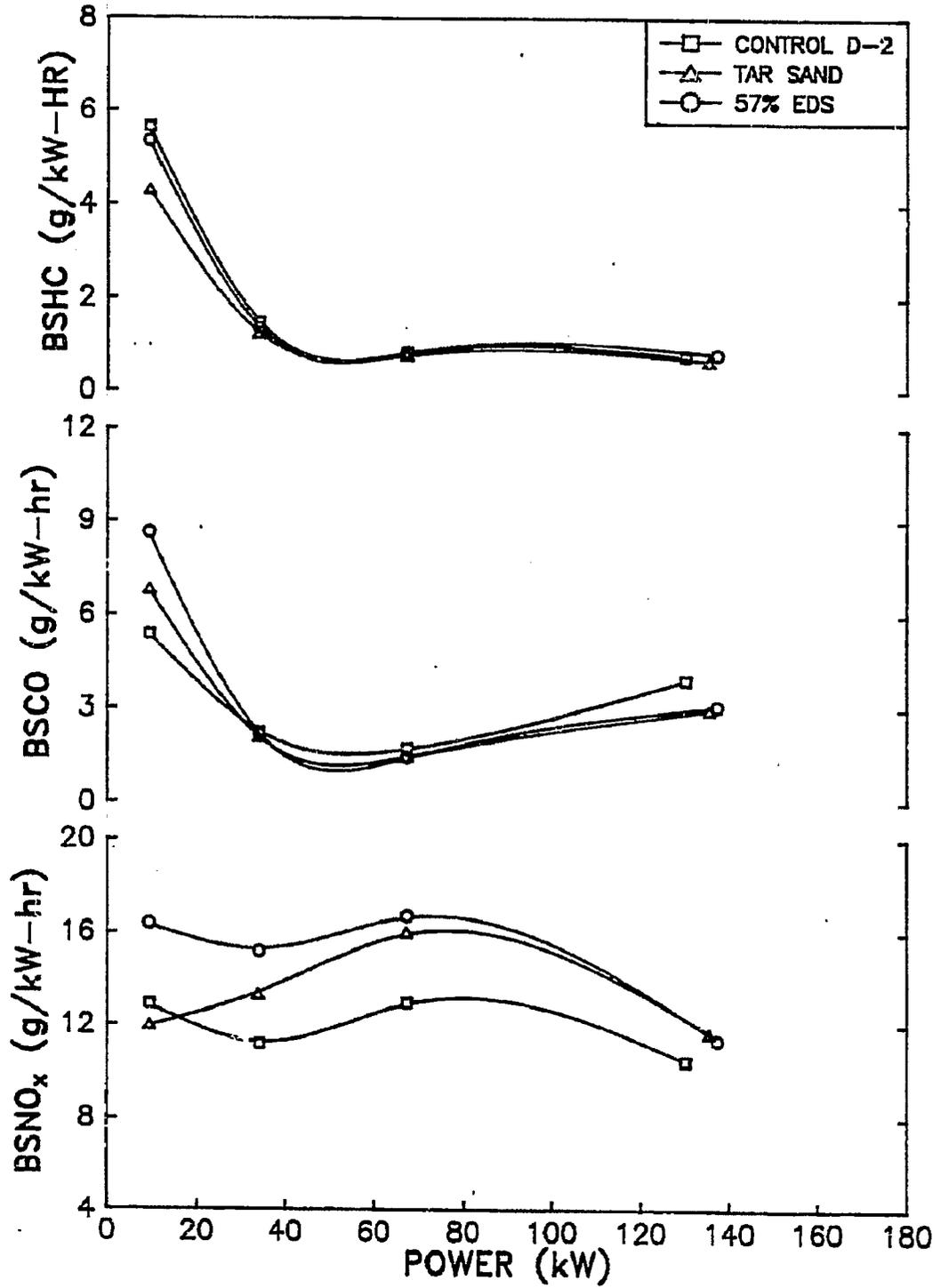
**FIGURE 6.39. BRAKE SPECIFIC EMISSIONS AT 1400 RPM, PHASE II SIMULATED AIR-TO-AIR AFTERCOOLER AND HIGH PRESSURE FUEL INJECTION**
