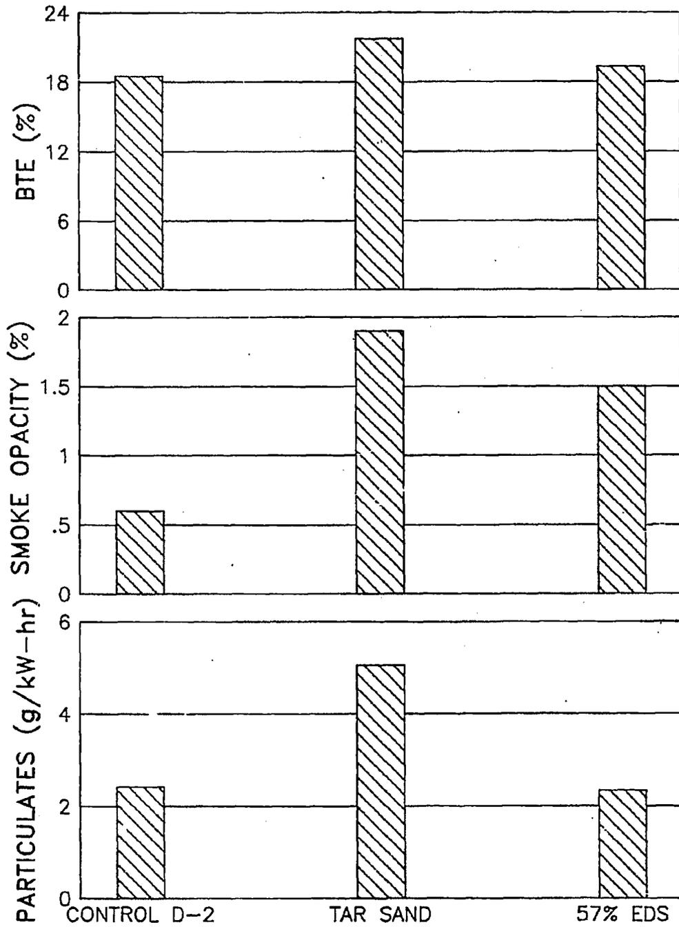
**FIGURE 6.32. PERFORMANCE RESULTS AT IDLE, PHASE II SIMULATED AIR-TO-AIR AFTERCOOLER**
