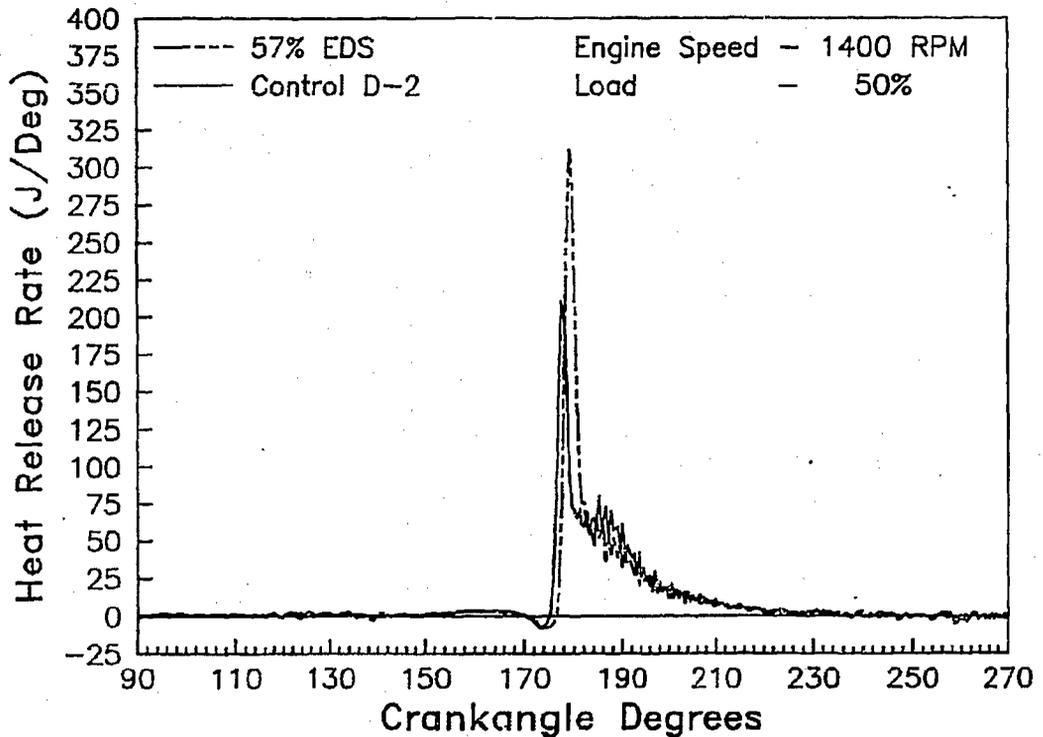
**FIGURE 6.35. HEAT RELEASE RATE FOR 57 PERCENT EDS AND CONTROL DF-2 FUELS AT 1400 RPM, 50 PERCENT LOAD, SIMULATED AIR-TO-AIR AFTERCOOLER**
