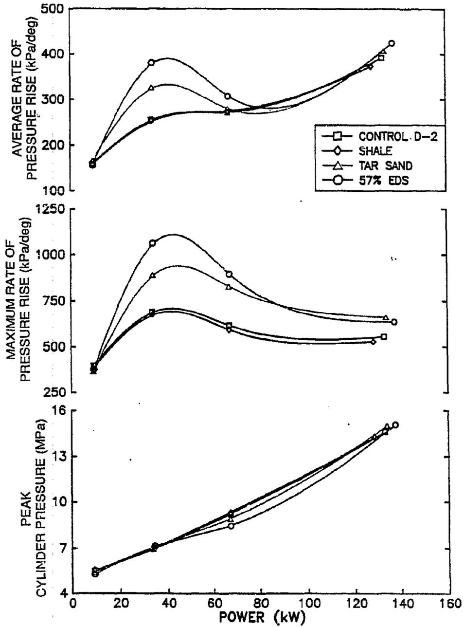
FIGURE 6.14. PEAK CYLINDER PRESSURES AND RATES OF PRESSURE RISE FOR EACH FUEL AT 1400 RPM
