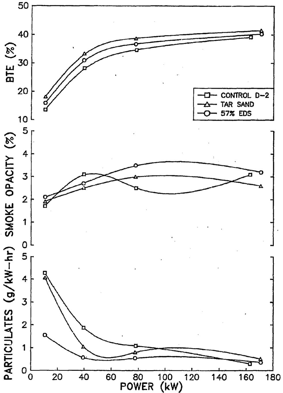
FIGURE 6.36. PERFORMANCE RESULTS AT 2200 RPM,
