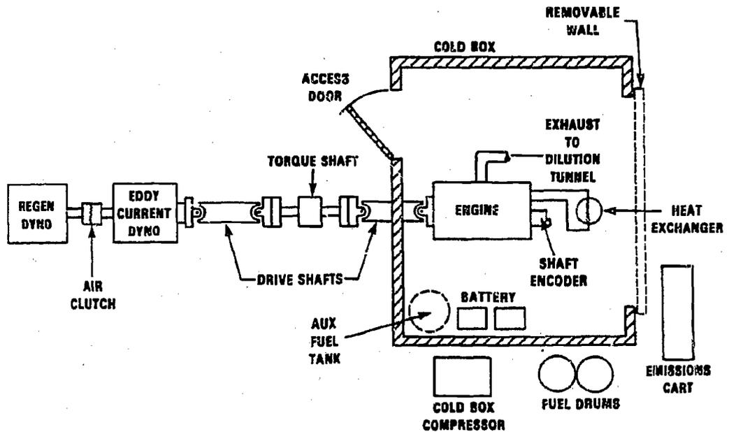
FIGURE 5.1. SCHEMATIC OF THE ENGINE IN THE TEST CELL
