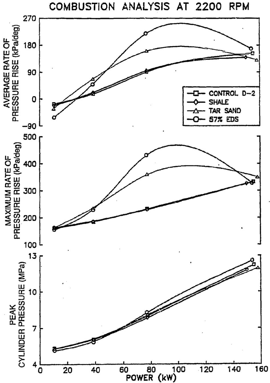
**FIGURE 6.15. PEAK CYLINDER PRESSURES AND RATES OF PRESSURE RISE FOR EACH FUEL AT 2200 RPM**
