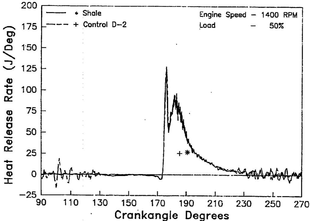
**FIGURE 6.7. HEAT RELEASE RATE FOR SHALE AND CONTROL D-2 FUELS AT 1400 RPM, 50 PERCENT LOAD**
