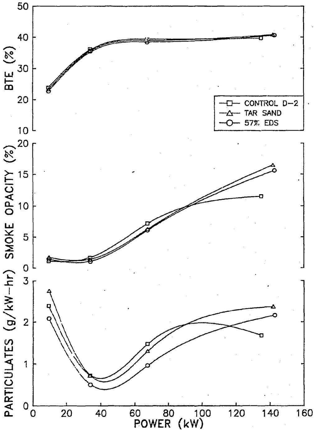
FIGURE 6.30. PERFORMANCE RESULTS AT 1400 RPM,
