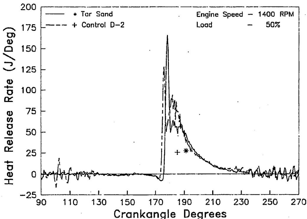
**FIGURE 6.8. HEAT RELEASE RATE FOR SHALE AND CONTROL D-2 FUELS AT 1400 RPM, 50 PERCENT LOAD**
