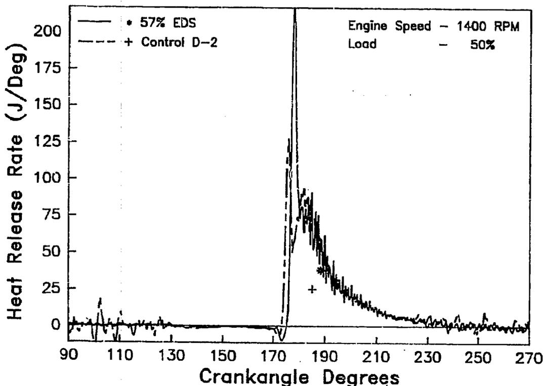
**FIGURE 6.9. HEAT RELEASE RATE FOR 57 PERCENT EDS AND CONTROL D-2 FUELS AT 1400 RPM, 50 PERCENT LOAD**
