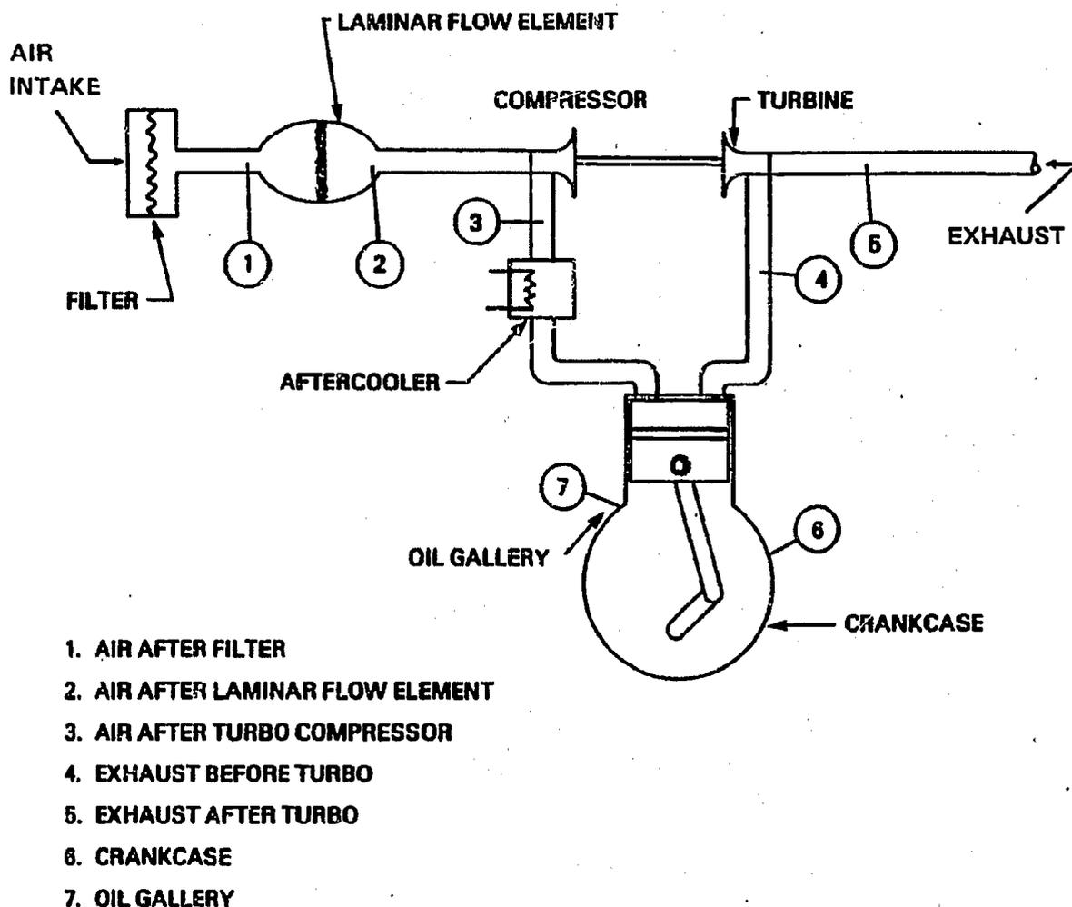
**FIGURE 5.5. TRANSDUCER PRESSURE MEASUREMENT POINTS**
