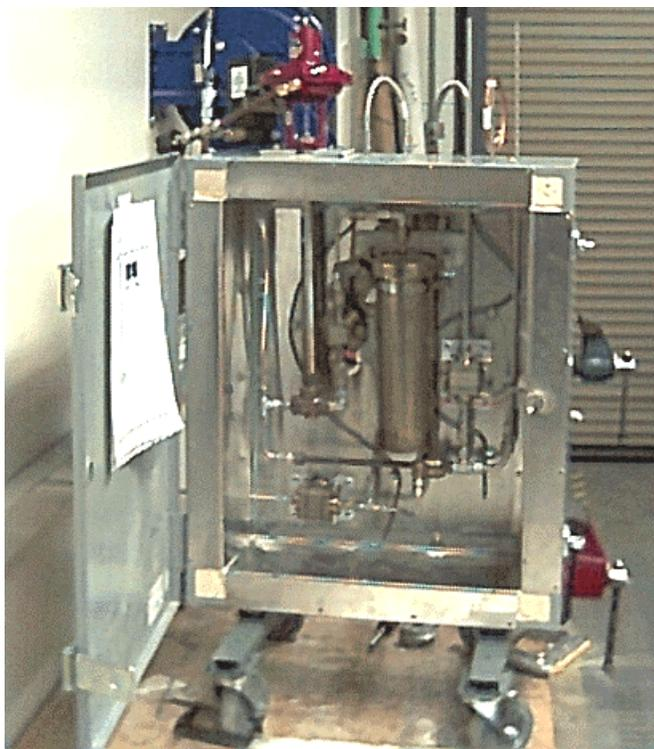
**Figure 2. Heated manifold box used during catalyst testing.**
