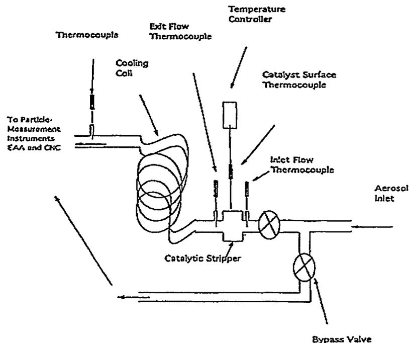
Typically more than 99% of the nanoparticles disappear by 300 C, the residue is likely to be metallic ash
