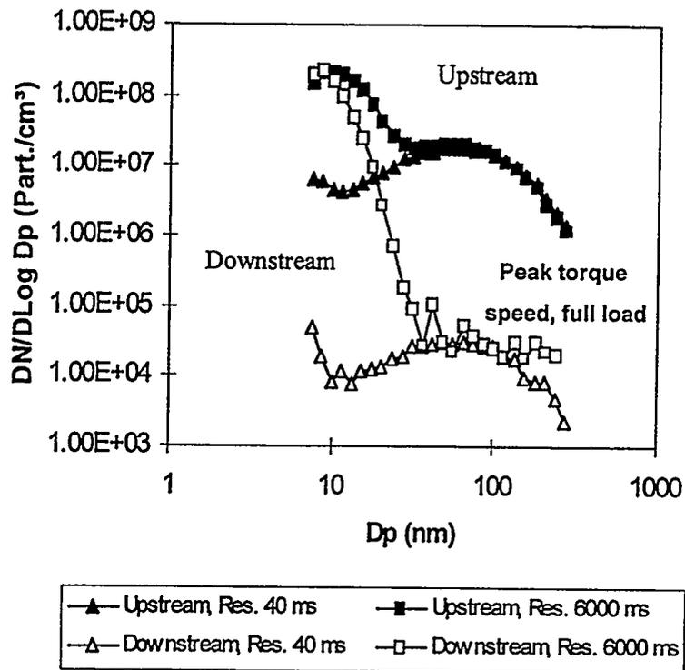
Our results suggest nanoparticles are mainly volatile, we have demonstrated this with a catalytic stripper
