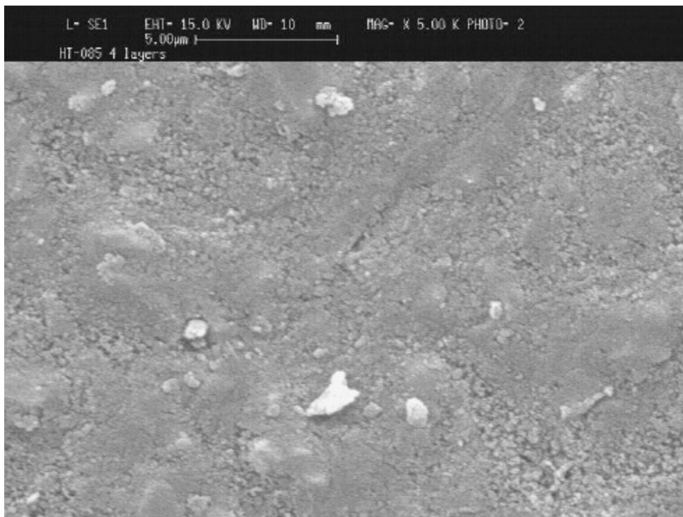
Figure 4.11 SEM photomicrograph of hydrotalcite membranes prepared from impregnation (4 times). Magnification: 1K top, 5K bottom.
