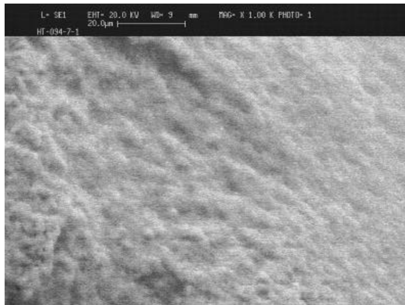
Figure 2 SEM photomicrograph of hydrotalcite membrane prepared via slip casting using the half of the particle density used for Figure 1 (HT-094-7-1)
