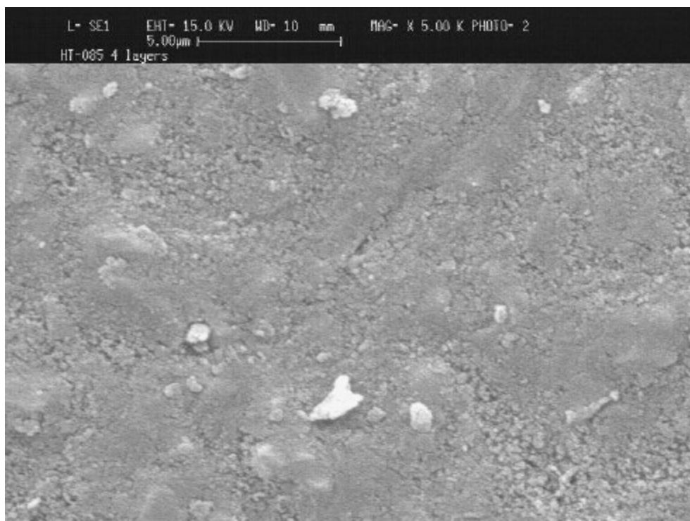
Figure 5a SEM photomicrograph of hydrotalcite membranes prepared from impregnation (4 times). Magnification: 1K top, 5K bottom.
