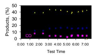
The fuel processor operated most effectively at 28 mL/min, equivalent to 5 kWe, with maximum hydrogen yield and CO elimination. Increasing the fuel feed rate from 14 to 28 mL/min increased the hydrogen (40 to 43%, dry) and carbon dioxide (12 to 16%, dry) concentrations, with a significant reduction in carbon monoxide from 7 to 3%. At this feed rate, the processor produced 75 L/min of hydrogen, sufficient to generate 4.2 kWe in a fuel cell stack.
