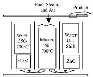
Fig. 2. Schematic of the integrated fuel processor.
