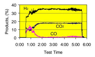
Fig. 3. Product composition from test with isooctane at fuel feed of 14 mL/min (equivalent to 2.5 kWe).
