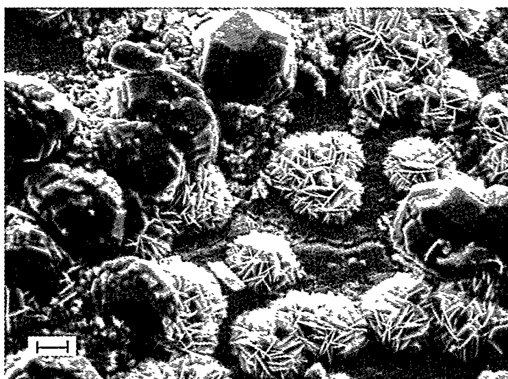
Fig. 5-30. Scanning Electron Image of Hydrated Glass Surface Showing Complex Silicate Precipitates
