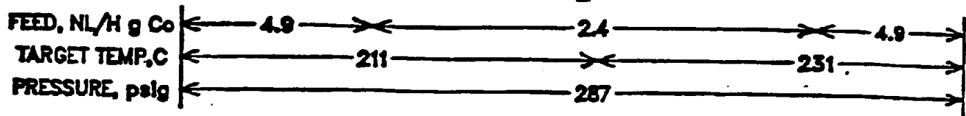
FIGURE 57 PLT 700A RUN 73 Co,Ru on 50/50 Al 2 O 3 /TiO 2 6531-134 w/7.45% Co via aq. Impreg 2:1 H 2 :CO In feed 13g Active in 160g SiO 2 sand
