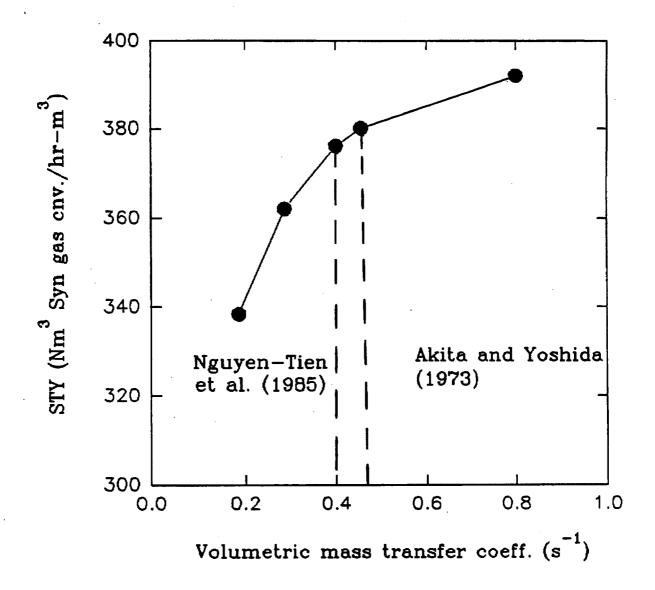
Figure 15. Effect of volumetric mass transfer coeff. on space time yield
