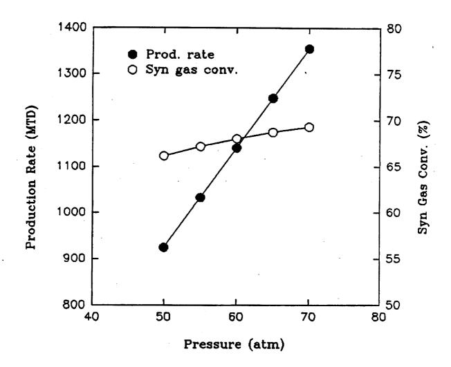
Figure 4. Effect of pressure on methanol production rate and hydrogen conversion
