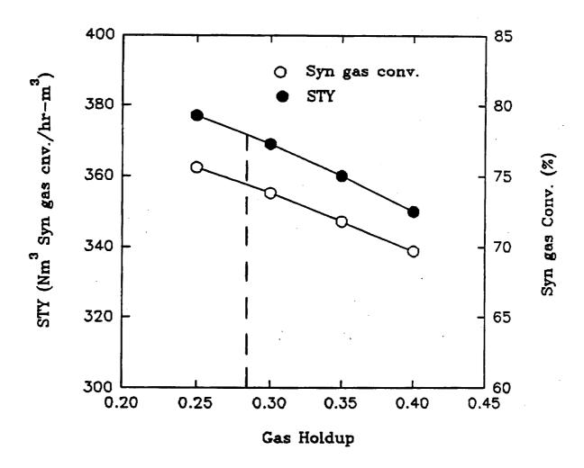
Figure 14. Effect of gas holdup on space time yield and syn gas conversion
