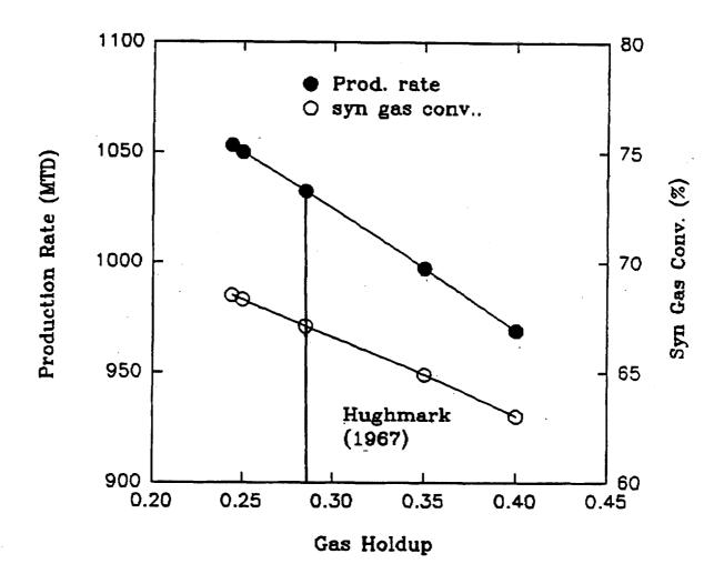
Figure 7. Effect of gas holdup on methanol production rate and hydrogen conversion
