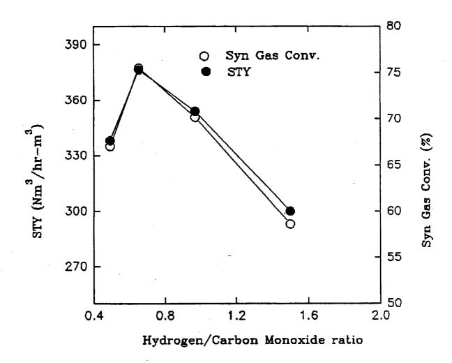
Figure 13. Effect of Hydrogen to Carbon Monoxide ratio on Syn Gas conversion
