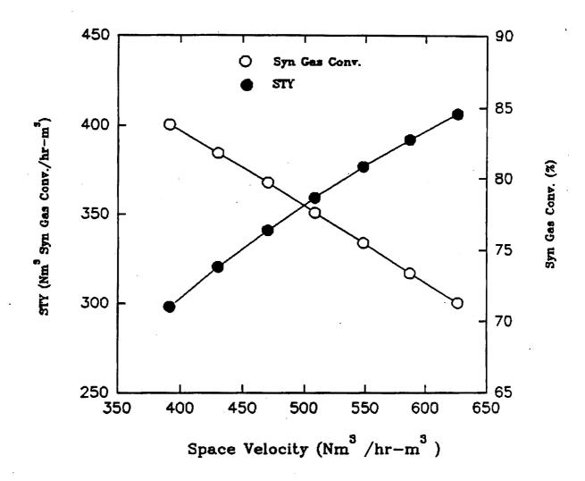
Figure 12. Effect of space velocity on space time yield and syn gas conversion
