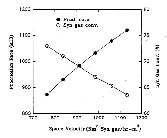
Figure 5. Effect of space velocity on methanol production rate and syn gas conversion.
