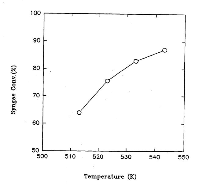
Figure 10. Effect of temperature on syngas conversion
