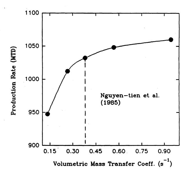
Figure 8. Effect of volumetric mass transfer coefficient on methanol production rate
