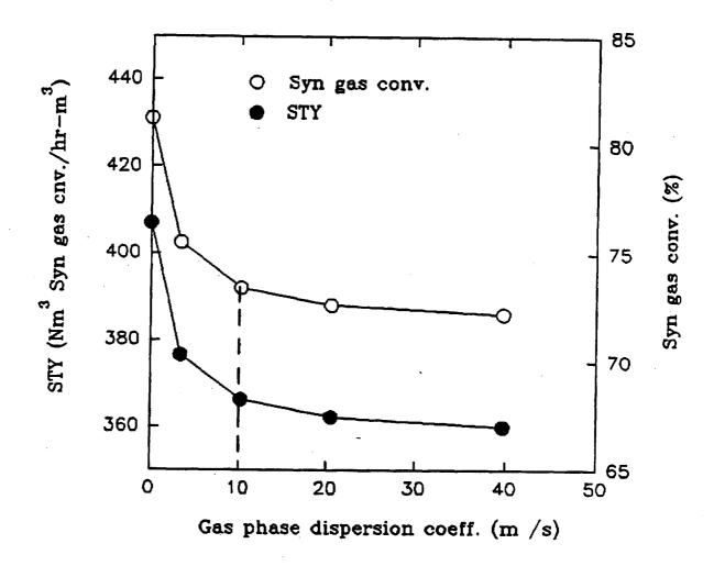
Figure 16. Effect of gas phase dispersion on space time yield and syn gas conversion
