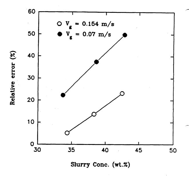
Figure 2. Effects of slurry concentration on relative error between predicted and experimental rates
