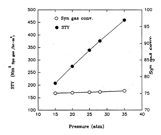
Figure 11. Effect of pressure on space time yield and syngas conversion
