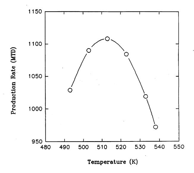
Figure 3. Effect of temperature on methanol production rate
