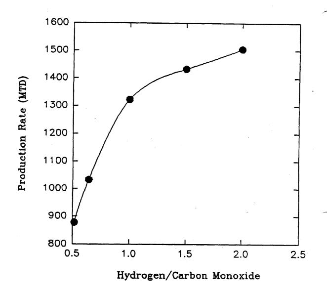
Figure 6. Effect of hydrogen to carbon monoxide ratio on methanol production rate.
