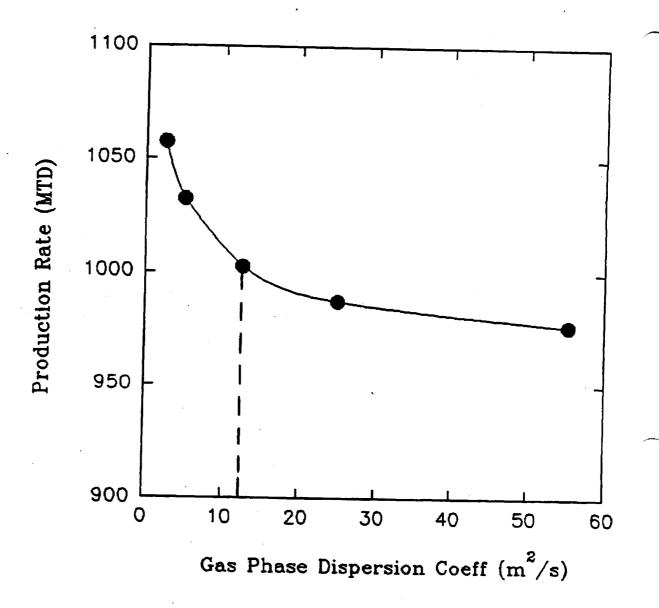
Figure 9. Effect of gas phase dispersion on methanol production rate
