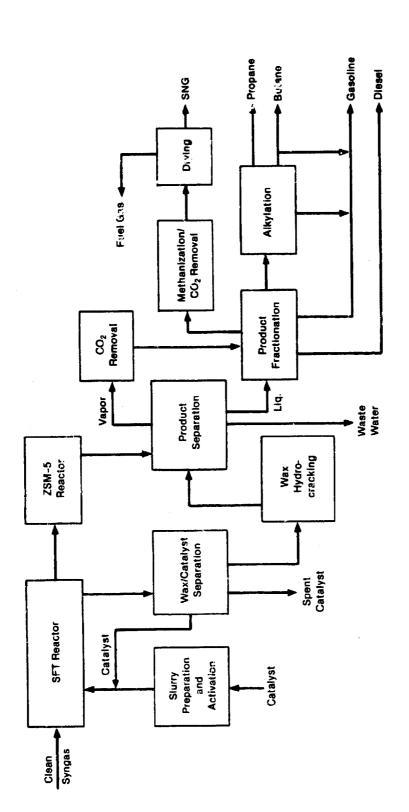
FIGURE 4-1 A SIMPLIFIED FLOW CHART FOR MOBIL HIGH-WAX CASE
