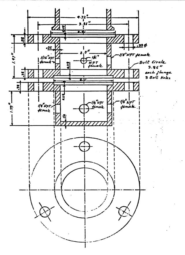
Figure 4: Support and distributor for the BC2
