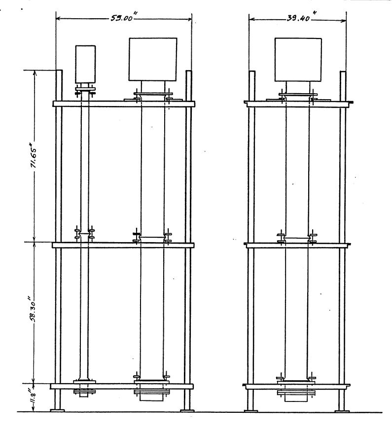
Figure 8: Frame support structure for bubble columns
