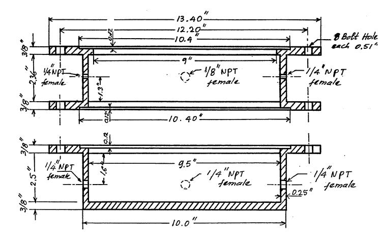
Figure 5. Support and distributor for the BC1
