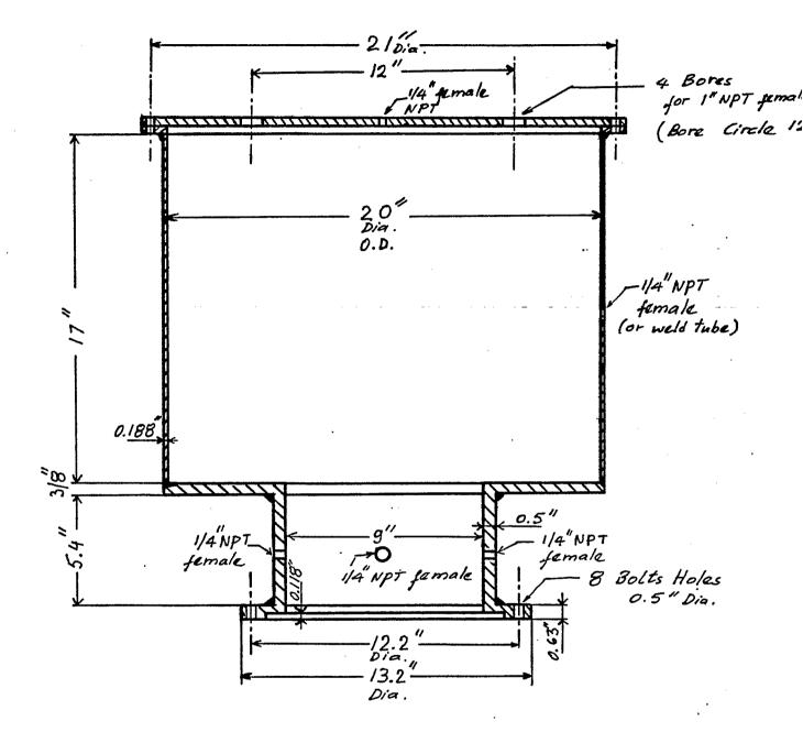
Figure 3: Expansion unit for the 9" ID bubble column (BC1)
