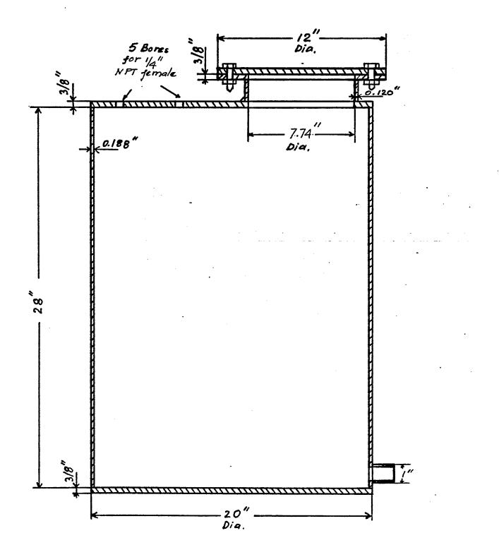
Figure 7: Storage tank for wax
