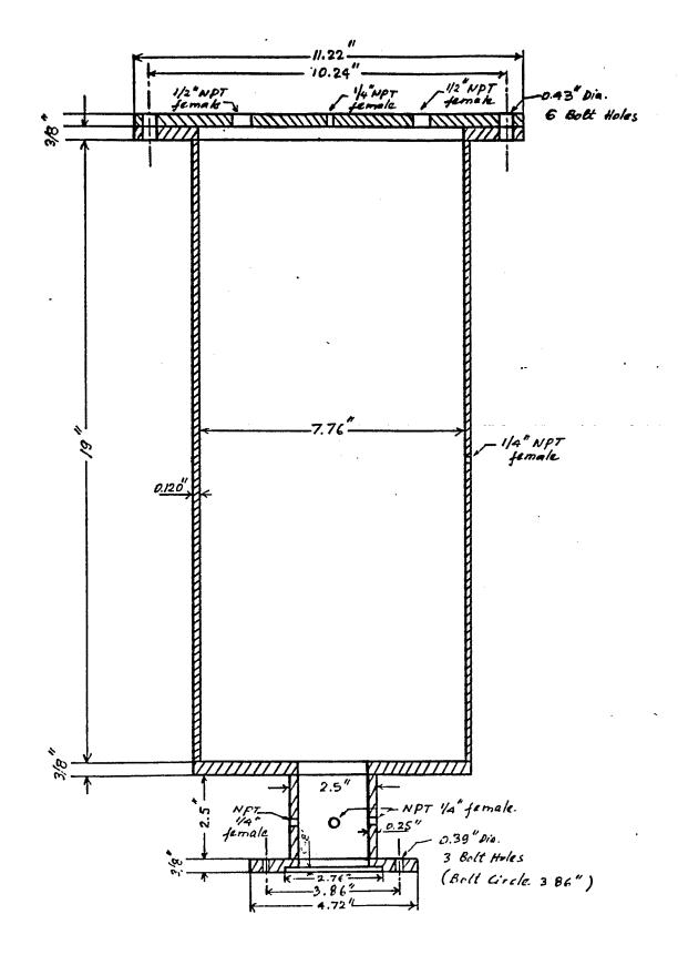
Figure 2: Expansion unit for the 2" ID bubble column (BC2)
