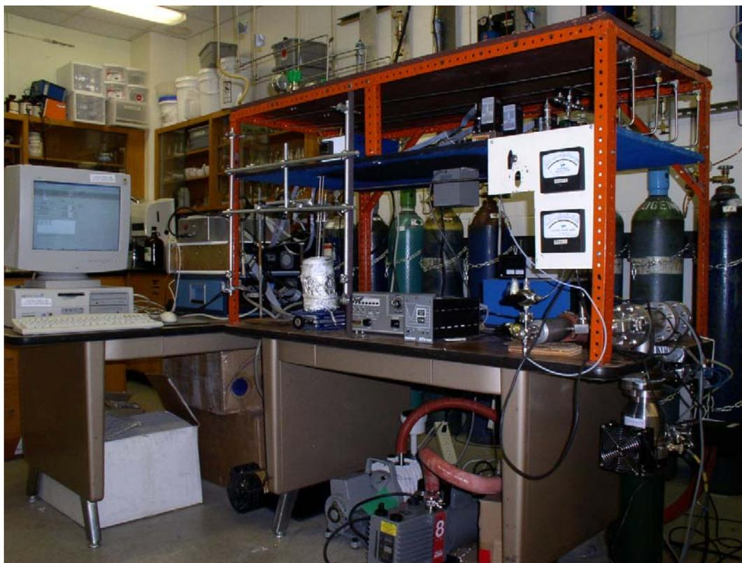
**Fig. 2.** Mass Spectrometry-TPD System
