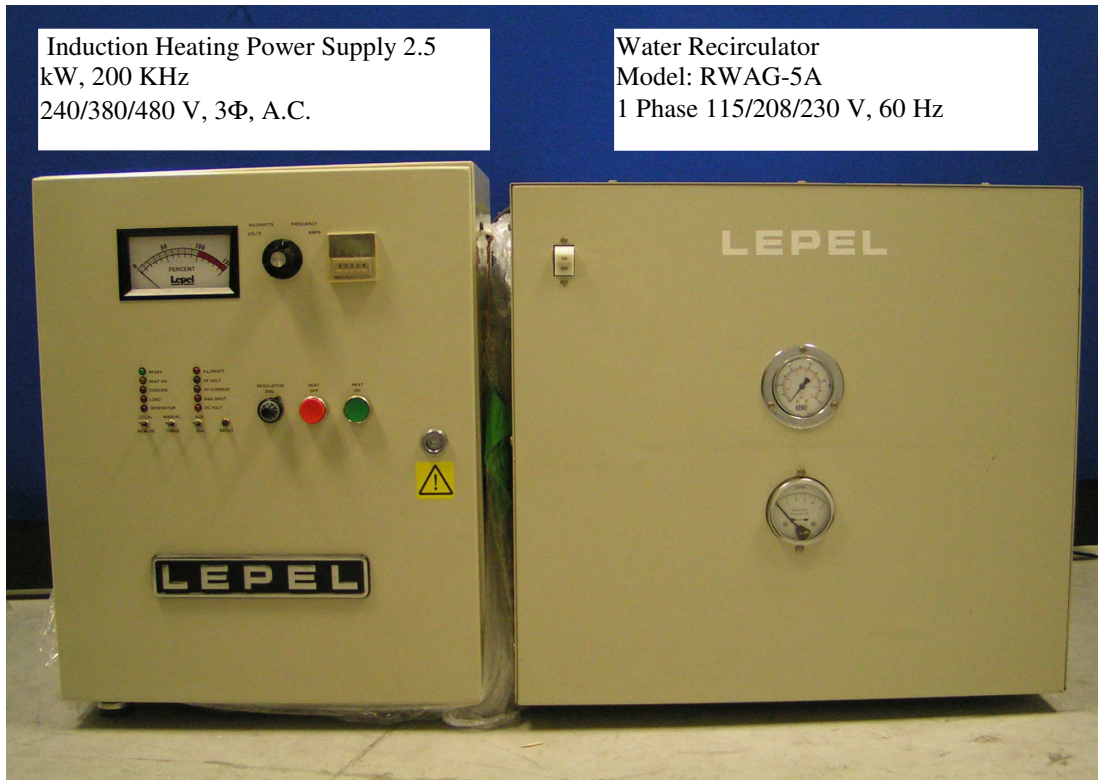
Fig. 3 Photograph of a power supply for the induction heating coil of the HTHP cell.
