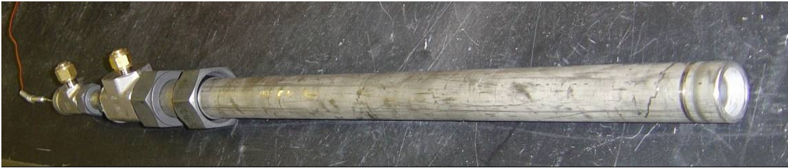
Figure 3. Membrane holding tube. The disk membrane will be attached to the end of this tube, which will be inserted into the center of the tube in Figure 2 (b)
