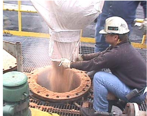
FIGURE 5-Emptying Totes Into Tank
