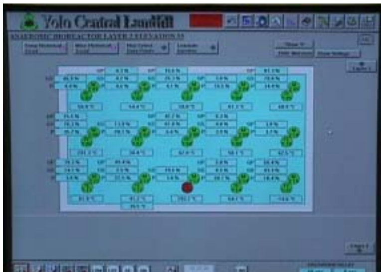
Image 7-3: NE anaerobic cell, layer 2 screen depicting temperature and moisture data.
