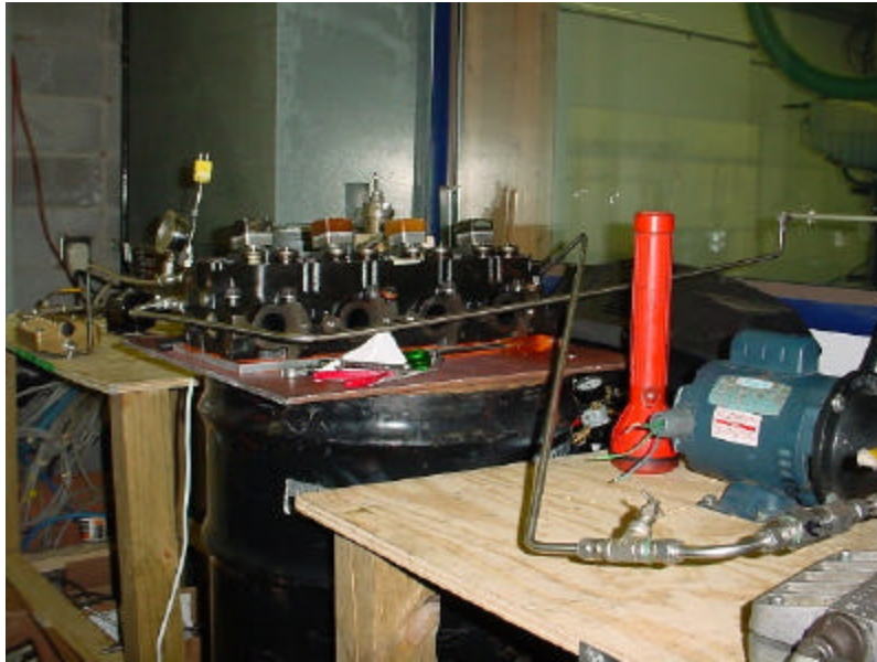
Fig. 29. Fuel Injector Test Stand During Fabrication Process
