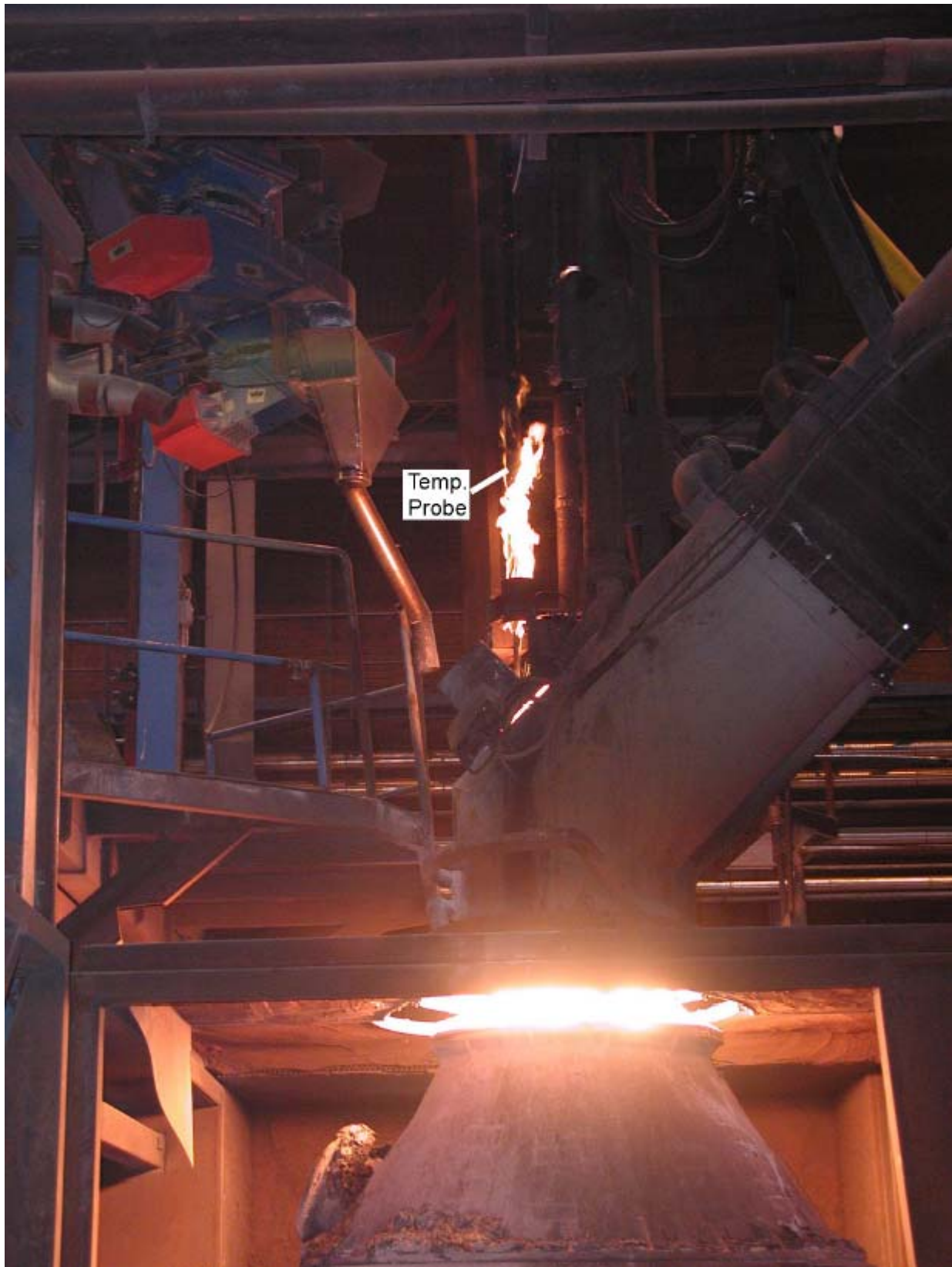
Figure 5. Temperature Probe Removal During Decarburization for Universal Converter
