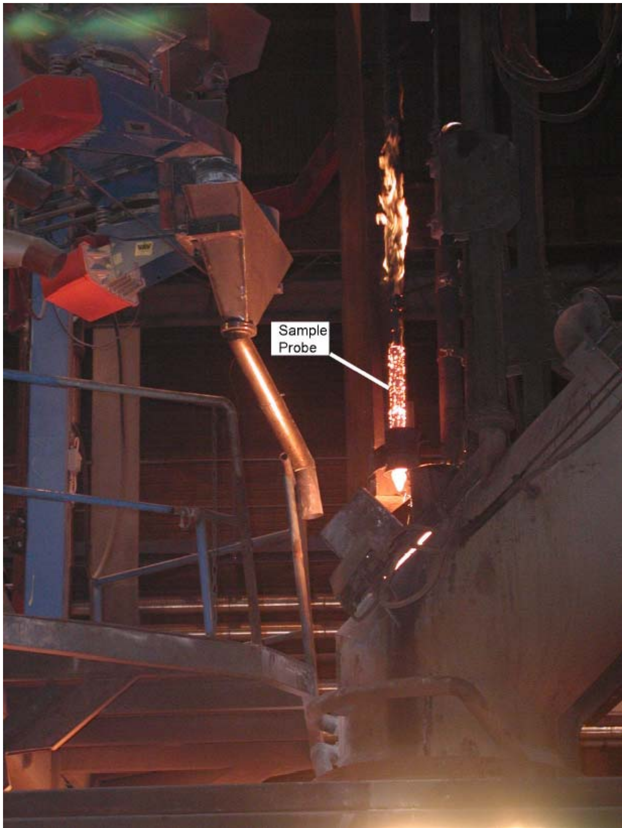
Figure 6 Metal Sample Probe Removal During Decarburization
