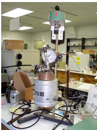
Figure 7. Batch Processing Slurry Reactor
