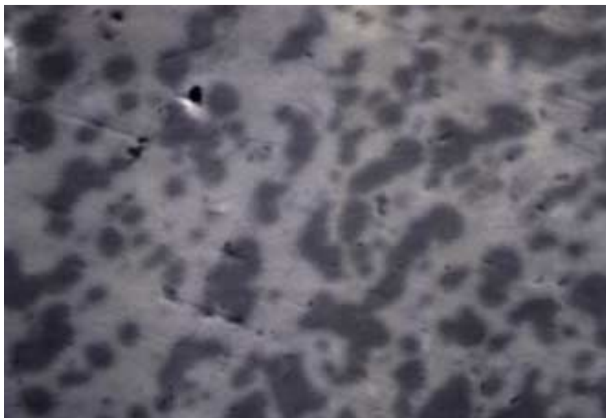
Figure 3. SEM image of a 54/46 wt.% ceramic/metal membrane. The dark regions are the metal phase and the light regions are the proton conducting ceramic.
