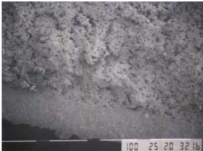
Figure 7. SEM image of a dense thin ceramic film (bottom) on a porous support of the same composition (top). The white bar represents 100 \mu\text{m} , which was also about the thickness of the film.
