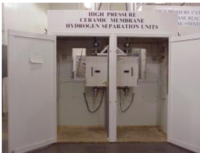
Figure 8. Photograph of the apparatus for evaluation of hydrogen separation membranes at high pressure.
