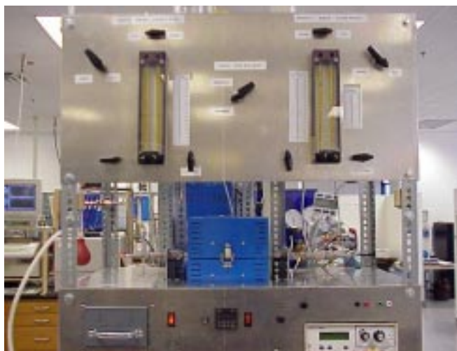
Figure 3. Photograph of the apparatus used for measurement of membrane proton and electron conductivity.
