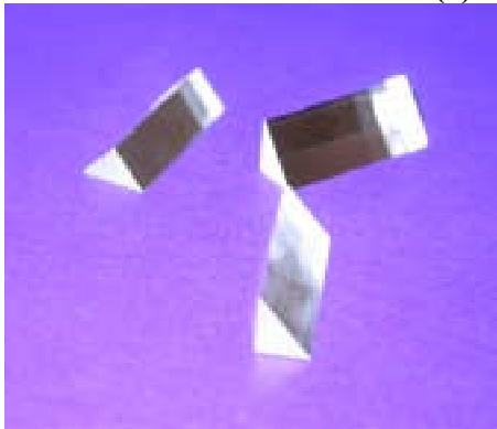
Figure 5.2. Single crystal sapphire right angle prism
