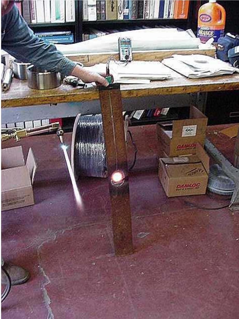
A temperature test with the pyrometer and a thermocouple was done to verify that the pyrometer system was working as designed. The thermocouple is the silver-colored wire taped on the carbon steel plate. The target area of the pyrometer is highlighted with white chalk on the steel plate. The bright spot on the carbon steel is the area that was heated up by a welding torch.
