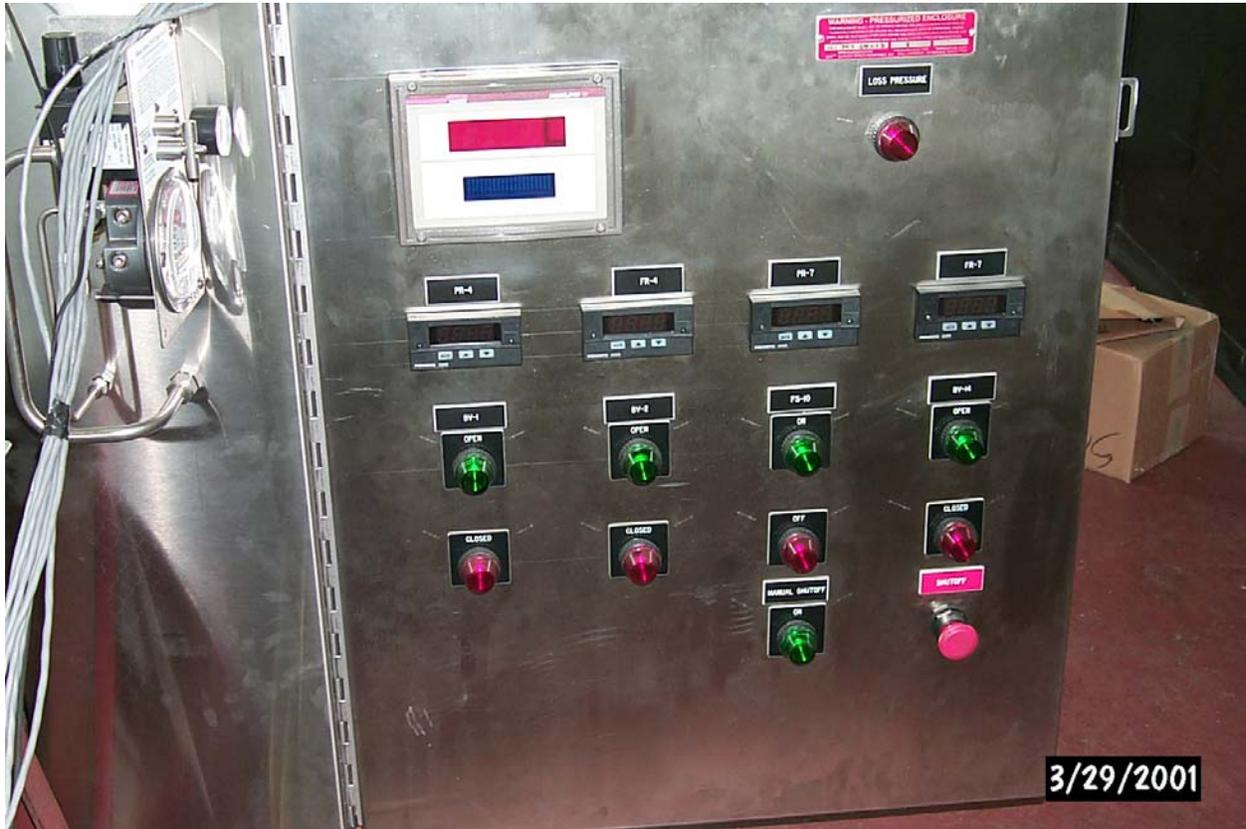
The front of the PLC panel contains the pyrometer temperature read out (upper left side.) Flow rates and pressure readings are shown in the digital displays. Status of valves (open/close) are shown as red/green lights. A manual shut down button in red is located on the lower right side.
