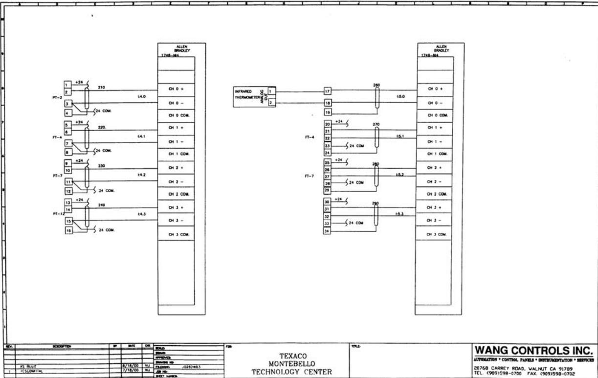
Figure 24 – PLC Connections - 3
