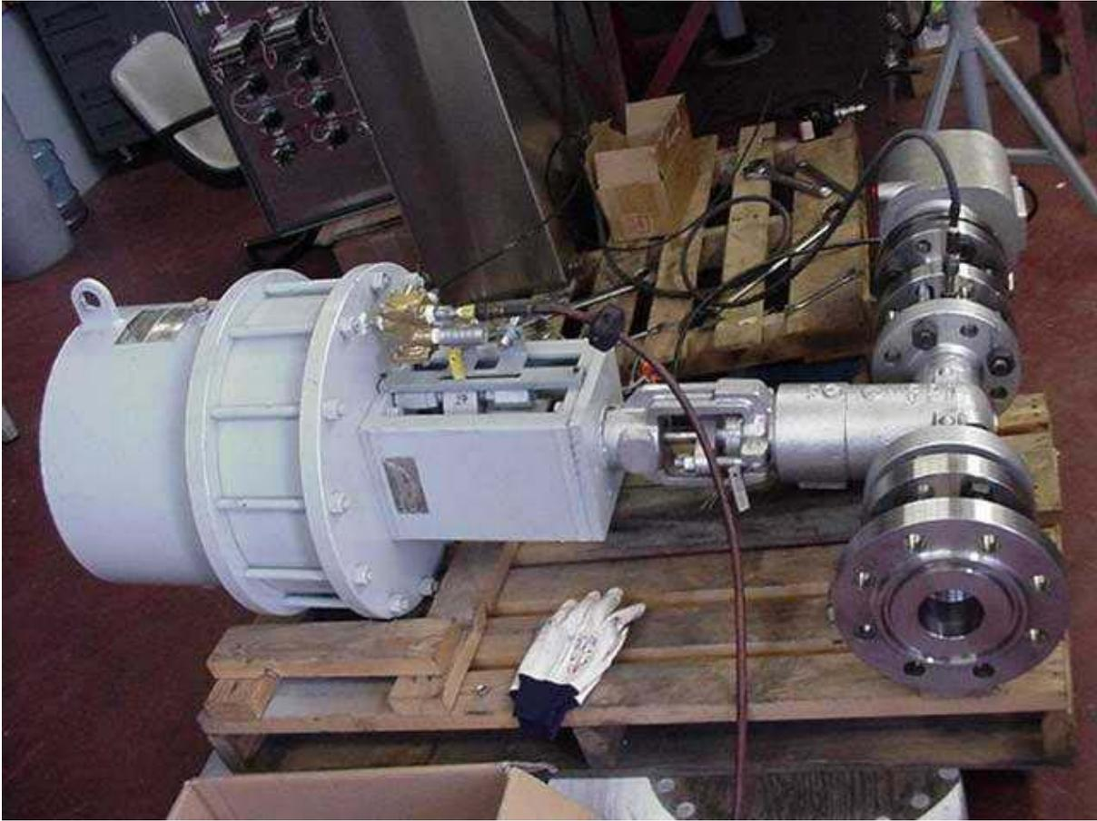
The shutdown valve is shown attached to the pyrometer camera (Oval silver-colored box in upper right side of the picture). Between the camera and valve are the spool pieces that house the quartz sight glasses and primary purge ring. The flanged spool piece in the lower right is the part that bolts on to the gasifier. This spool piece contains the secondary purge ring. The entire optical train assembly is heavy enough that it requires external support when connected to a gasifier.
