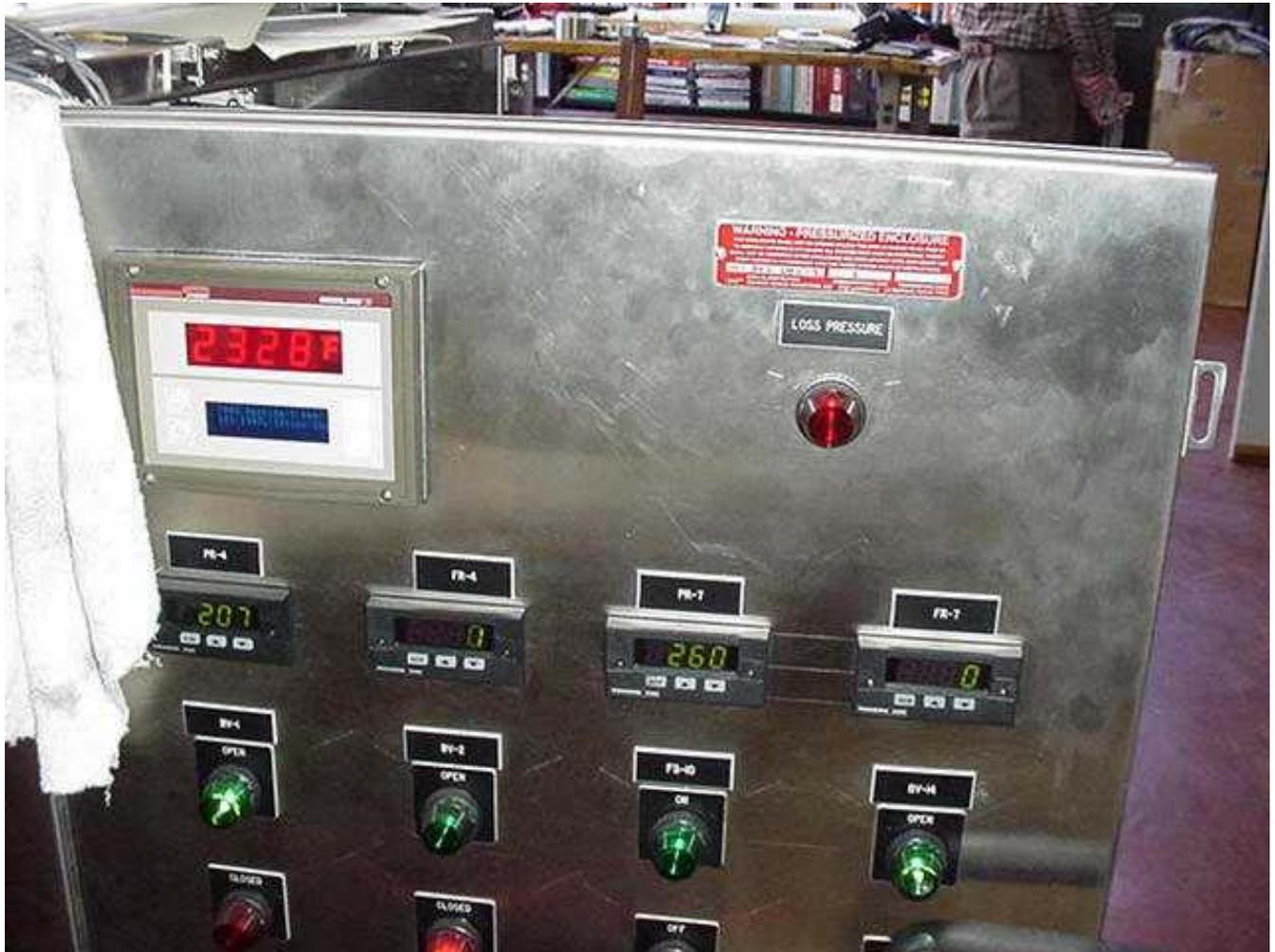
The pyrometer indicated a temperature of 1276 C (2328 F) while the thermocouple indicated a range of temperature that fluctuated above 1093 C (+2000 F). An accurate thermocouple temperature could not be attained due to the rapid changes in temperature of the metal and the relative crude test set up.
