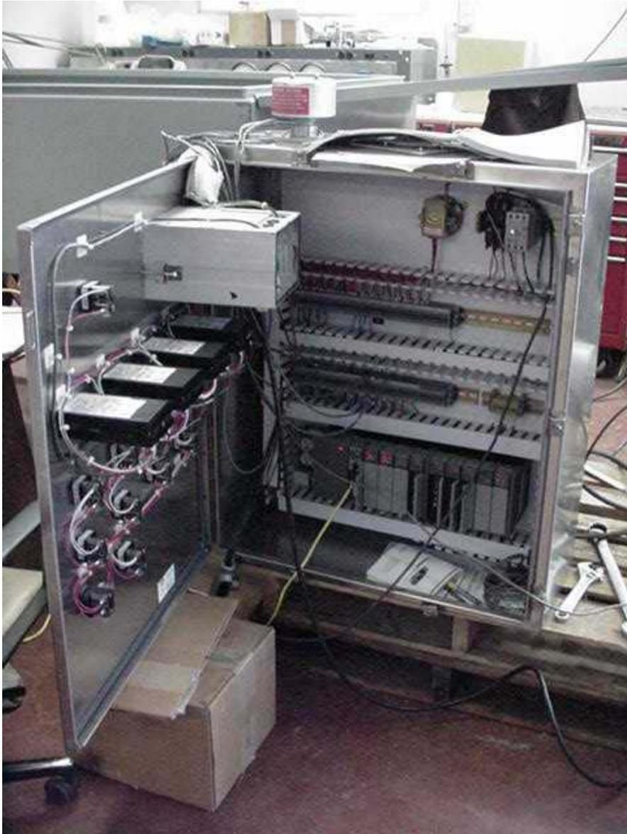
All electronic controls are housed in the PLC panel. The actual PLC is shown as the rectangular gray boxes on the bottom row of the panel box.
