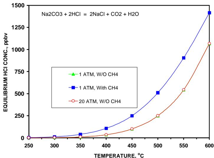
**Figure 3.3 – HCl Concentration Following Equilibration with  $\text{Na}_2\text{CO}_3$**
