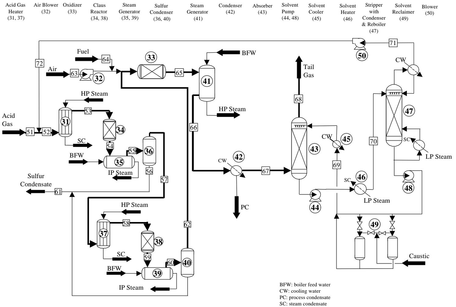
**Figure 4.5 - Conventional Syngas Cleaning - Sulfur Recovery Section**
