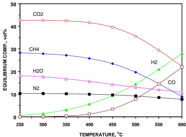
**Figure 3.1 - Equilibrium Syngas Composition in the Presence of CH<sub>4</sub>**
