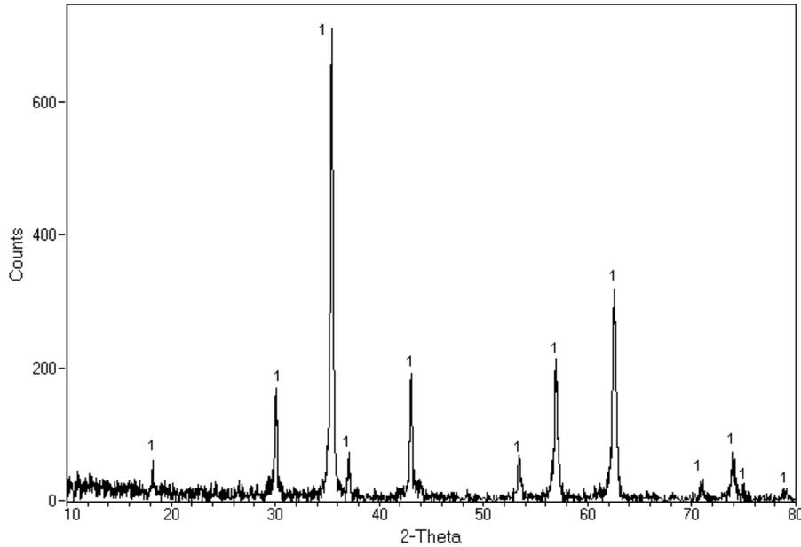
**Figure 3.29 – XRD Pattern of Highly Reduced Iron Oxide By-Product Sample**
