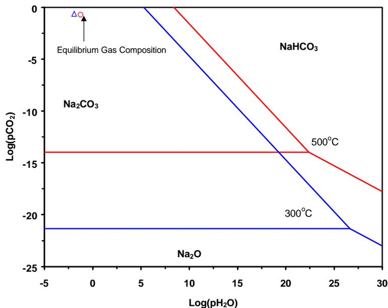
**Figure 3.6 – Predominance Area Diagram for the Na-C-H-O System at 300 and 500°C**
