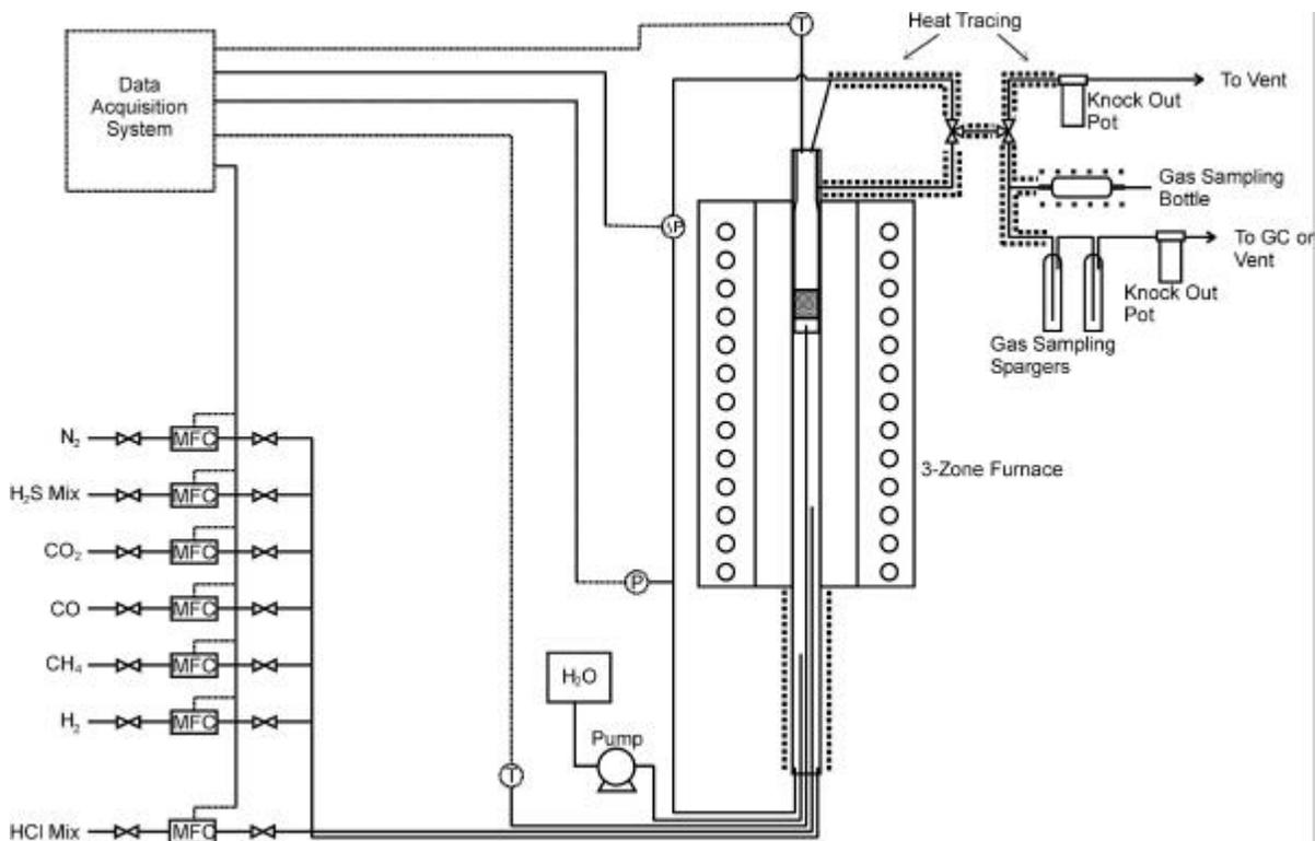
**Figure 3.15 – Schematic Diagram of the Packed-Bed Reactor Unit**
