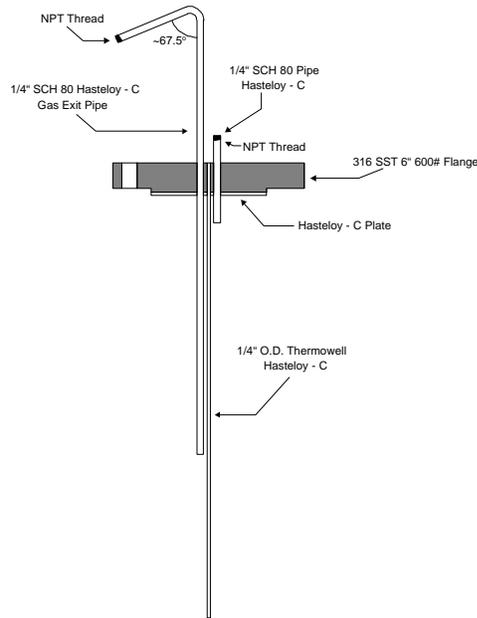
**Figure 3.19 – Details of Newly-Designed Top Flange**
