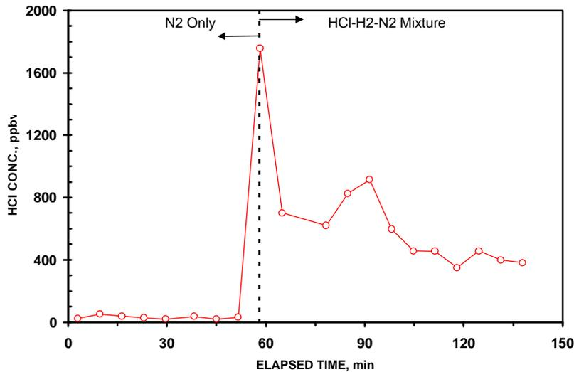
**Figure A9 – Measured HCl Concentration in a 400 ppbv HCl in H<sub>2</sub>-N<sub>2</sub> Mixture**
