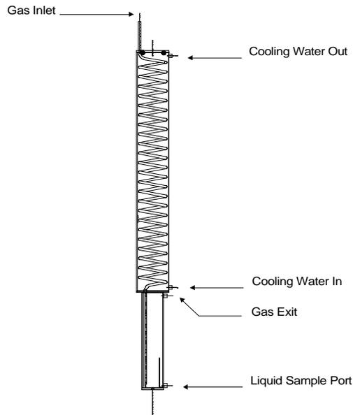
**Figure 3.20 – Details of Exit Reactor Gas Cooling System and HCl Recovery**
