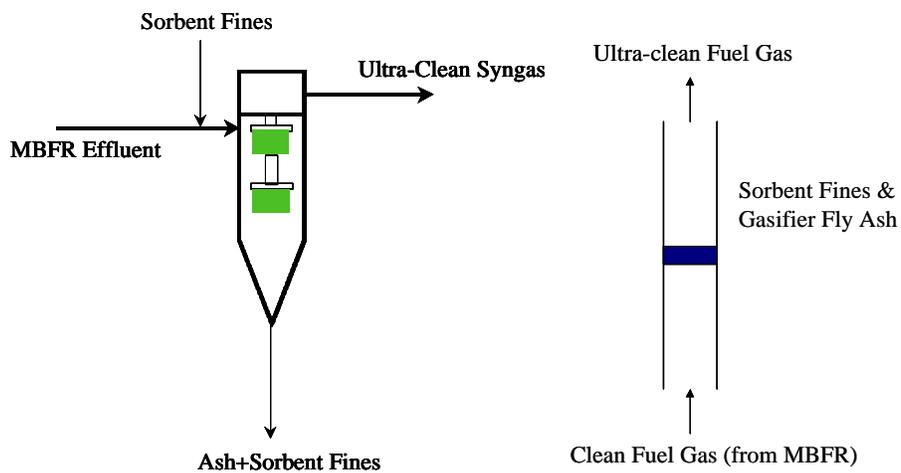
**Figure 3.14 – Laboratory Simulation of Barrier Filter-Reactor**
