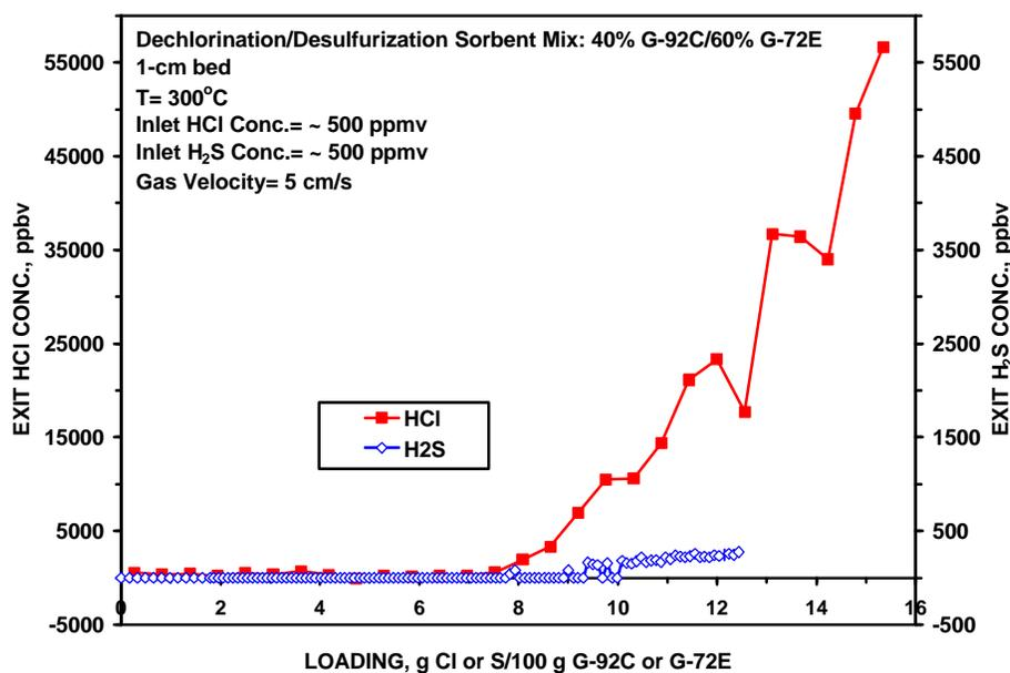
**Figure 3.60 – HCl and H<sub>2</sub>S Breakthrough Curves**
