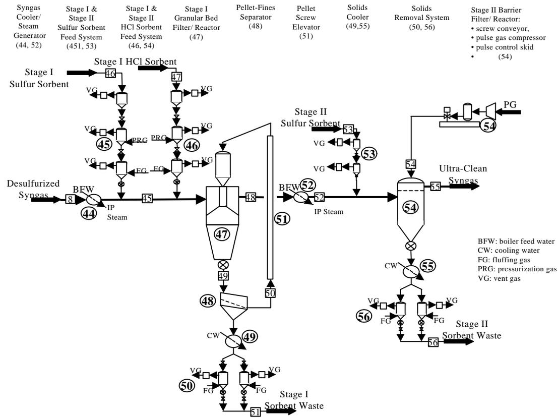
Figure 4.20 - Novel LP-SOFC Fuel Gas Cleaning Ultra-Clean Section
