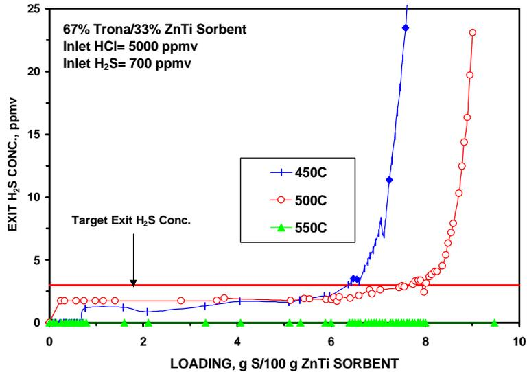
**Figure 3.40 – Effect of Temperature on Efficiency and Effective Capacity of GTI’s Zinc Titanate Sorbent for Sulfur Absorption**
