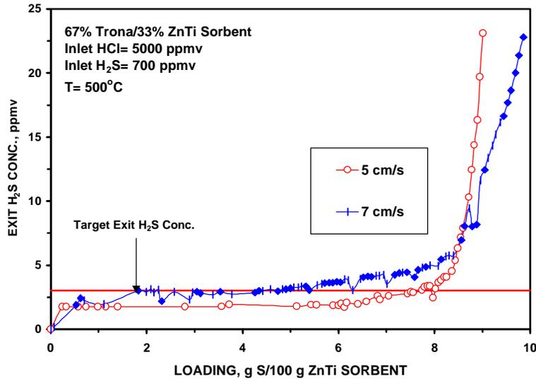
**Figure 3.38 – H<sub>2</sub>S Breakthrough Curves at Two Gas Velocities**
