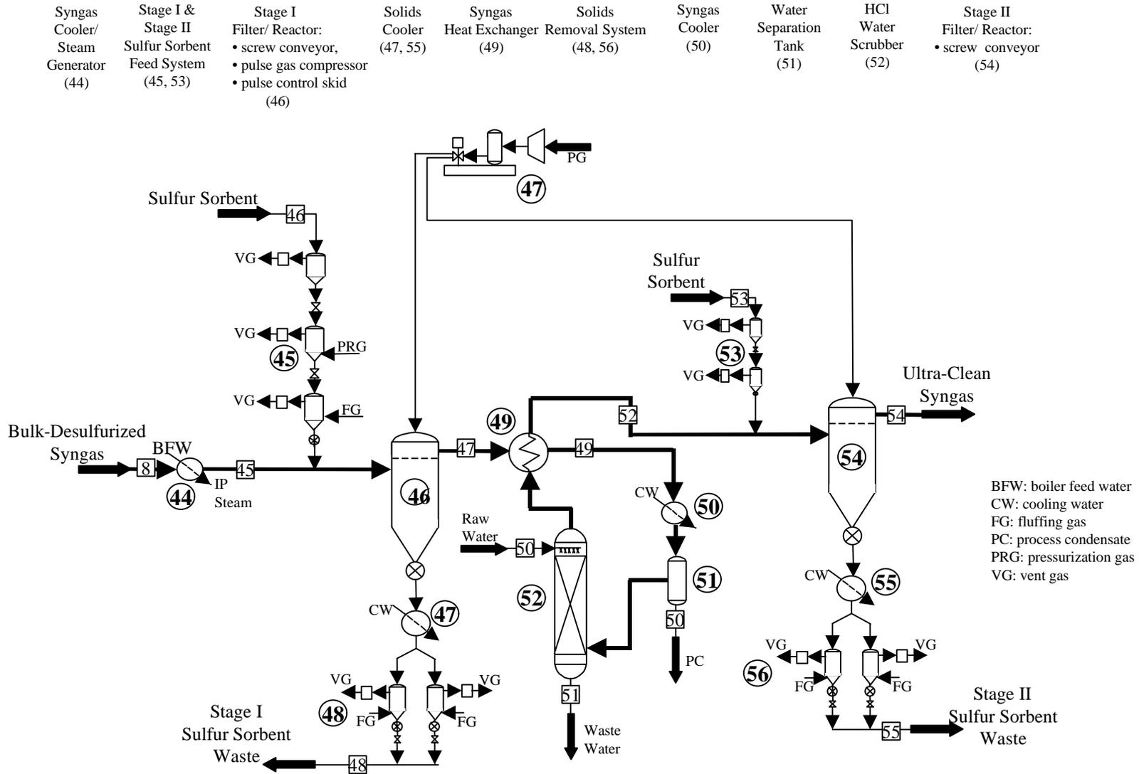
Figure 4.18 - Novel Syngas Cleaning - Ultra-Clean Section with HCl Scrubbing
