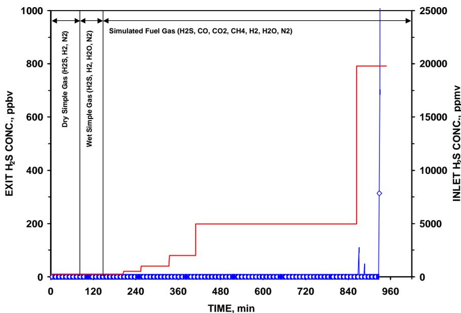
**Figure 3.56 – Scoping/Loading Test with Zingard 1000 Sulfur Absorber at 300°C**
