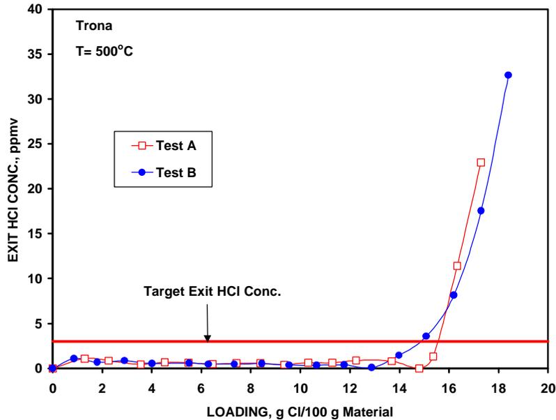
**Figure 3.23 – Reproducibility of the Results from Testing of Trona**
