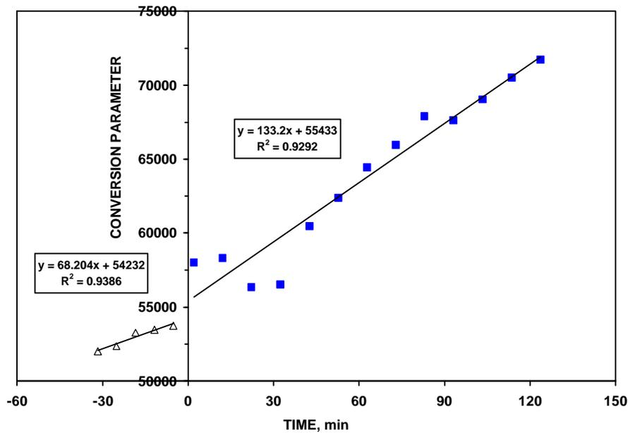
**Figure 3.51 – HCl Pre-breakthrough Concentration with G-92C at 350°C**
