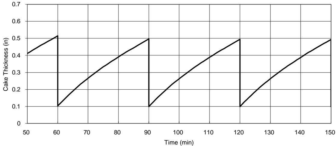
**Figure 4.16 - Stage I Barrier Filter-Reactor Plenum Filter Cake Thickness**
