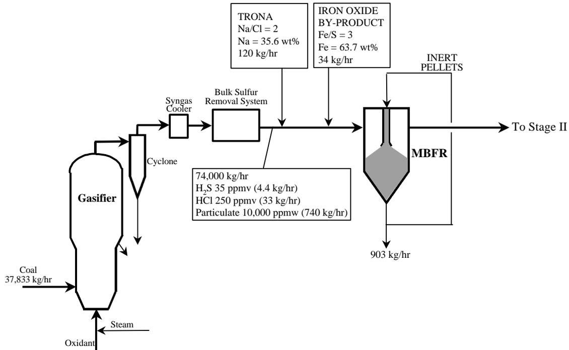
**Figure 3.30 – Material Balance for the Moving Bed Filter-Reactor with Iron Oxide By-Product Sulfur Sorbent**
