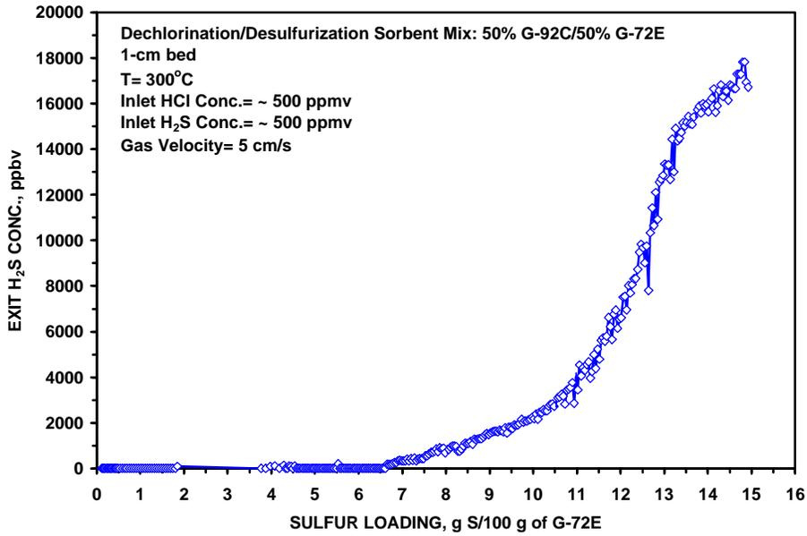
**Figure 3.58 – H<sub>2</sub>S Breakthrough Curve in Simultaneous HCl/H<sub>2</sub>S Removal**
