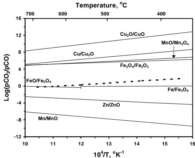
**Figure 3.7 – Superimposed Stability Diagrams for Cu, Fe, Mn, and Zn Oxides as a Function of Temperature and CO<sub>2</sub> to CO Ratio**
