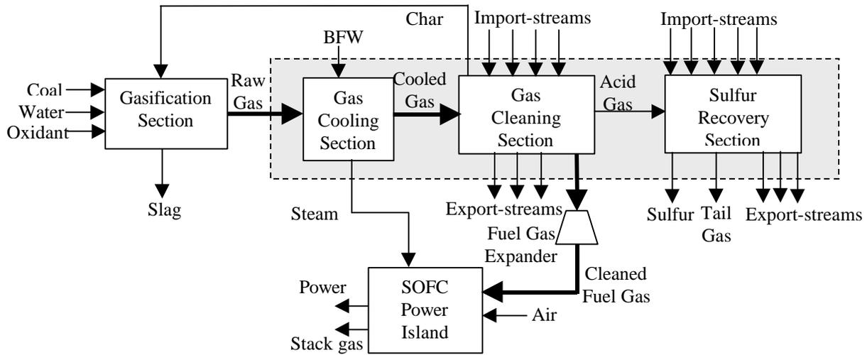
**High-Pressure SOFC Gas Cleaning**
