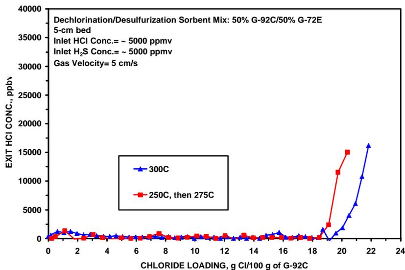
**Figure 3.62 – Effect of Temperature on Sorbent Effective Capacity**
