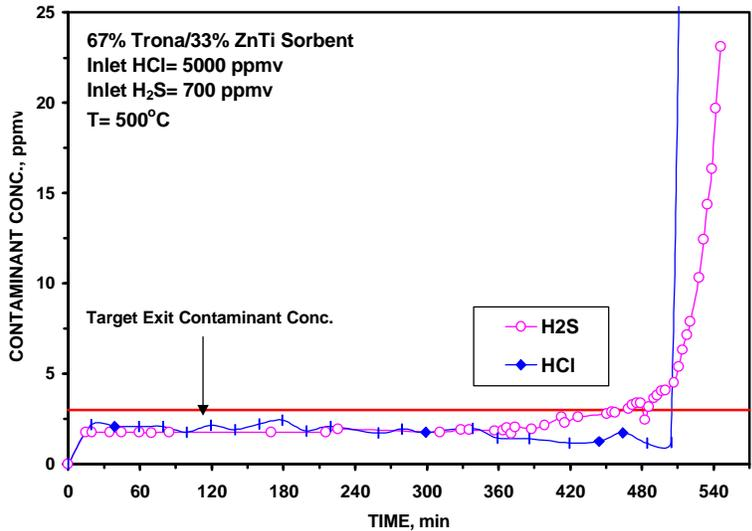
**Figure 3.36 – HCl and H<sub>2</sub>S Breakthrough Curves at 5 cm/s Gas Velocity**
