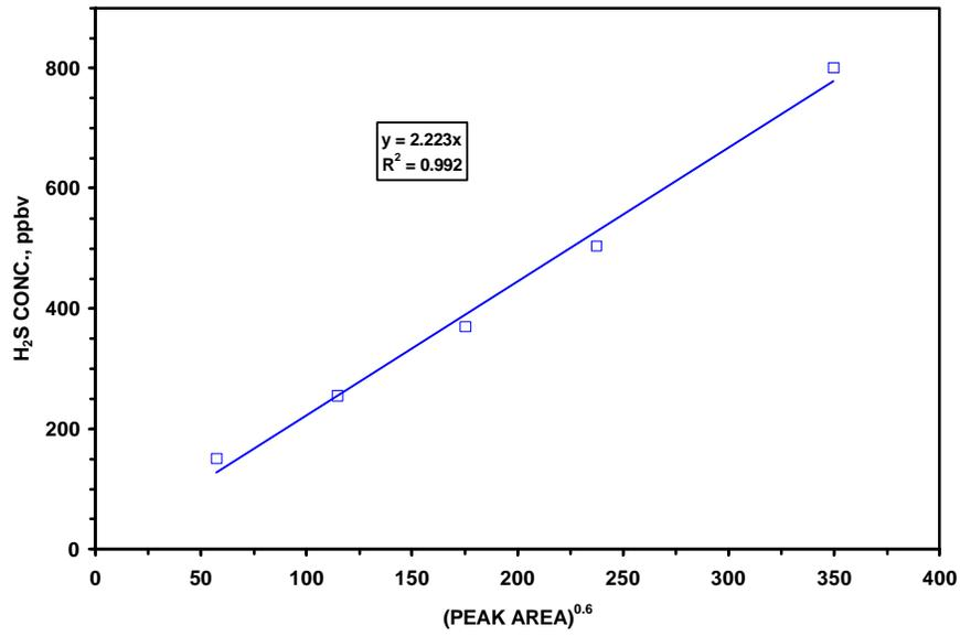
**Figure B3 – GC Calibration Curve for H<sub>2</sub>S Measurement at Trace Level**
