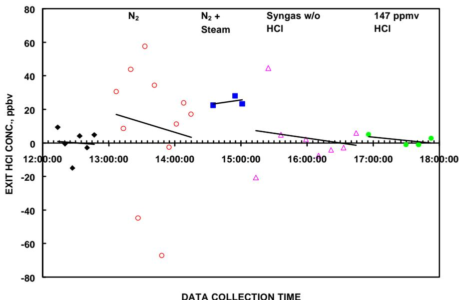
**Figure 3.43 – Scoping Dechlorination Test with the G-92C Material**
