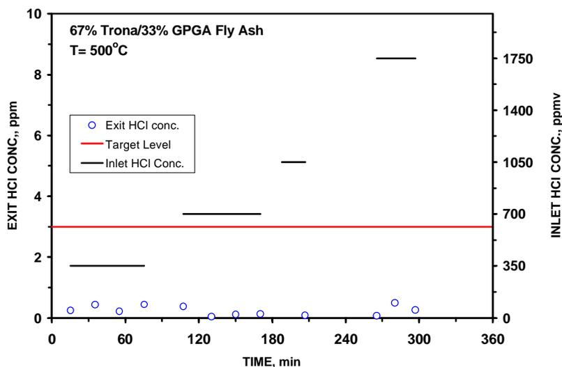
**Figure 3.25 – Effect of GPGA Material on Trona Performance**
