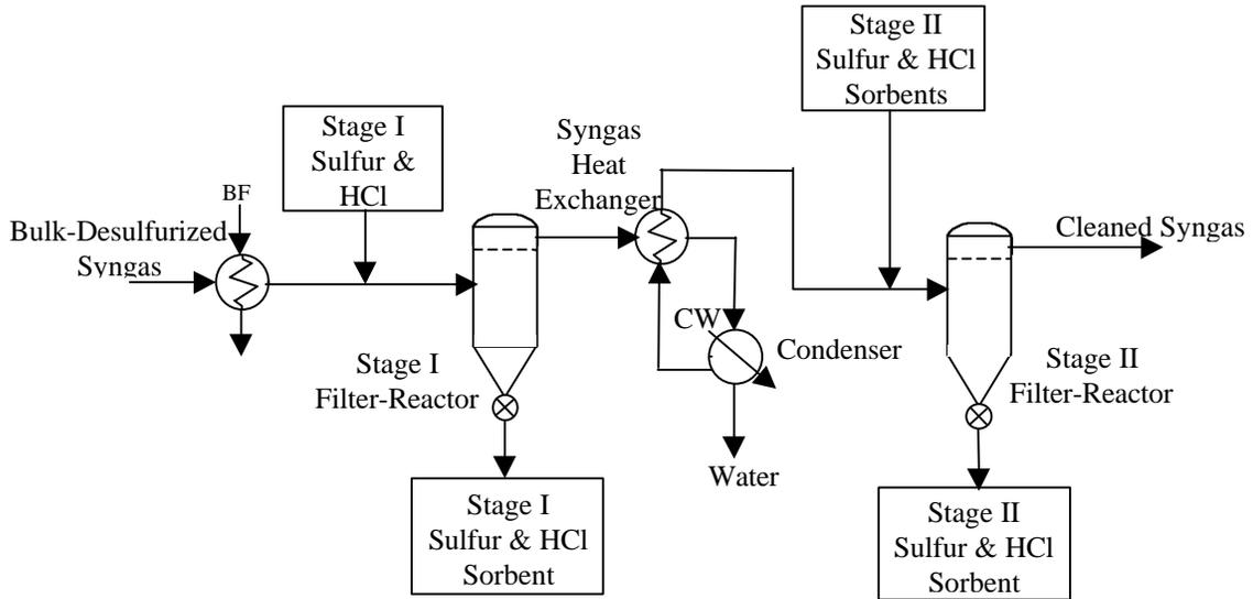
**Figure 4.9 – Ultra-Clean Section with Drying for Syngas Polishing**
