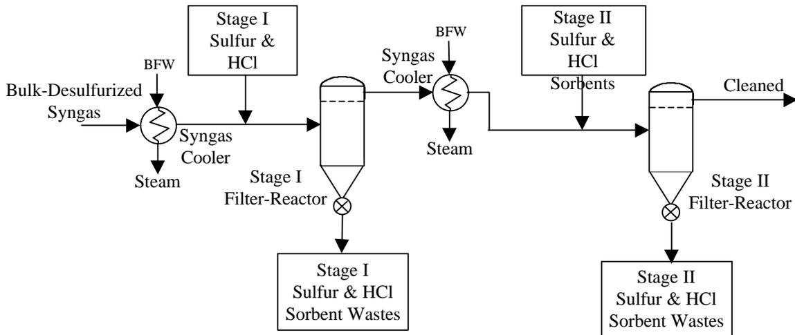
**Figure 4.8 – Base Ultra-Clean Section for Syngas Polishing**
