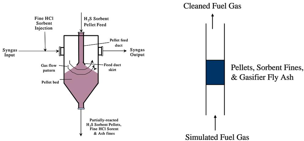
**Figure 3.13 – Laboratory Simulation of Moving Bed Filter-Reactor**
