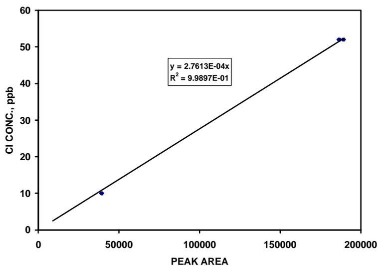
**Figure A5 – IC Calibration Curve for Chloride Determination in Liquid Solutions**
