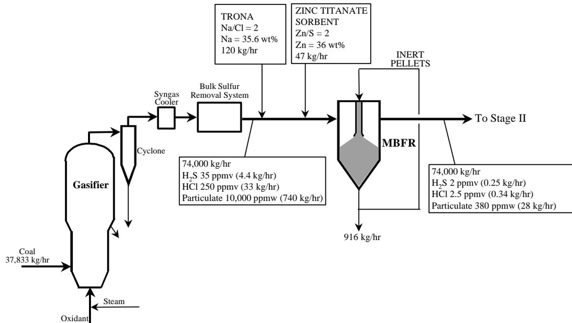
**Figure 3.63 – Material Balance for the Stage I Moving Bed Filter-Reactor (500°C)**
