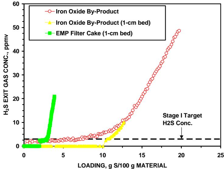
**Figure 3.26 – Performance Comparison of Stage I Desulfurization Minerals**
