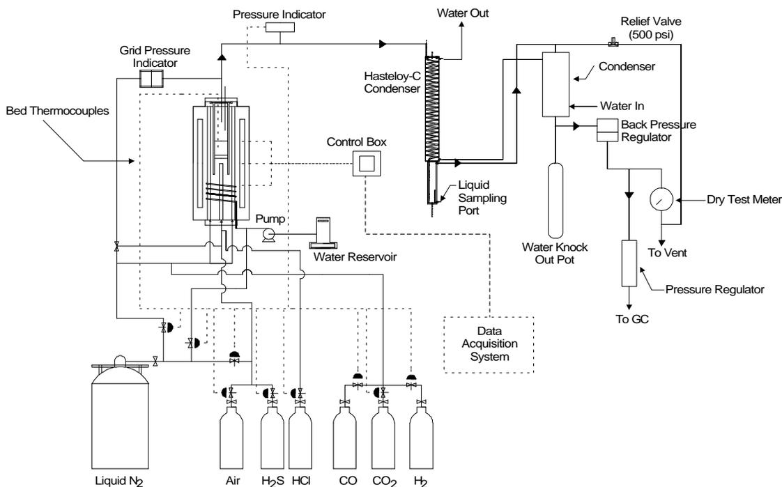
**Figure 3.18 – Overall Arrangement of the High-Pressure High-Temperature Packed-/Fluidized-Bed Reactor System**
