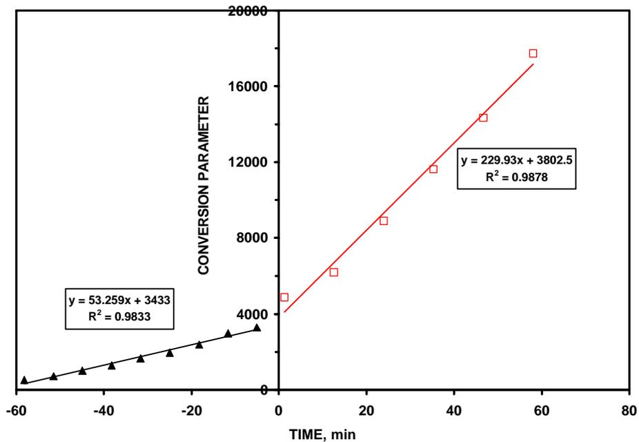
Figure 3.46 – HCl Pre-breakthrough Concentration with Katalco 59-3 at 350°C
