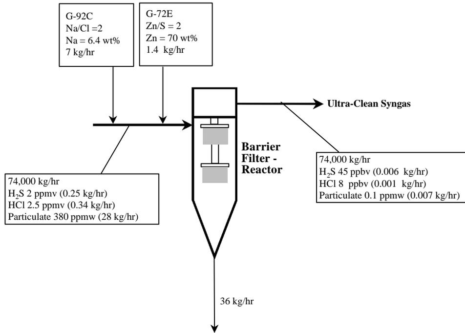
**Figure 3.66 – Material Balance for Stage II Barrier Filter Reactor with 50% Sorbent Conversion – Chemical Synthesis Application (300°C)**
