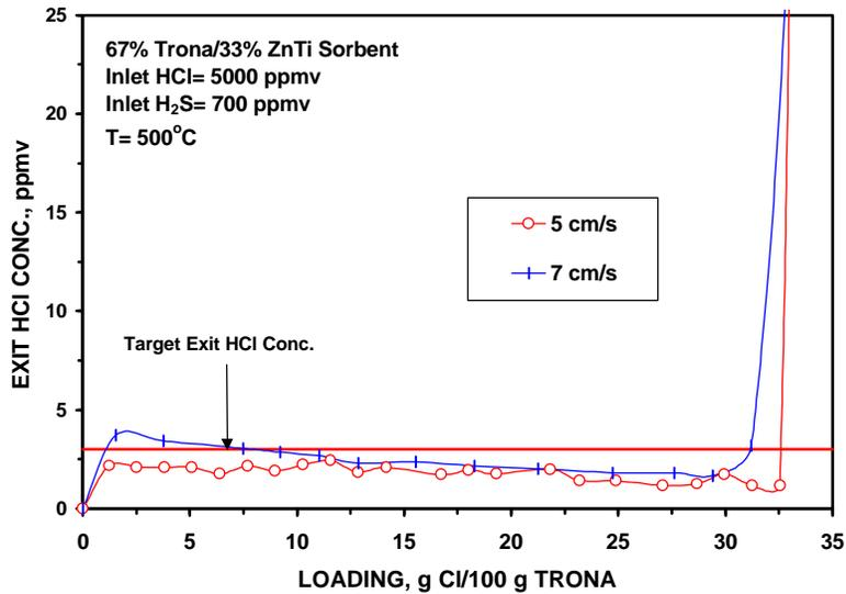
**Figure 3.37 – HCl Breakthrough Curves at Two Gas Velocities**
