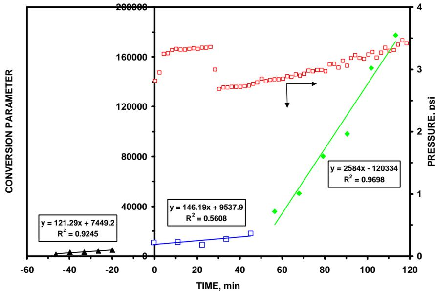
**Figure 3.48 – Reactor Pressure and Pressure Drop Across Sorbent Bed During Dechlorination Test with Trona**
