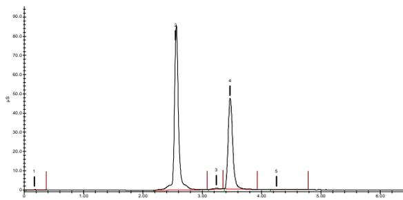
**Figure B2 – 1 ppm HCl and SO<sub>4</sub><sup>2-</sup> Liquid Calibration Standard**
