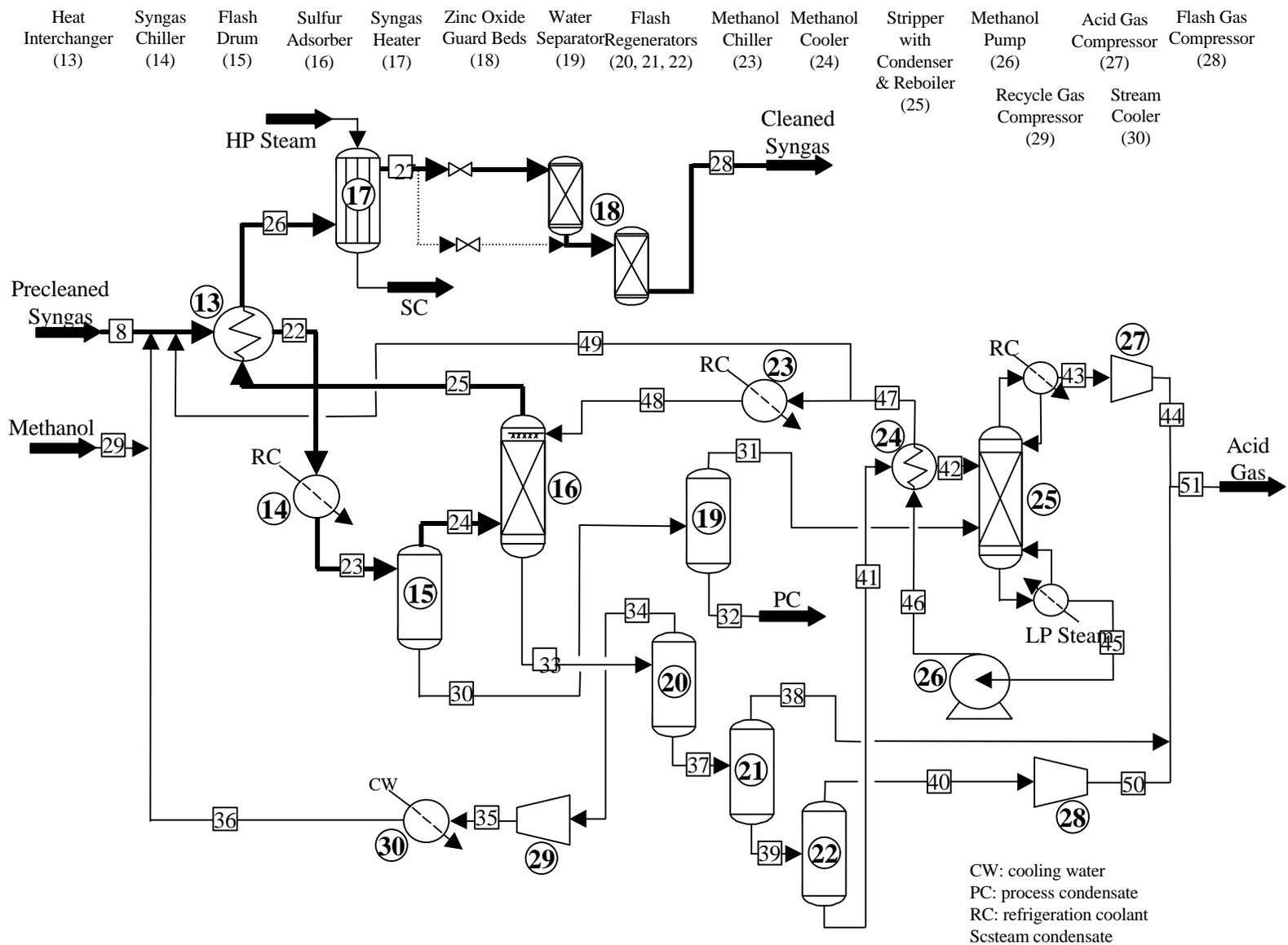
**Figure 4.4 - Conventional Syngas Cleaning - Desulfurization Section**
