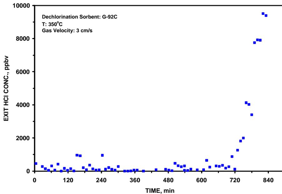
**Figure 3.50 – HCl Breakthrough Curve with G-92C Sorbent at 350°C and 3 cm/s**
