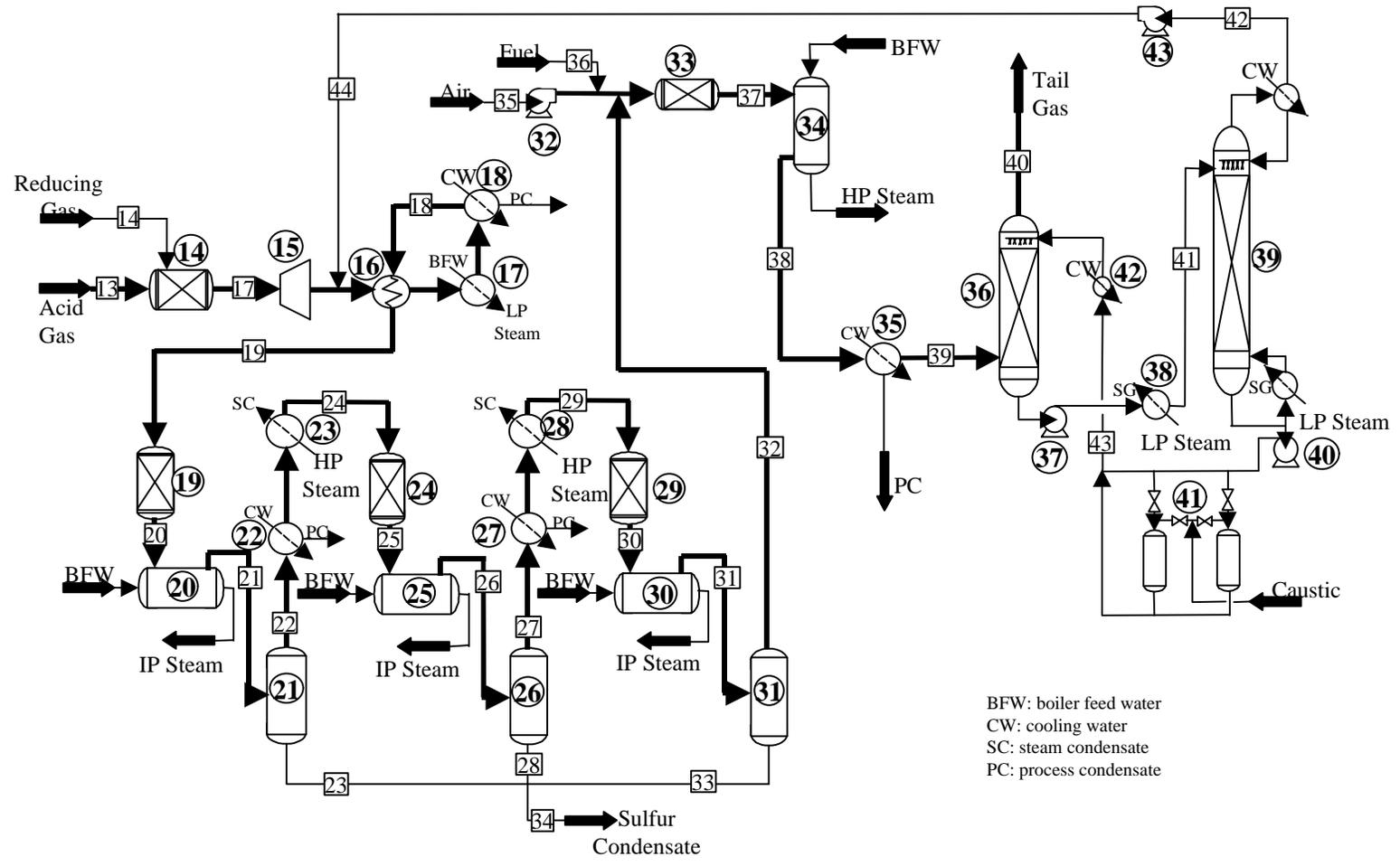
Figure 4.12 - Novel Syngas Cleaning - Sulfur Recovery Section
