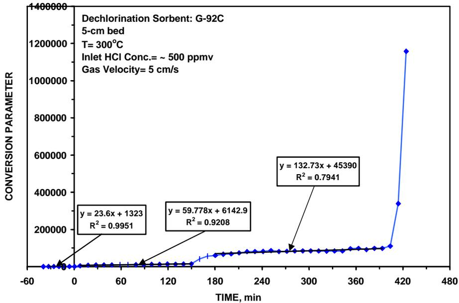
Figure 3.55 – HCl Removal Efficiency
