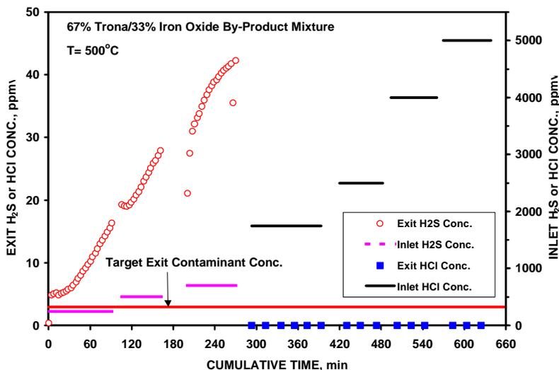
**Figure 3.31 – Scoping Test Involving H<sub>2</sub>S and HCl**
