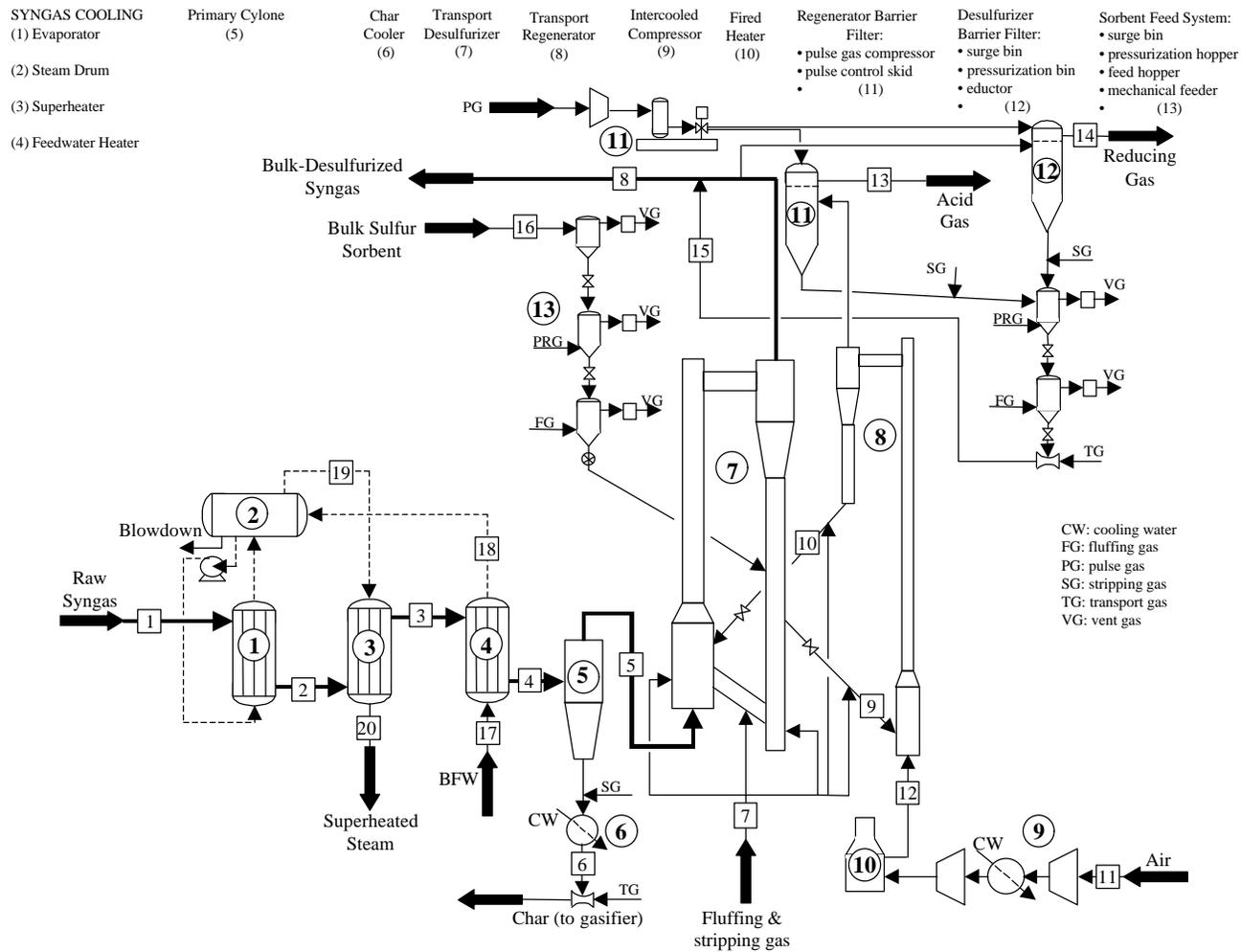
**Figure 4.19 - Novel LP-SOFC Bulk Desulfurization Section**
