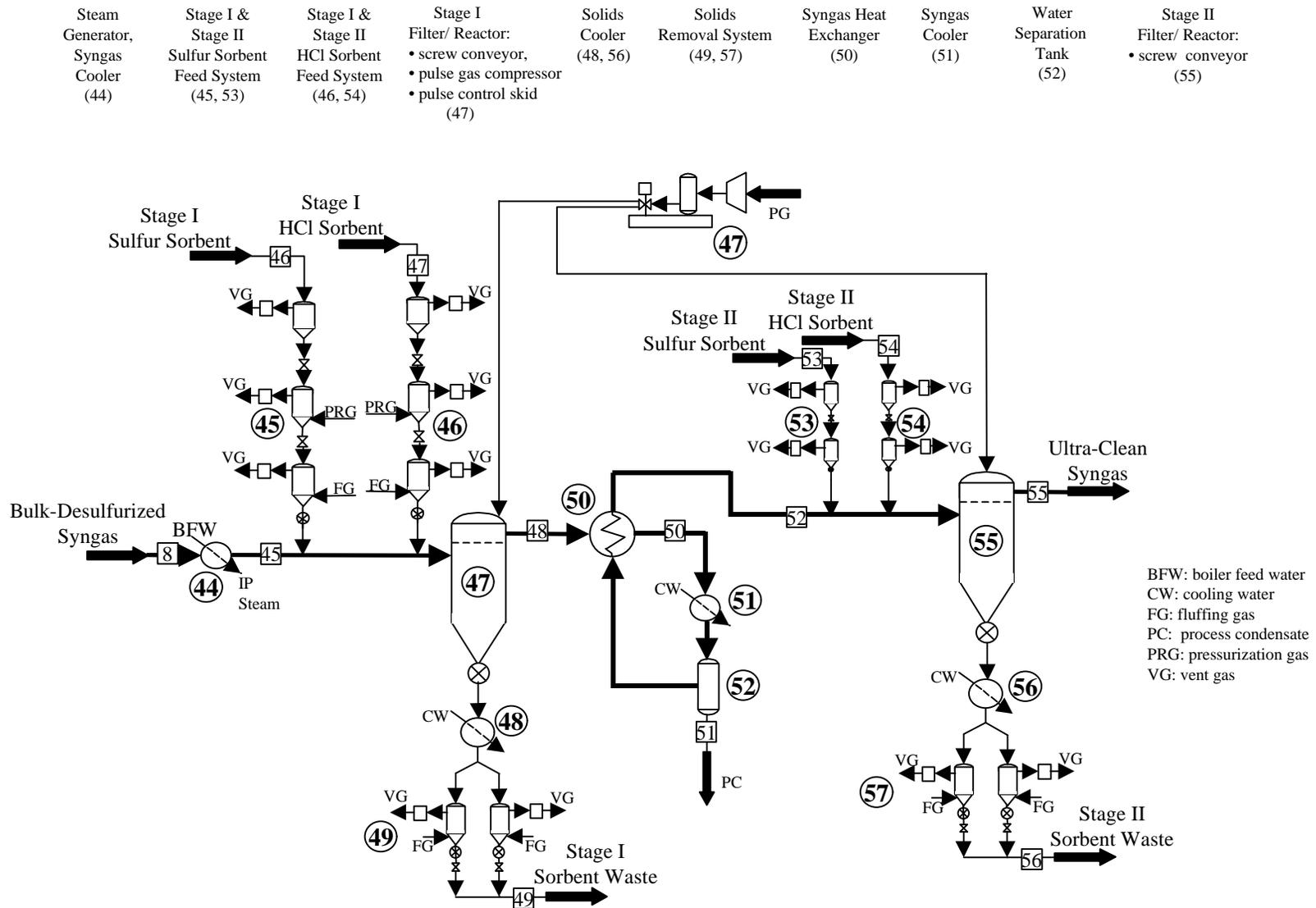
Figure 4.17 - Novel Syngas Cleaning - Ultra-Clean Section with Drying
