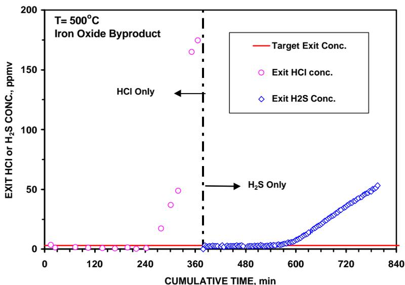
**Figure 3.32 – Scoping Test A HCl and  $\text{H}_2\text{S}$  Breakthrough Curves**
