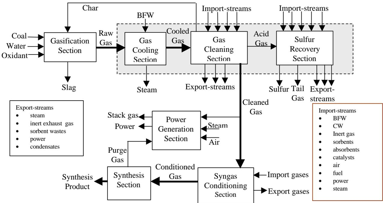
**Figure 4.1 – Vision 21 Co-production Plant and Gas Cleaning Process Boundaries**
