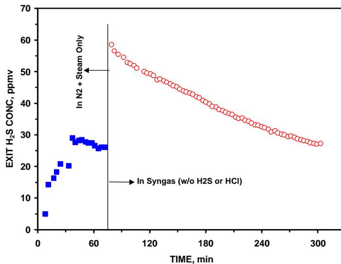
**Figure 3.11 – H<sub>2</sub>S Evolution from GPGA Ash Sample upon Exposure to Syngas**
