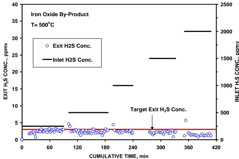
**Figure 3.27 – Scoping Test With Iron Oxide By-Product Material**
