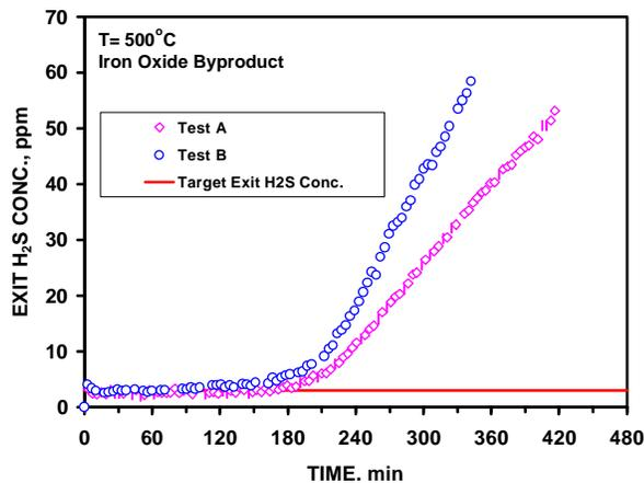
Figure 3.34 – H<sub>2</sub>S Breakthrough Curves from Tests A and B
