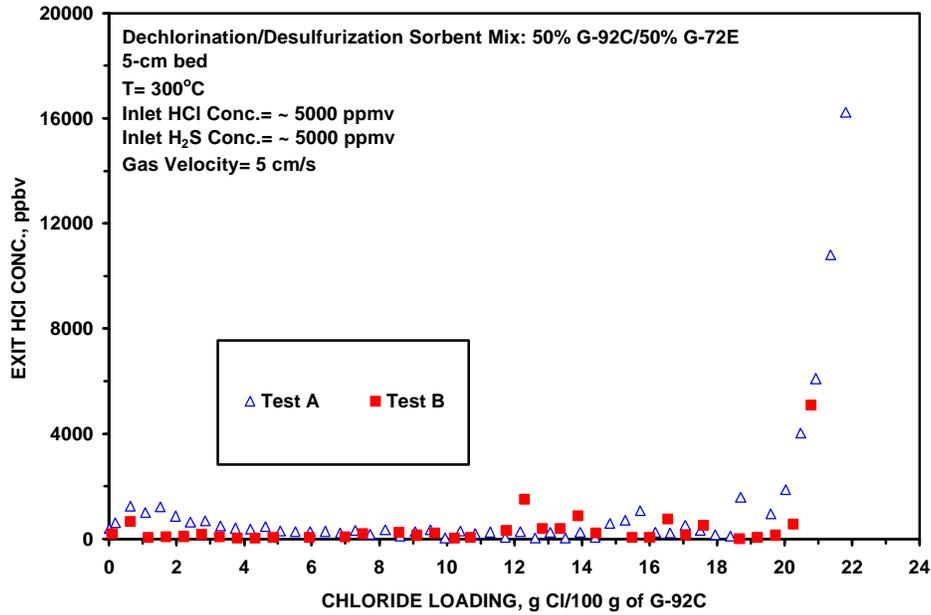
**Figure 3.61 – Stage II Chloride Removal Reproducibility**
