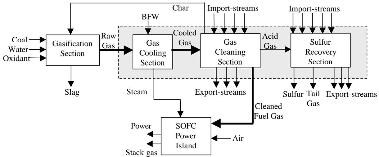
**Low-Pressure SOFC Gas Cleaning**
