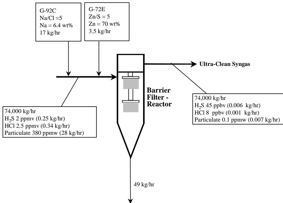
**Figure 3.65 – Material Balance for Stage II Barrier Filter Reactor with 20% Sorbent Conversion – Chemical Synthesis Application (300°C)**
