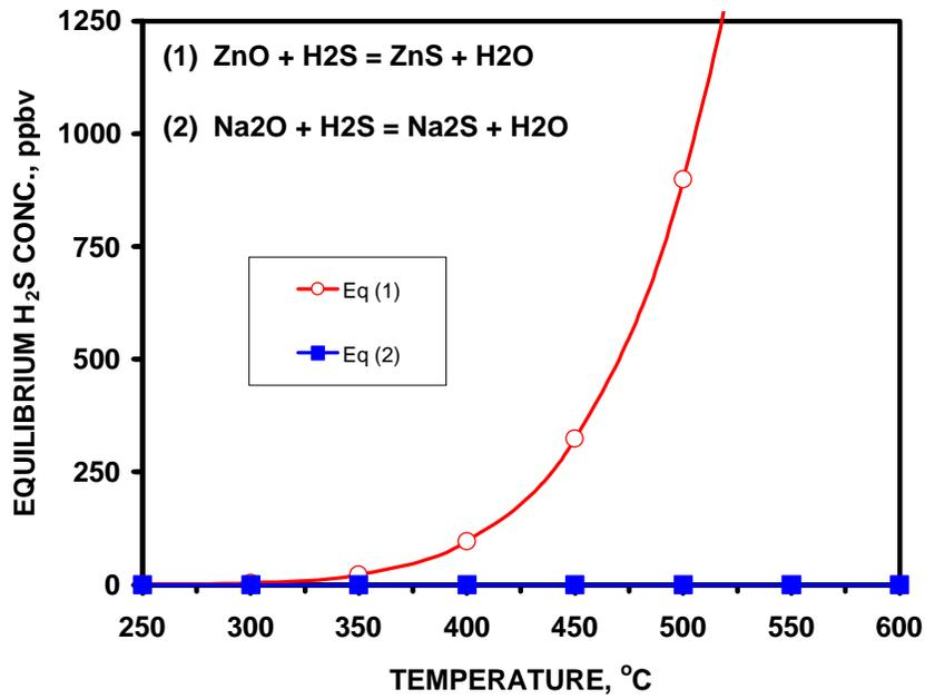
Figure 3.9 – Equilibrium H<sub>2</sub>S Concentration for ZnO and Na<sub>2</sub>O
