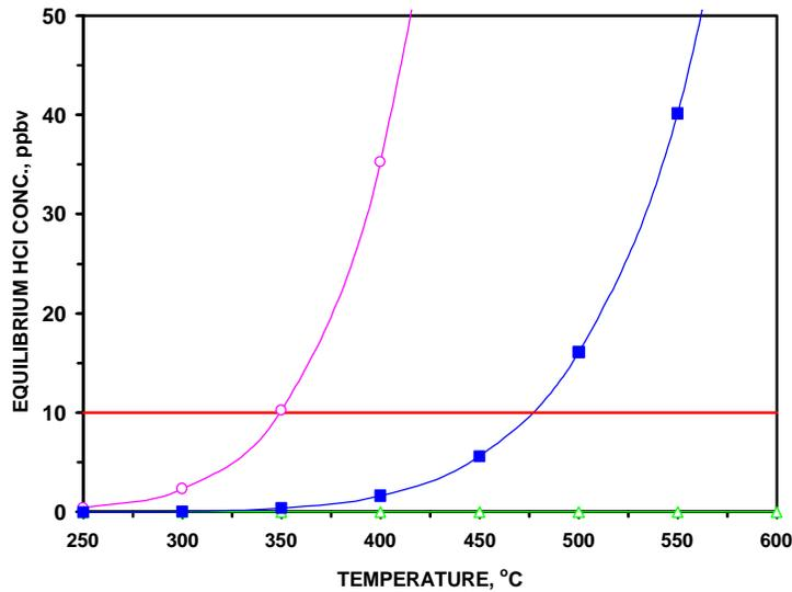
**Figure 3.5 – HCl Concentration in Simulated Syngas Following Equilibration with  $\text{Na}_2\text{CO}_3$ ,  $\text{Na}_2\text{O}$ , and  $\text{K}_2\text{CO}_3$**
