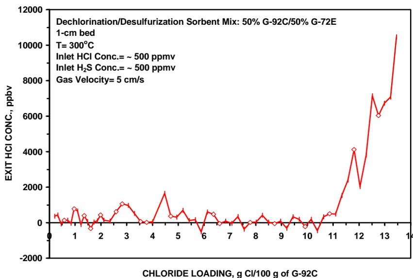
**Figure 3.57 – HCl Breakthrough Curve in Simultaneous HCl/H<sub>2</sub>S Removal Test**
