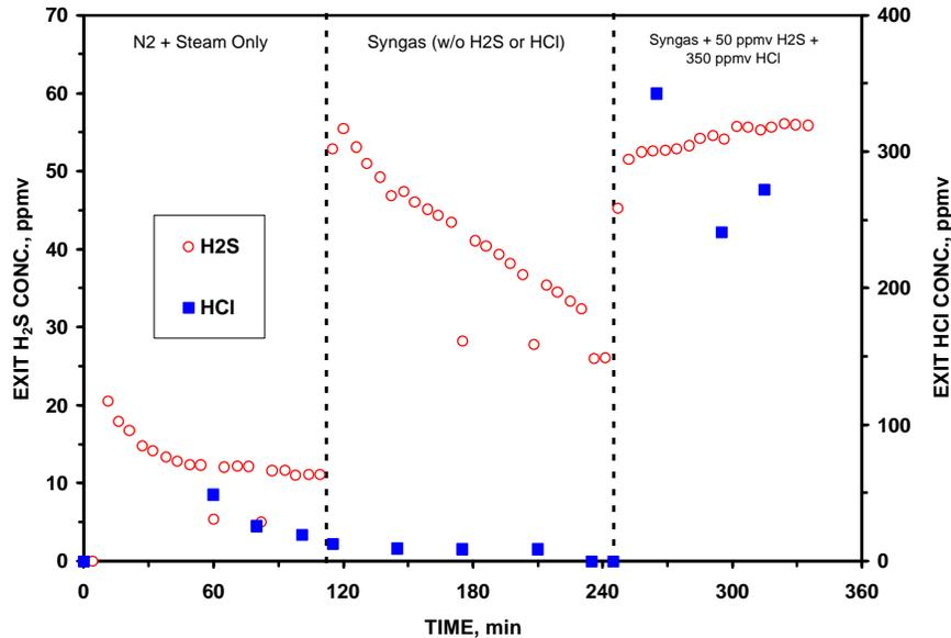
Figure 3.12 – H<sub>2</sub>S and HCl Evolution from TECo Slag Sample upon Exposure to Syngas
