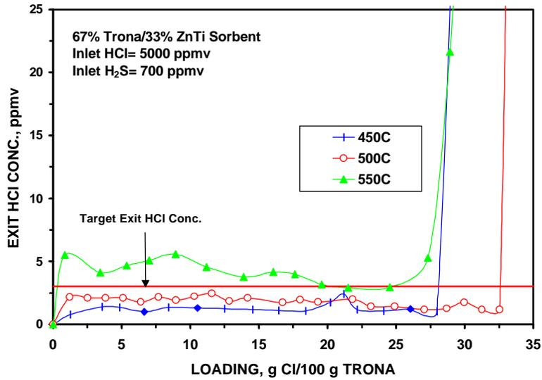
**Figure 3.39 – Effect of Temperature on Efficiency and Effective Capacity of Trona for Chloride Absorption**
