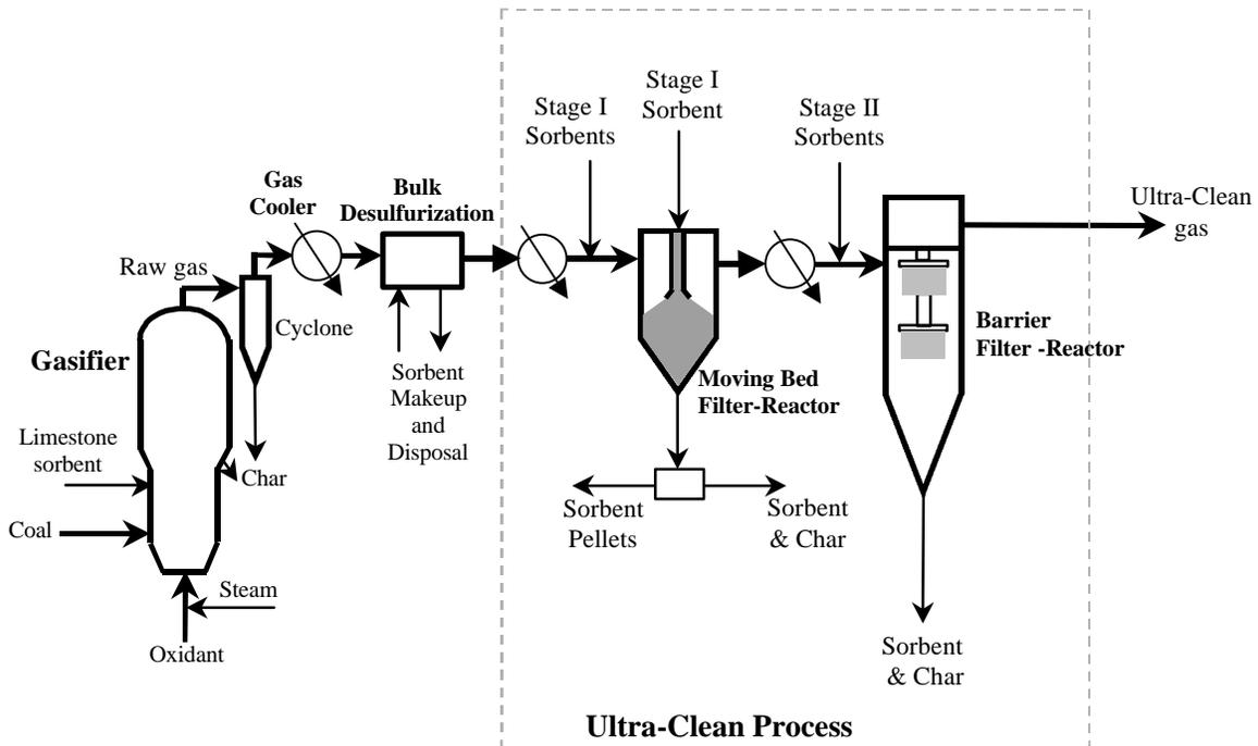
**Figure 1.1 - Ultra-Clean Gas Polishing Concept**
