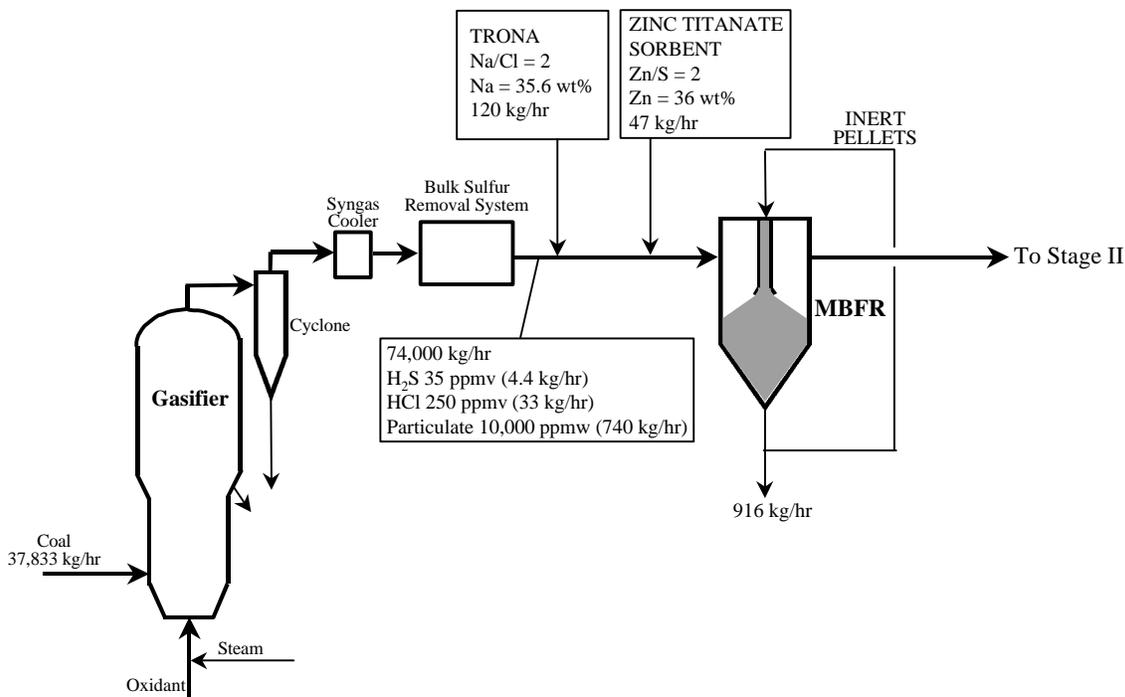
**Figure 3.35 – Material Balance for the Moving Bed Filter-Reactor with Zinc Titanate Sulfur Sorbent**
