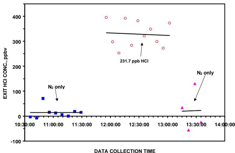
**Figure A10 – Measurement of HCl at Trace Levels**
