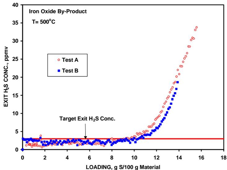
**Figure 3.28 – Reproducibility of Results from Testing of the Iron Oxide By-Product**
