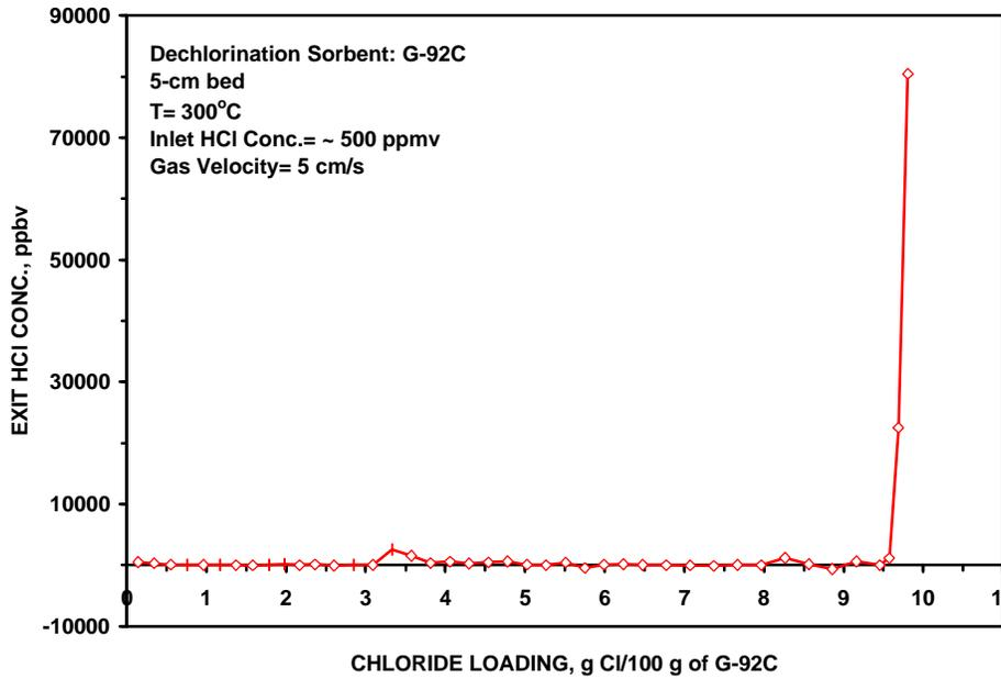
**Figure 3.54 – HCl Breakthrough Curve**
