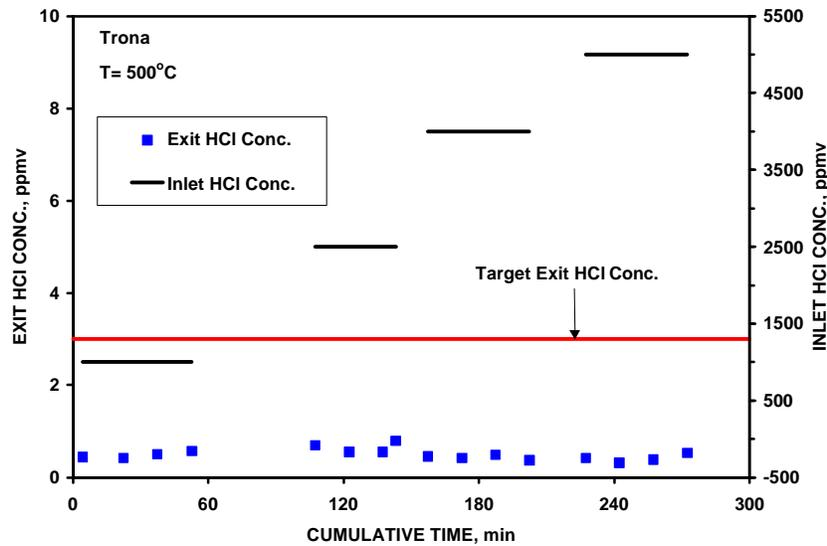
**Figure 3.22 – Scoping Test with Trona**
