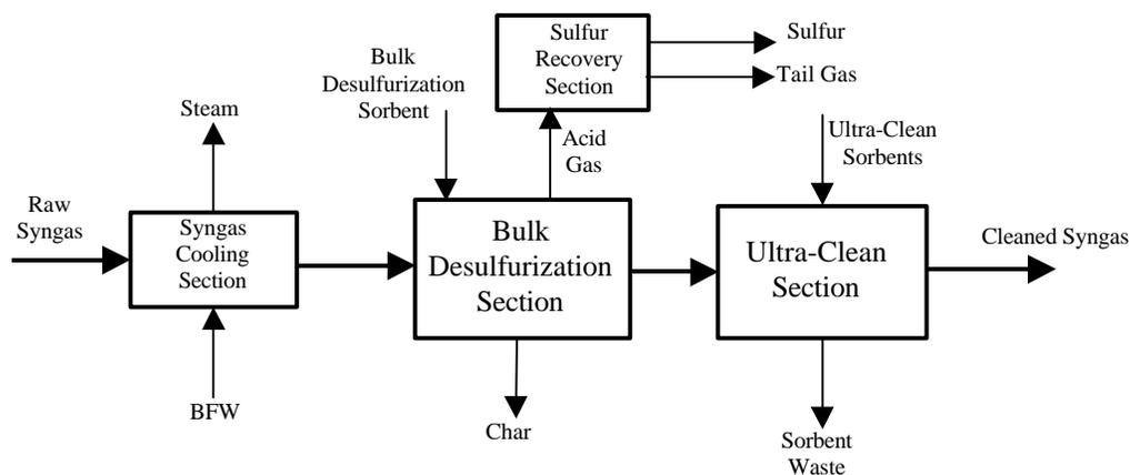
**Figure 4.7 – Novel Syngas Cleaning Process Overall Configuration**
