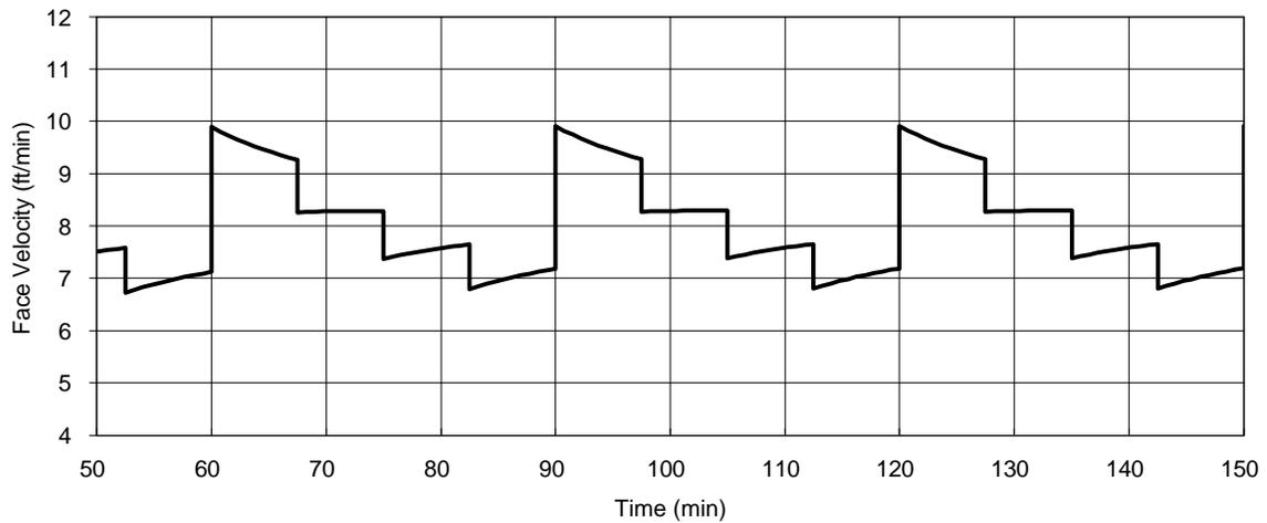
**Figure 4.15 - Stage I Barrier Filter-Reactor Plenum Face Velocity**
