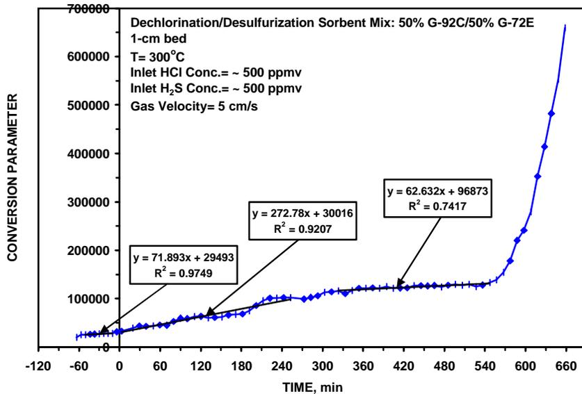
**Figure 3.59 – HCl Removal Efficiency in Simultaneous HCl/H<sub>2</sub>S Removal Test**
