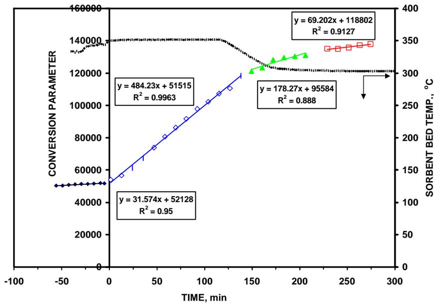
Figure 3.47 – Scoping Dechlorination Test with Pre-calcined Trona at 350°C and 300°C
