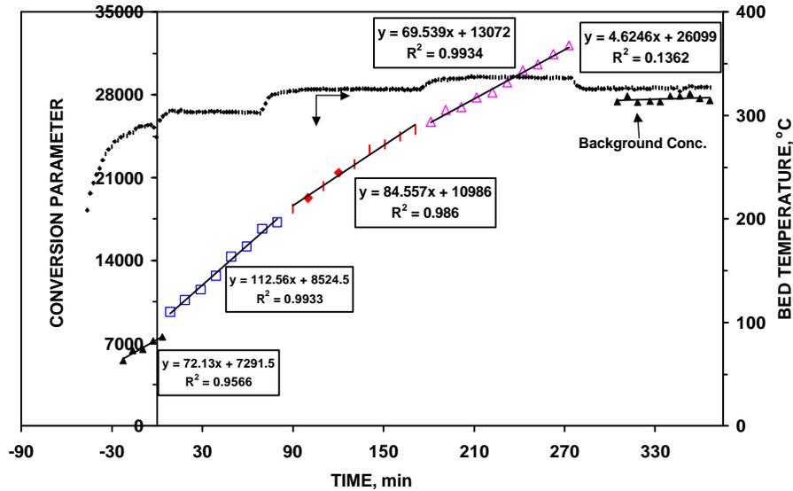
**Figure 3.53 – Scoping/Reproducibility Test with G-92C at 300-325°C**
