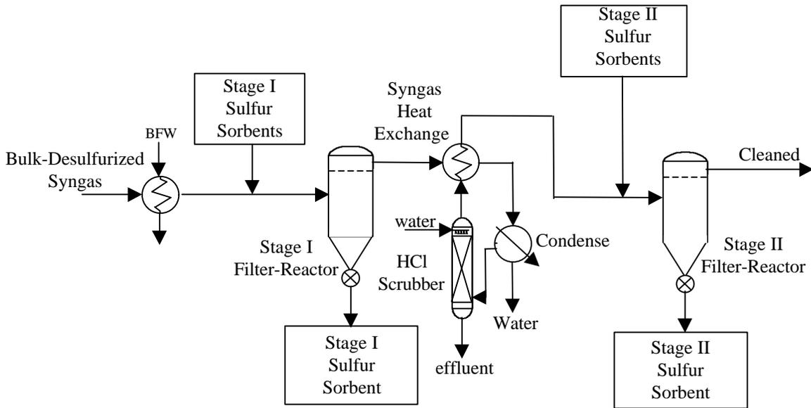
**Figure 4.10 – Ultra-Clean Section with HCl Scrubbing for Syngas Polishing**
