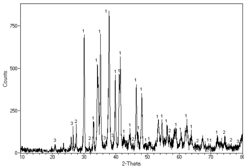
**Figure 3.24 – XRD Pattern of Highly Reduced Trona Sample**
