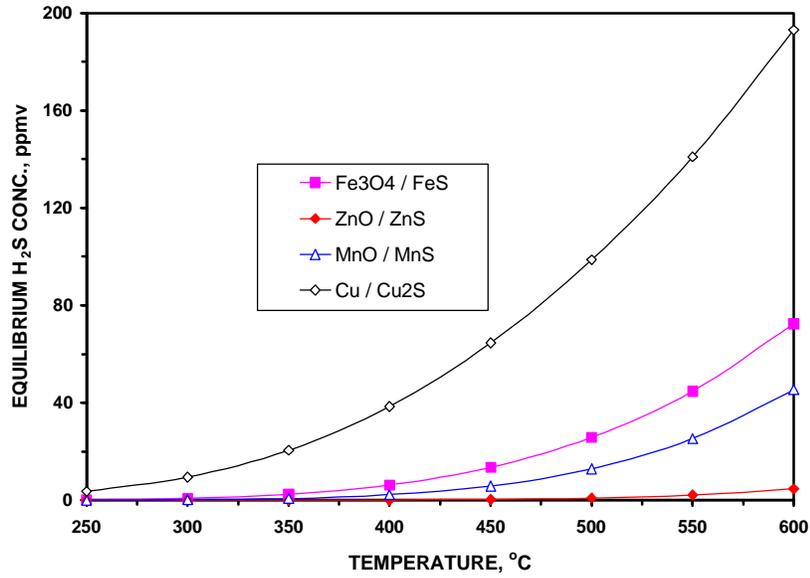
Figure 3.8 – Equilibrium H<sub>2</sub>S Concentration for Fe, Cu, Mn, and Zn Oxides
