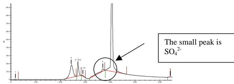
**Figure B1 – Chromatogram for 219 ppbv H<sub>2</sub>S in N<sub>2</sub>, CO, CO<sub>2</sub>, and CH<sub>4</sub>**
