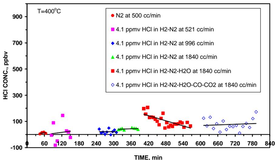
**Figure 3.42 – Scoping Test with the G-92C Dechlorination Material**
