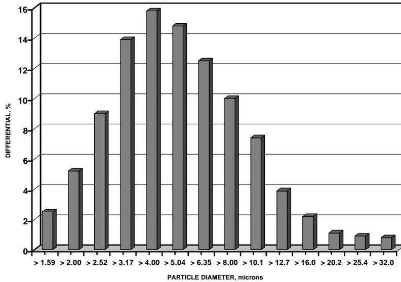
**Figure 3.10 – Size Distribution of Selected Gasifier Fly Ash (Piñon Pine)**
