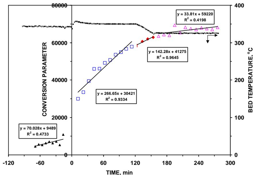
**Figure 3.52 – HCl Pre-breakthrough Concentration with G-92C at 350°C and 325°C**
