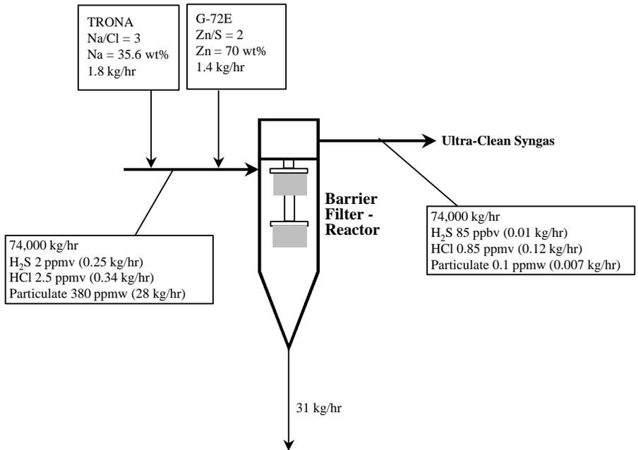
**Figure 3.64 – Material Balance for the Barrier Filter Reactor – Fuel Cell Application (350°C)**
