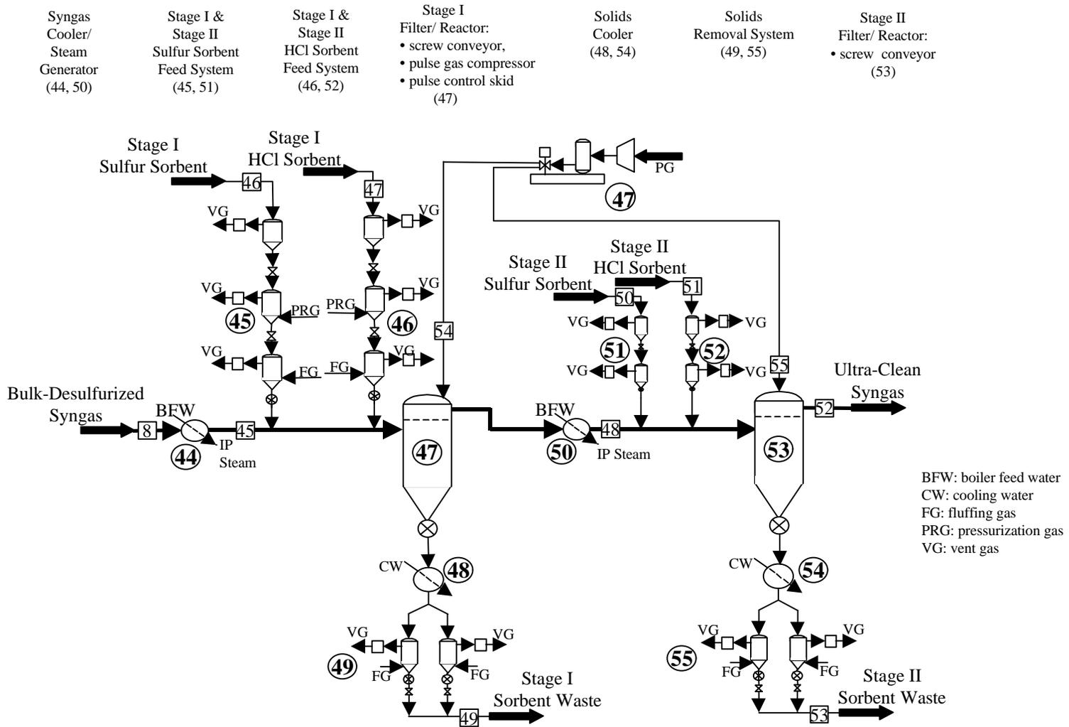
**Figure 4.13 - Novel Syngas Cleaning - Ultra-Clean Base Section**
