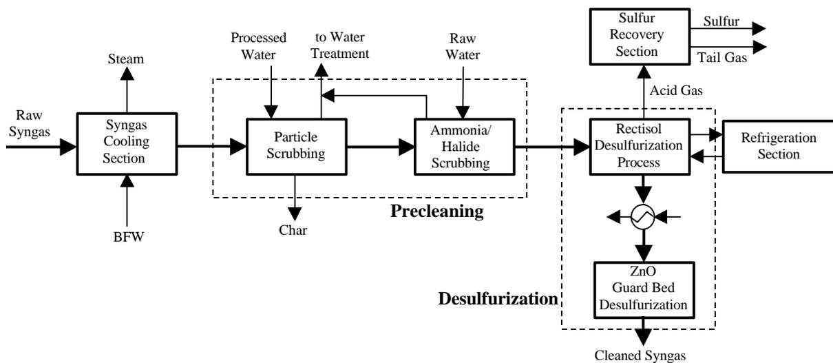
**Figure 4.2 – Conventional Syngas Cleaning Schematic**
