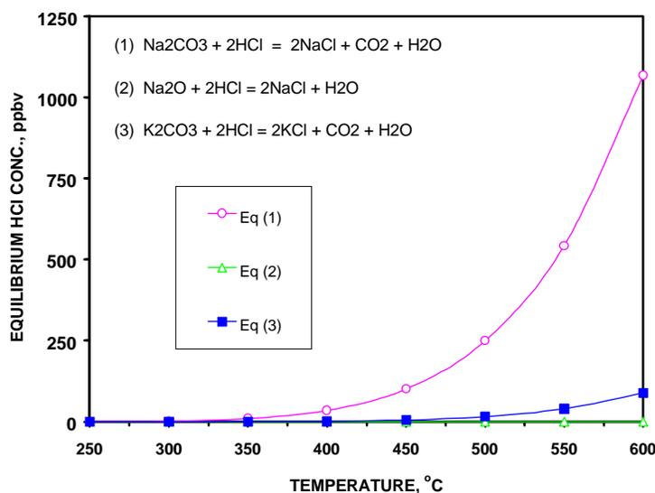
**Figure 3.4 – HCl Concentration Following Equilibration with  $\text{Na}_2\text{CO}_3$ ,  $\text{Na}_2\text{O}$ , and  $\text{K}_2\text{CO}_3$**
