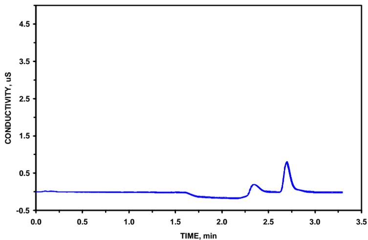
**Figure A4 – IC Chromatograms for the 10-ppb Cl Standard Solution**
