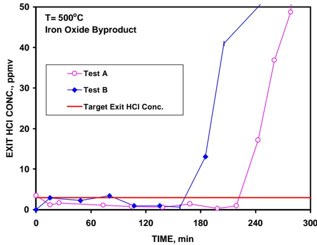
Figure 3.33 – HCl Breakthrough Curves from Tests A and B
