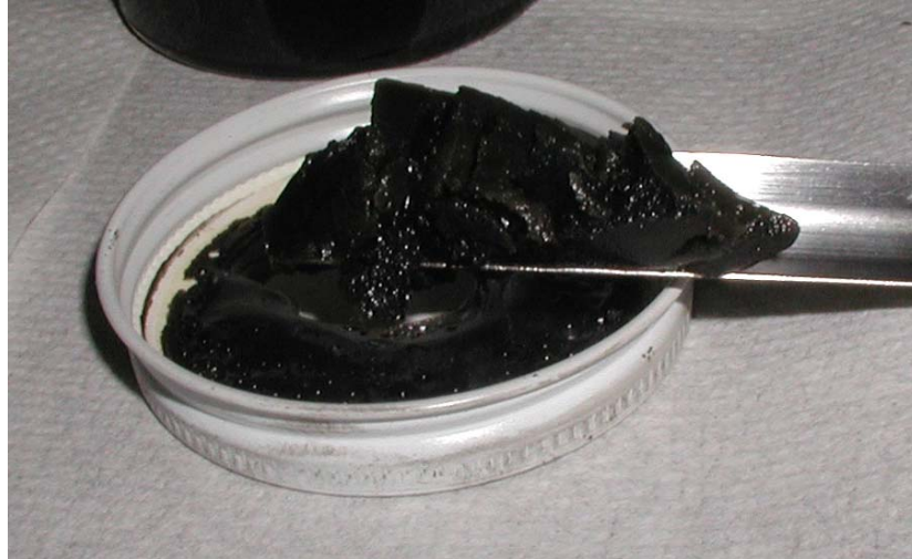
Figure VIII.C.2-1. Hydrocarbon (Durasyn)/Used Catalyst; Feed Mix – RI59.
