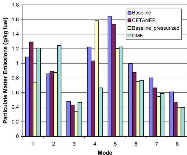
Figure 4. Particulate Matter Emissions, g/kg Fuel Basis.
