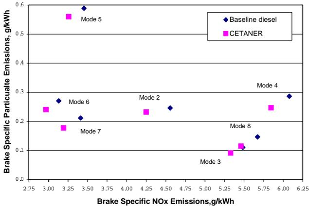
Figure 6. Brake-Specific Particulate Emission vs. NOx Emission Tradeoff.
