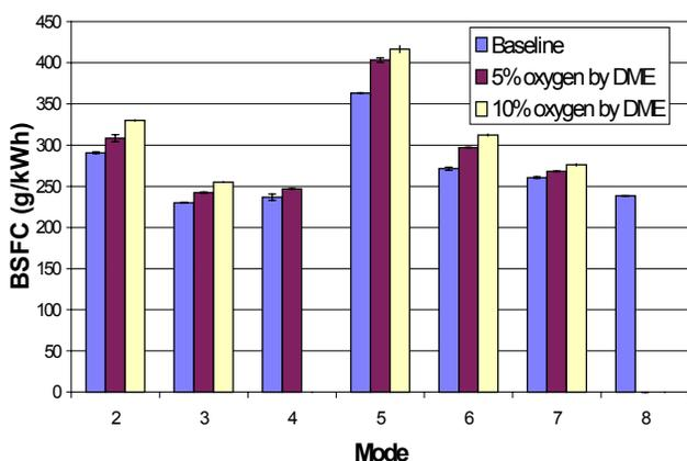
**Figure 8. Brake Specific Fuel Consumption (BSFC)**
