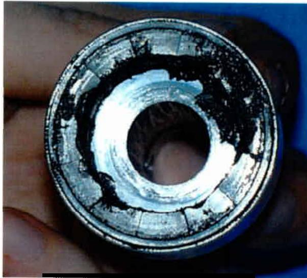
**Figure 16. Damaged magnetic coupling from Tuthill gear pump.**
