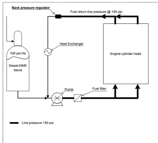
Figure 2. Diagram of the pressurized fuel system [5].
