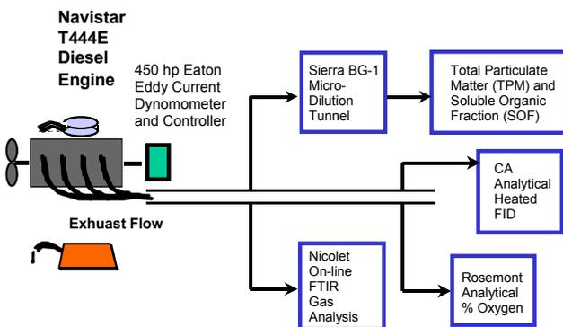
**Figure 1. Multicylinder Test Cell, Navistar T444E Turbodiesel**
