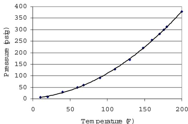
**Figure 5. Vapor pressure of DME as a function of temperature [50].**
