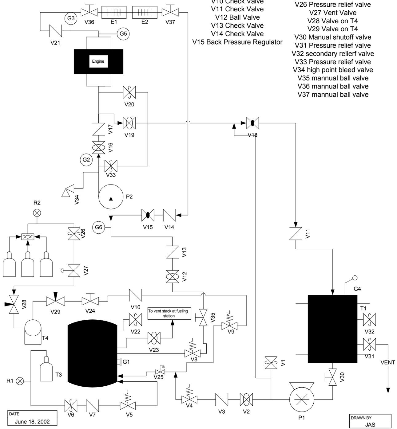
**Figure 2. Schematic Diagram of the DME-Diesel Fueling System**
