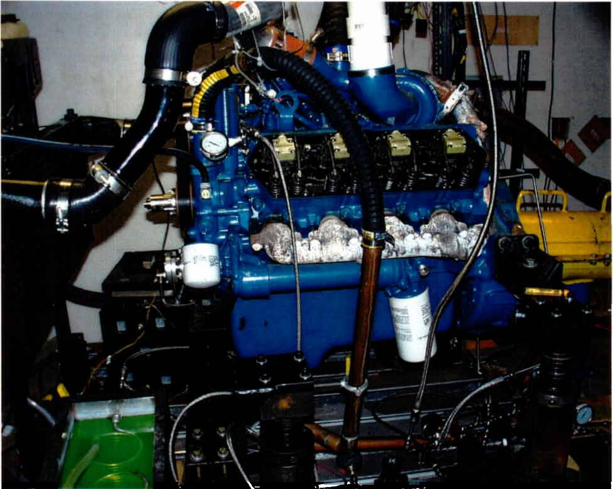
**Figure 2. Navistar T444E showing conversion to DME-diesel operation.**
