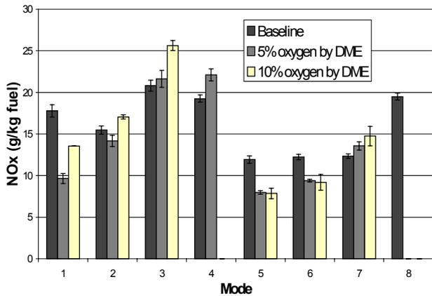
**Figure 4. NOx Emission Results per unit fuel consumed, g/kg fuel**
