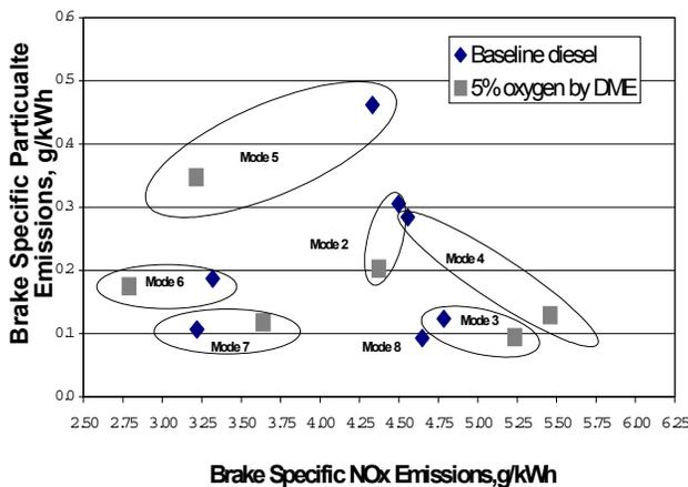
**Figure 5. Brake-Specific Particulate Emission vs. NOx Emission Tradeoff**
