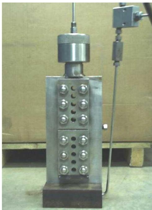
Figure 1. High pressure viscometer housing.
