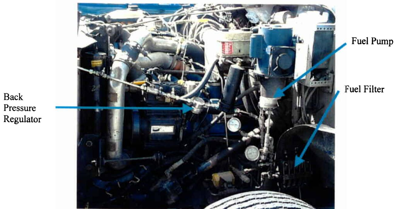
**Figure 14.** Photograph of the fuel handling system on the converted shuttle bus
