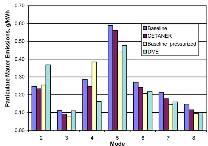
Figure 3. Particulate Matter Emissions, Brake Specific Basis.
