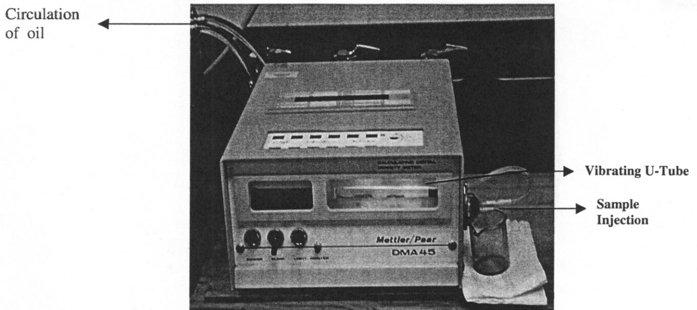
FIGURE 3.1 The Anton-Paar Digital Density Meter.
