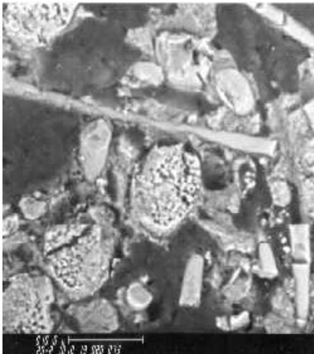
Figure 15. 20X BSE image of sample C2-2 from thermal fatigue exposure test.
