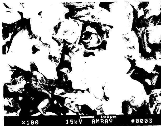
Figure 20 SEM micrographs of the failed ceramic filter showing morphological characteristics of the fractured surface.
