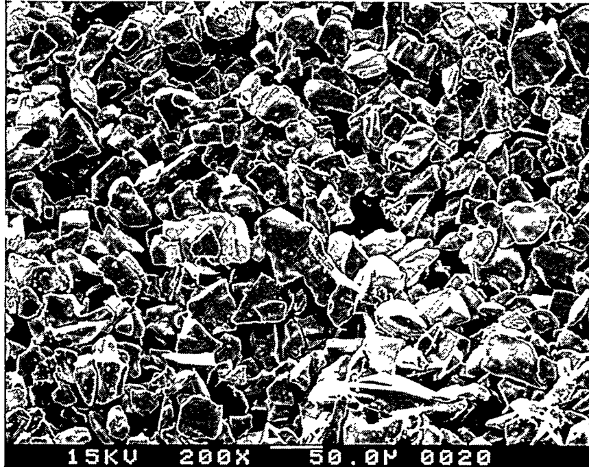
Figure 4-26. Micrograph of Refractron 70/3 with 442-T/Unused: Outer surface (200X)
