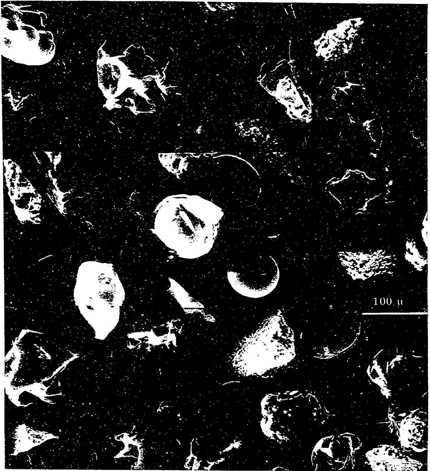
Figure IIA-8. SEM Micrograph of a 558°C Drop Tube Char of Pittsburgh No.8 Bituminous Coal. Magnification: 300X.
