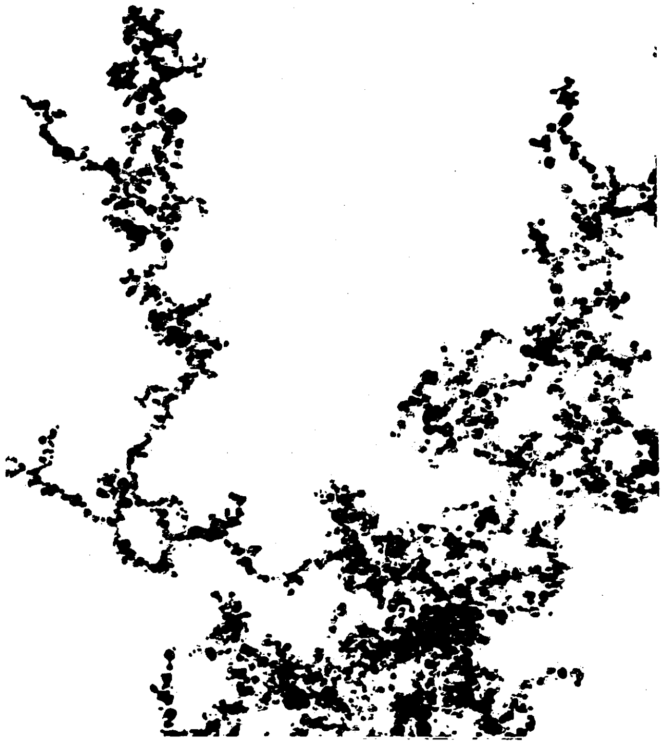
Figure 11 Electron Micrograph of Particles Collected by P-T-P Electrostatic Precipitation Magnification 200,000X
