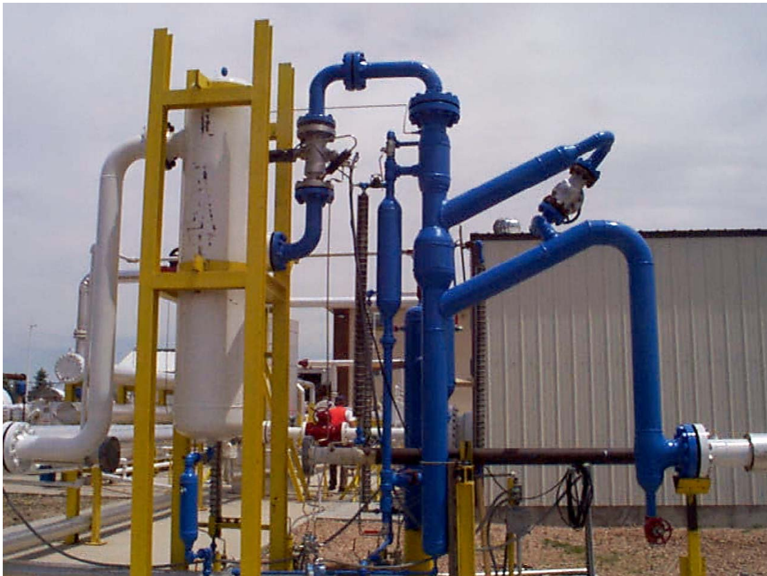
Figure 21 – High Pressure GLCC Test Facility at CEESI (Colorado Engineering Experiment Station)
