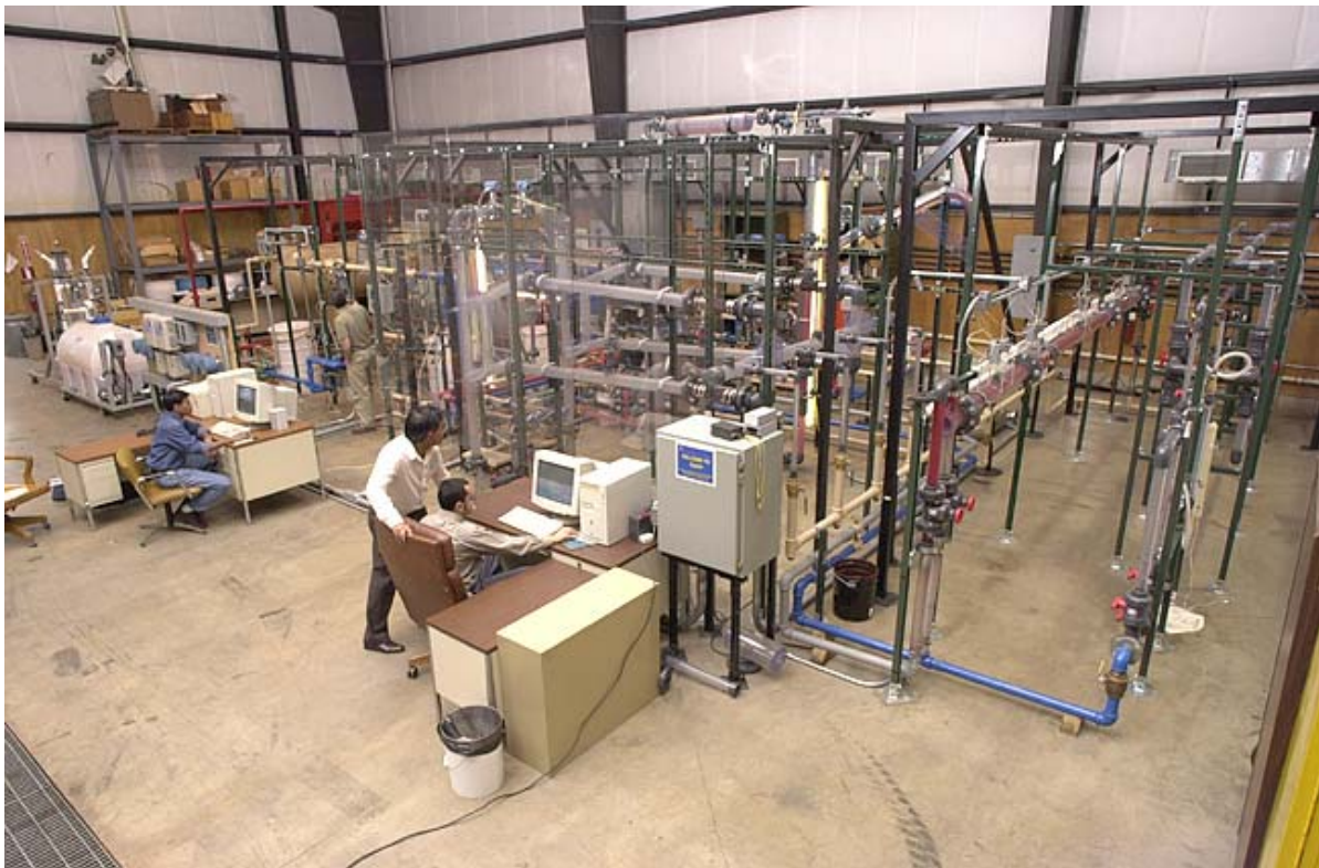
Figure 3. Three-phase Flow Loop
