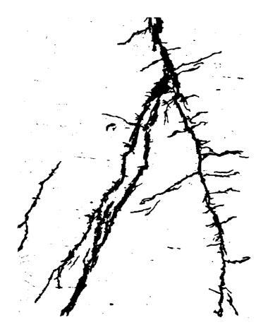
No. 3 Complex transgranular cracking near the intersection of a transverse and longitudinal crack. 200x, Oxalic acid, 2 minutes.
