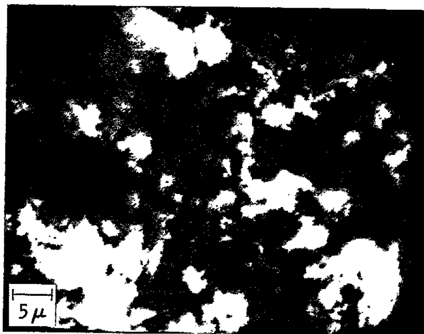
Figure 15. SEM photomicrograph of the surface of ICI 46-1 catalyst used in ATR of the n-tetradecane/thiophene mixture at P = 1 atm, T_p = 1150^\circ\text{F} , (\text{O}_2/\text{C})_m = 0.38 , (\text{S}/\text{C})_m = 0.6 , and \text{S.V.} = 10,000 \text{ hr}^{-1} .
