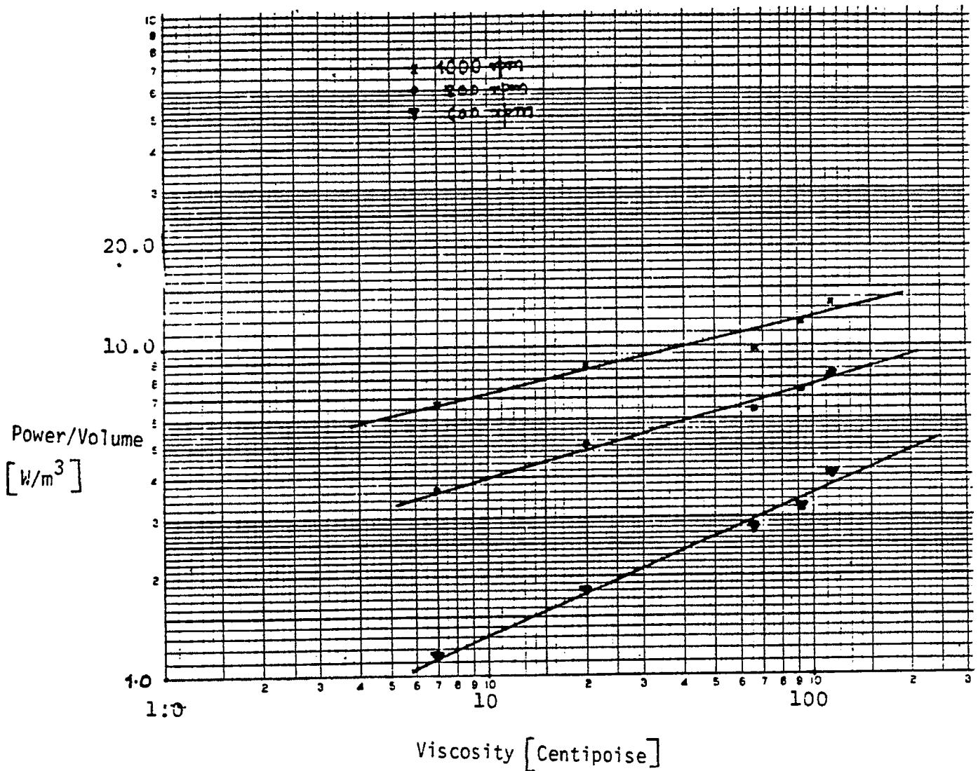
FIGURE 3.6 Variation of Power/Volume with Viscosity
