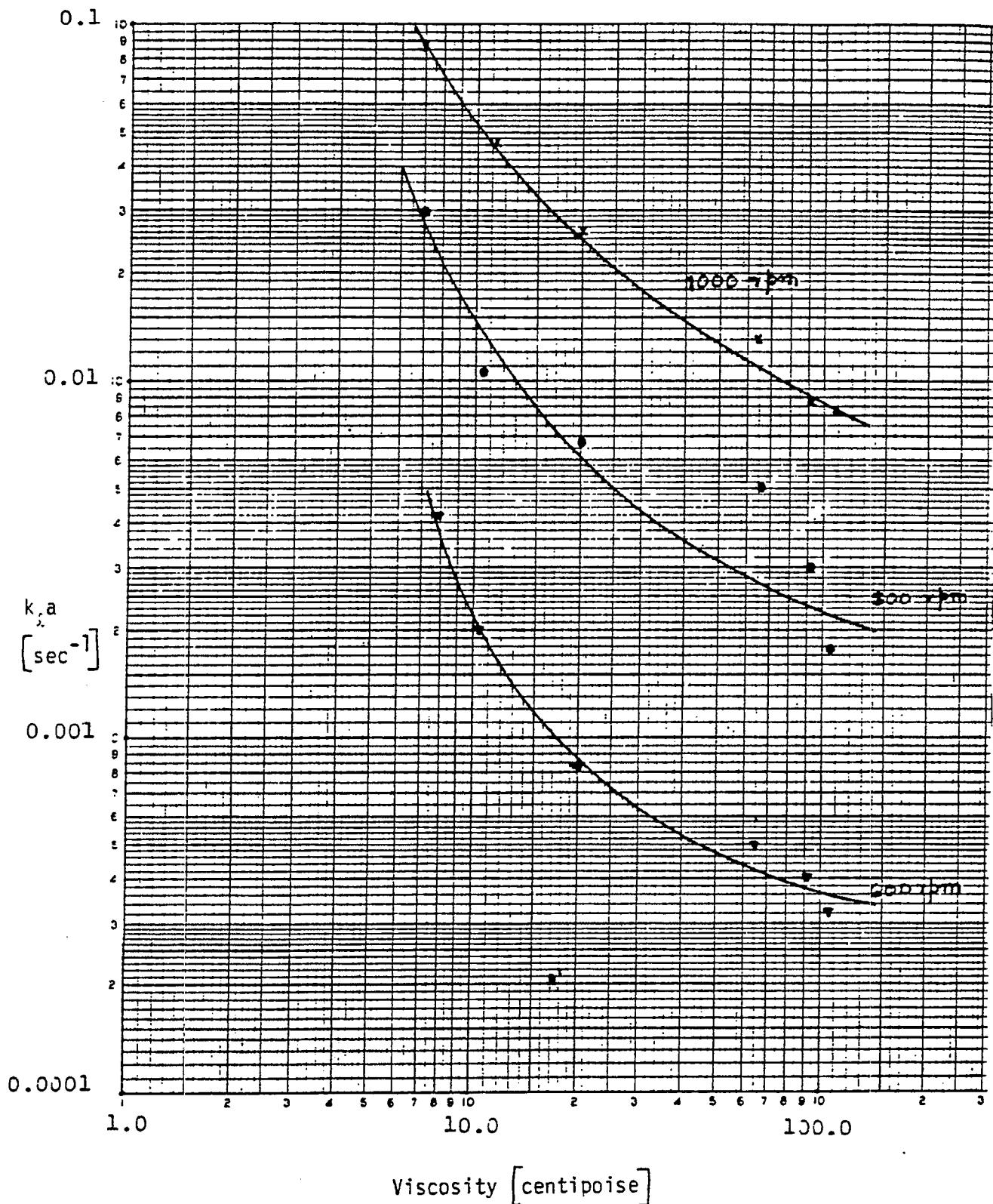
FIGURE 3.2 ' $k_l a$ ' as a Function of Liquid Phase Viscosity
