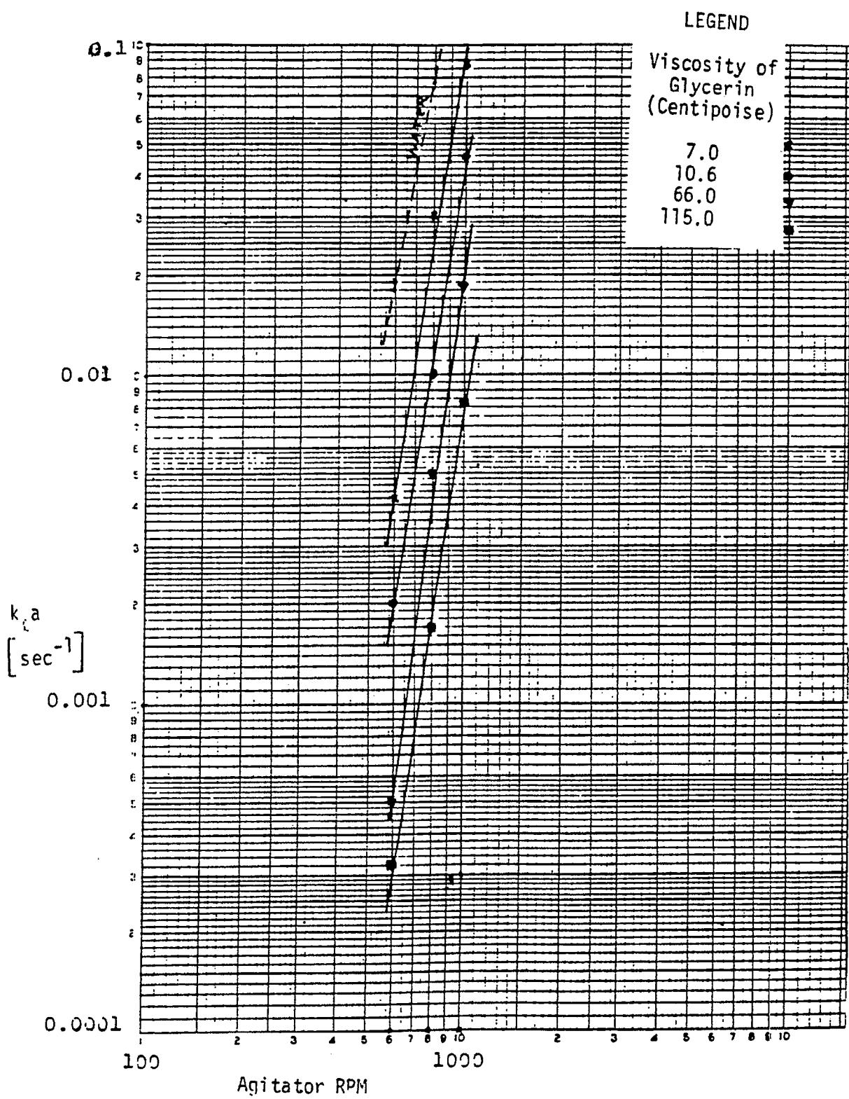
FIGURE 3.4 Variation of ' $k_f a$ ' with Agitator RPM
