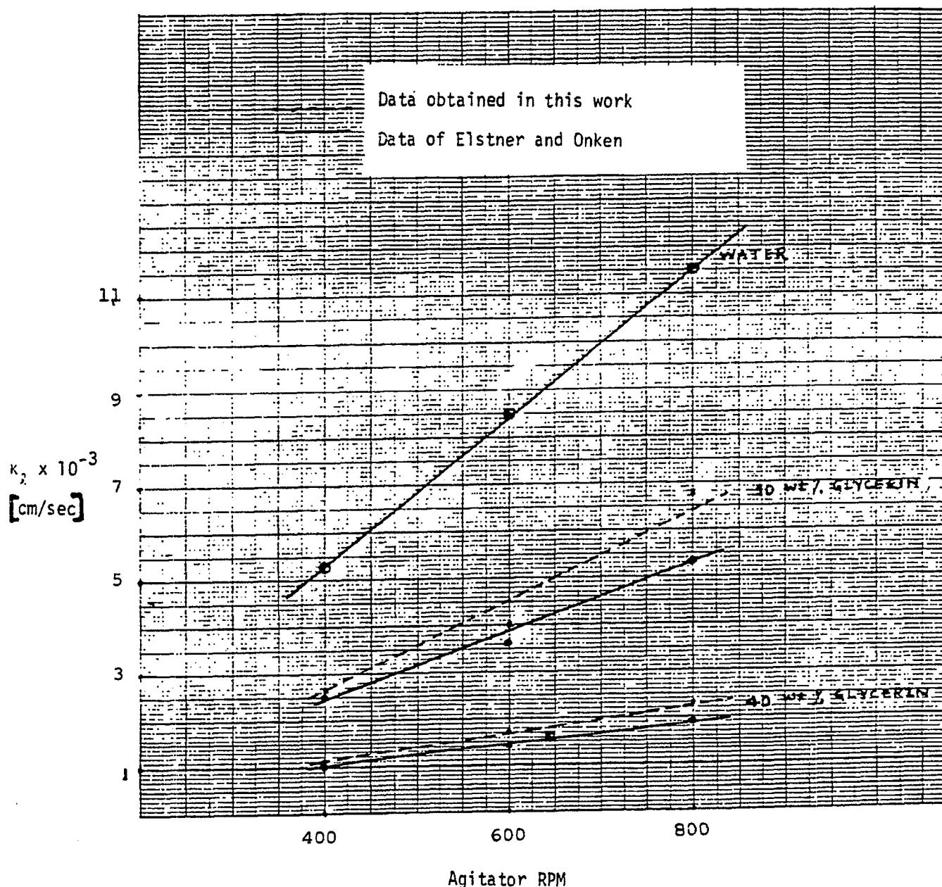
FIGURE 3.1 Values of Mass Transfer Coefficient ' $k_L$ ' for Various Values of Agitator RPM in Standard Vessel Arrangement
