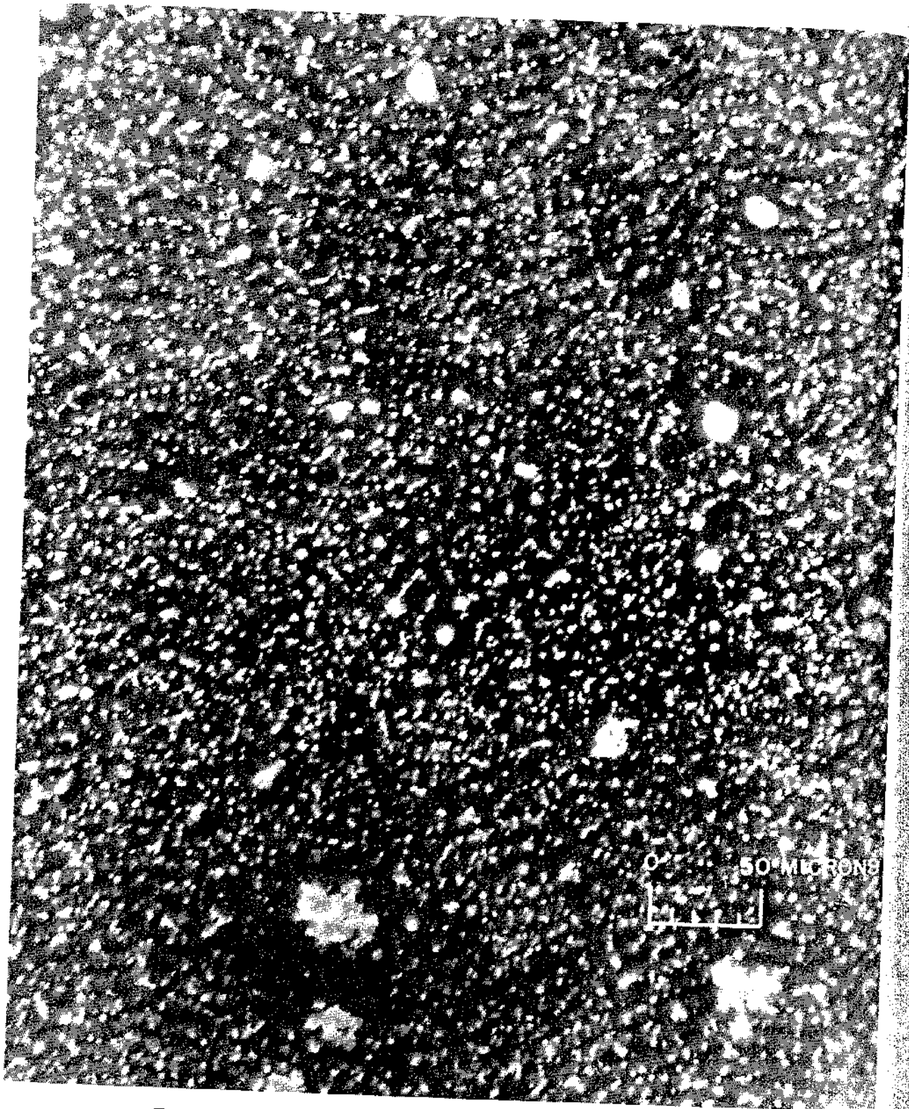
Figure 17. - Dispersion of fine particles showing agglomeration.
