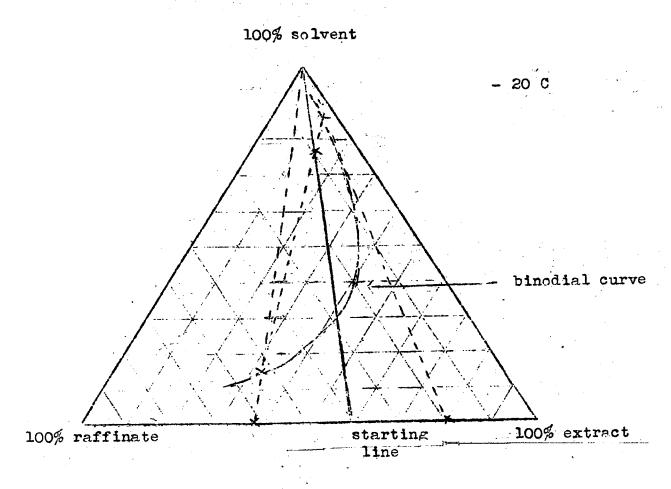
The solvent need not be a chemical individual. On the contrary it proved to be advantageous to use a combination of two solvents which could be adapted to any oil with regard to solubility of wax and optimum triangular considerations. Besides the chemical character of an oil and its molecular weight, it is the percentage of dilution which is of deciding influence upon phase separation. The desirable condition for feeding stock to the filters is expressed in the following graph:
