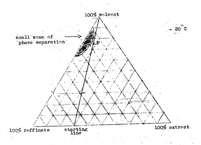
There should exist a small zone of phase separation for the more saturated components of the oil. That does not mean that the oil will give phases when diluted, but its more valuable constituents shall not be readily miscible with the solvent under all circumstances.
