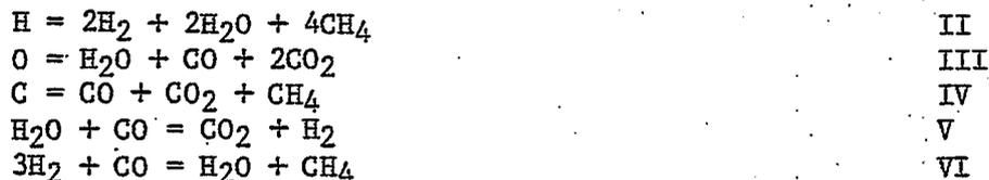
The two chemical equations are the water-gas shift (V) and methanation (VI) reactions.
